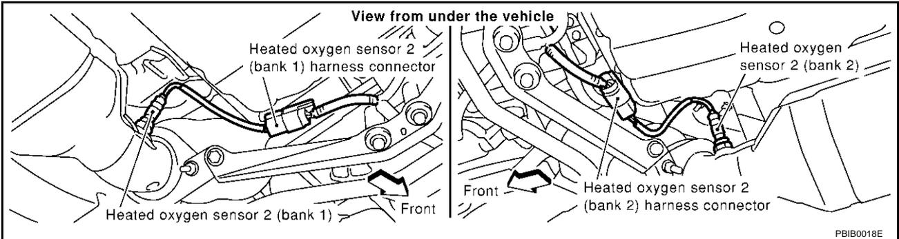
3. Check harness continuity between HO2S2 terminal 4 and engine ground.
