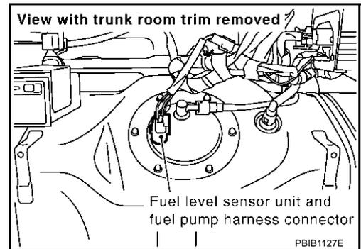
4. Check voltage between fuel level sensor unit and fuel pump terminal 5 and ground with CONSULT-II or tester.
