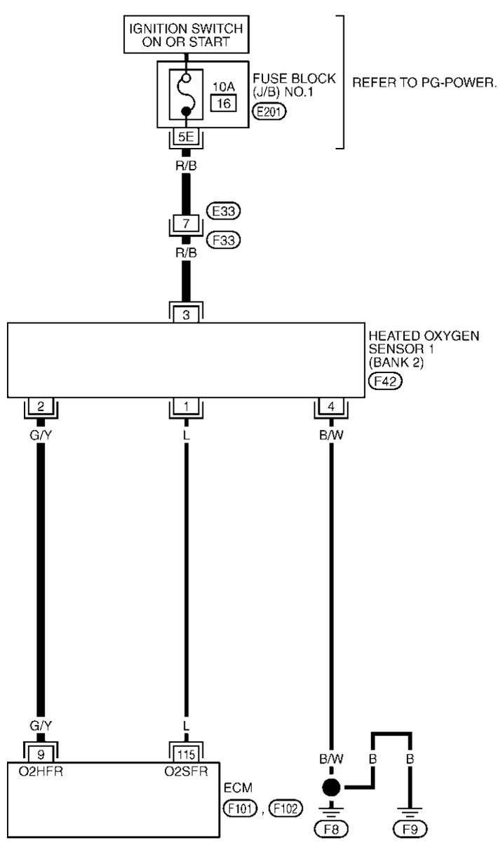
— : DETECTABLE LINE FOR DTC
