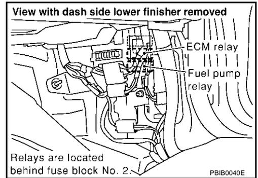
2. Check voltage between ECM relay terminal 7 and ground with CONSULT-II or tester.
