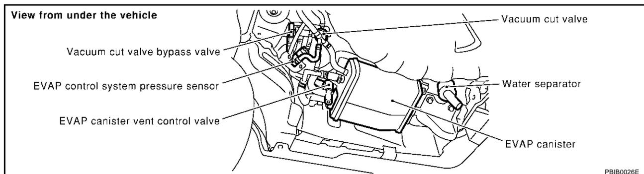
2. Check sensor harness connector for water.
