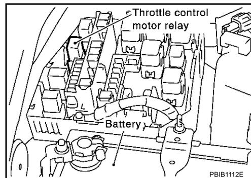
4. Check voltage between throttle control motor relay terminals 2, 5 and ground with CONSULT-II or tester.
