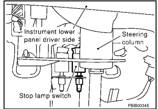
2. Check continuity between stop lamp switch terminals 1 and 2 under the following conditions.
