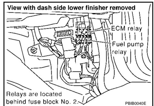
2. Check voltage between ECM relay terminals 2, 5 and ground with CONSULT-II or tester.
