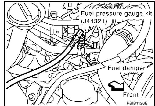
3. Connect the fuel pressure test gauge (quick connector adapter hose) to the inline fuel quick disconnected fitting.
