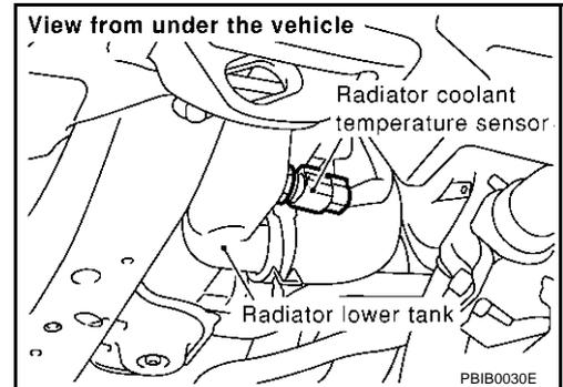
4. Check voltage between radiator coolant temperature sensor terminal 1 and ground with CONSULT-II or tester.
