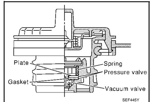
2. Check valve opening pressure and vacuum.
