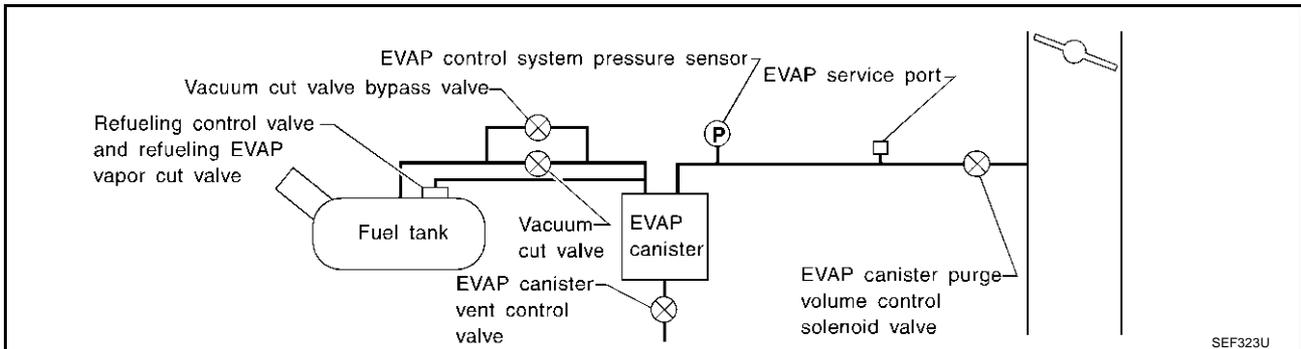
In this evaporative emission (EVAP) control system, purge flow occurs during non-closed throttle conditions. Purge volume is related to air intake volume. Under normal purge conditions (non-closed throttle), the EVAP canister purge volume control solenoid valve is open to admit purge flow. Purge flow exposes the EVAP control system pressure sensor to intake manifold vacuum.
