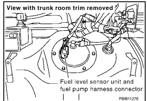
4. Check voltage between fuel level sensor unit and fuel pump terminal 5 and ground with CONSULT-II or a tester.
