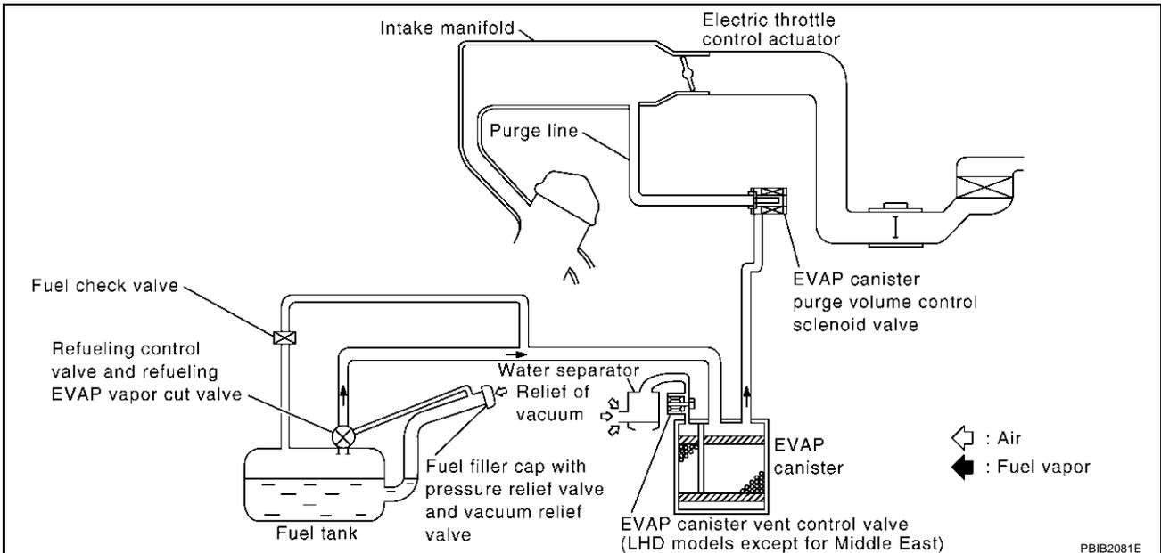
The evaporative emission system is used to reduce hydrocarbons emitted into the atmosphere from the fuel system. This reduction of hydrocarbons is accomplished by activated charcoals in the EVAP canister.
