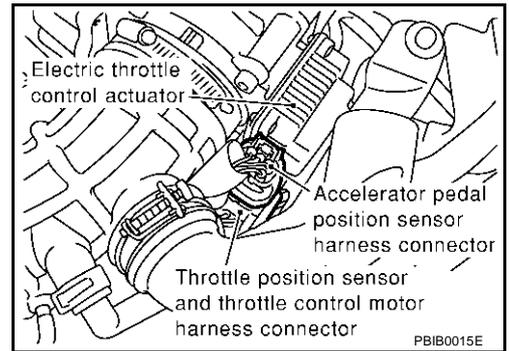
3. Check voltage between electric throttle control actuator terminals 7, 10 and ground with CONSULT-II or tester.
