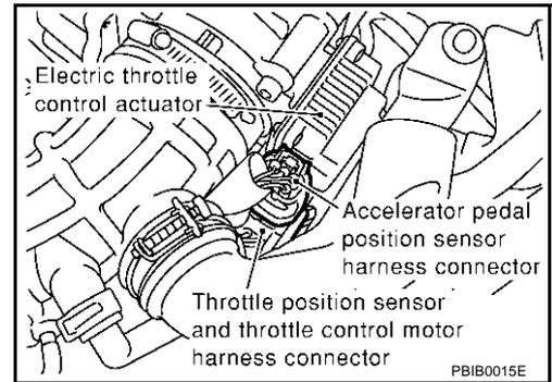
3. Check voltage between electric throttle control actuator terminal 7 and ground with CONSULT-II or tester.
