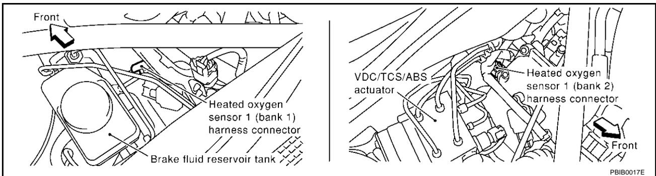
2. Check harness continuity between HO2S1 terminal 4 and engine ground. Refer to Wiring Diagram.
