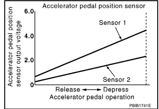
Idle position of the accelerator pedal is determined by the ECM receiving the signal from the accelerator pedal position sensor. The ECM uses this signal for the engine operation such as fuel cut.
