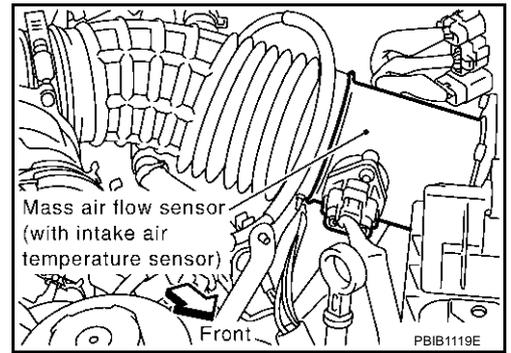
3. Check voltage between MAF sensor terminals 2, 4 and ground with CONSULT-II or tester.
