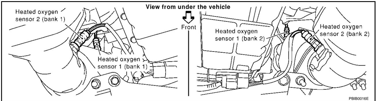
**Tightening torque: 40 - 50 N·m (4.1 - 5.1 kg·m, 30 - 37 ft·lb)**
