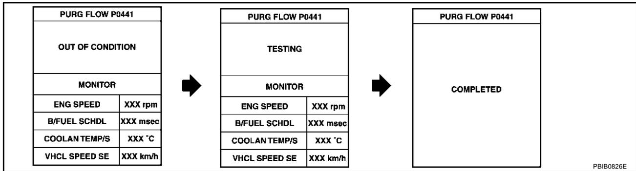
If "TESTING" is not changed for a long time, retry from step 2.
