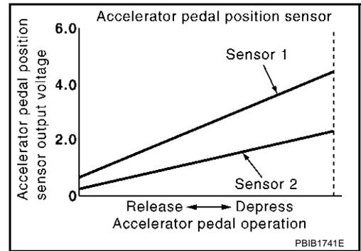
Idle position of the accelerator pedal is determined by the ECM receiving the signal from the accelerator pedal position sensor. The ECM uses this signal for the engine operation such as fuel cut.
