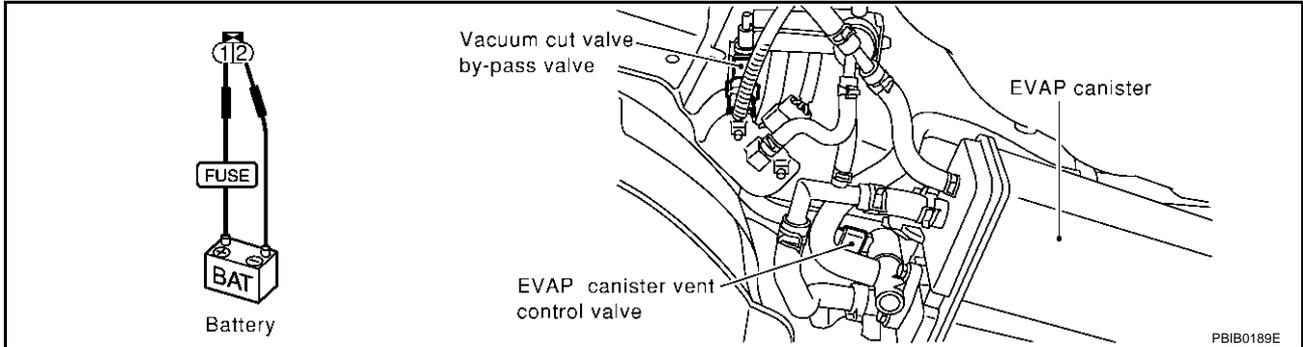
4. Pressurize the EVAP line using pressure pump with 1.3 to 2.7 kPa (10 to 20 mmHg, 0.39 to 0.79 inHg), then remove pump and EVAP service port adapter.
