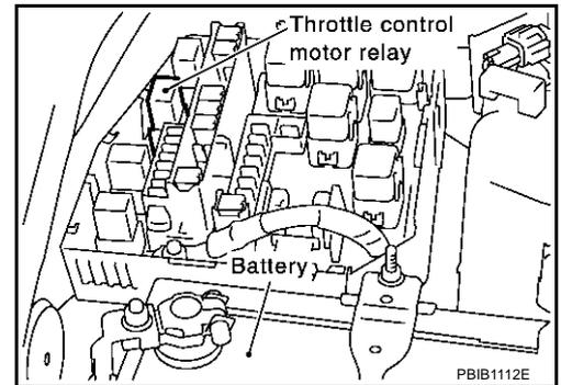
2. Check voltage between throttle control motor relay terminals 2, 5 and ground with CONSULT-II or tester.
