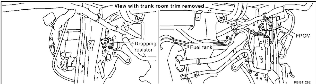
4. Check harness continuity between fuel pump relay terminal 5 and fuel pump terminal 3, fuel pump terminal 1 and dropping resistor terminal 2, dropping resistor terminal 1 and body ground. Refer to Wiring Diagram.
