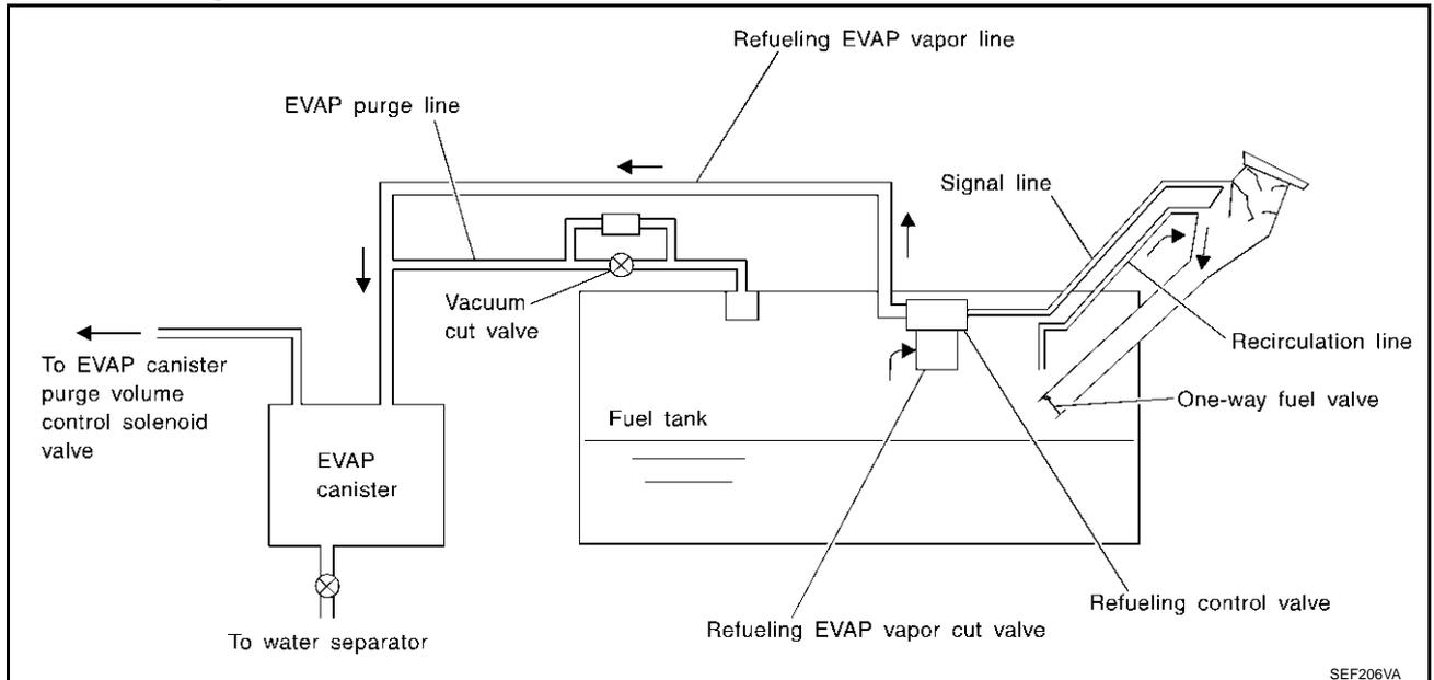
From the beginning of refueling, the fuel tank pressure goes up. When the pressure reaches the setting value of the refueling control valve (RCV) opening pressure, the RCV is opened. After RCV opens, the air and vapor inside the fuel tank go through refueling EVAP vapor cut valve, RCV and refueling vapor line to the EVAP canister. The vapor is absorbed by the EVAP canister and the air is released to the atmosphere.
