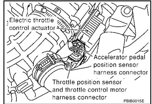
3. Check voltage between electric throttle control actuator terminal 1 and ground with CONSULT-II or tester.
