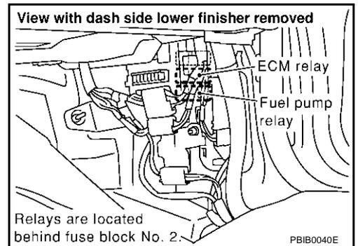
4. Check voltage between terminals 2, 3 and ground with CONSULT-II or tester.
