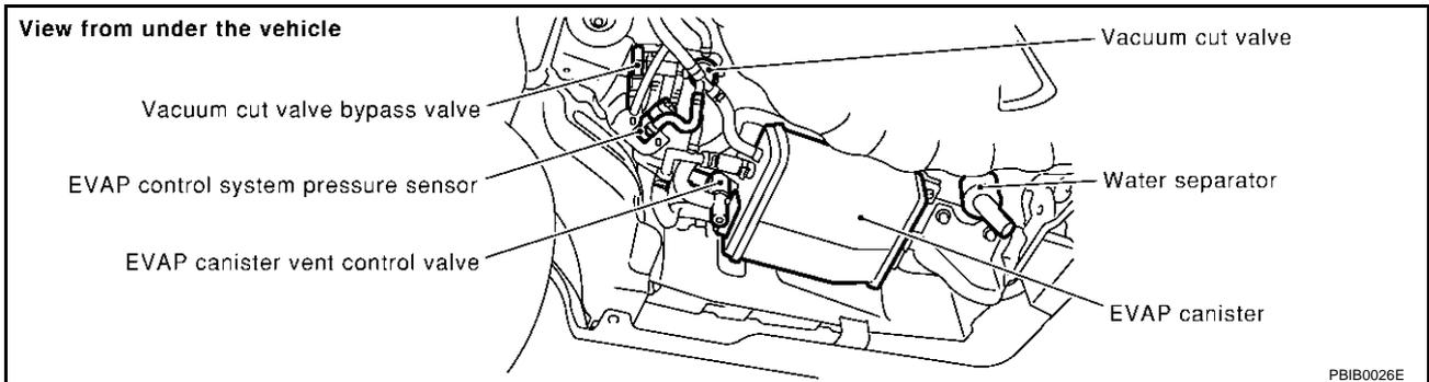
3. Check the rubber tube for clogging.
