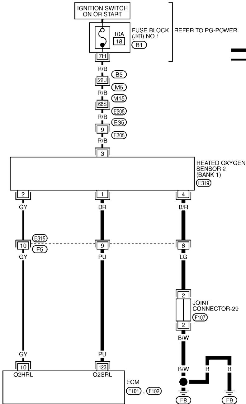
— : DETECTABLE LINE FOR DTC
