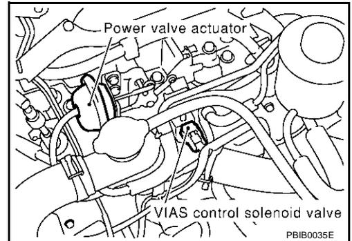
4. Check voltage between terminal 1 and ground with CONSULT-II or tester.
