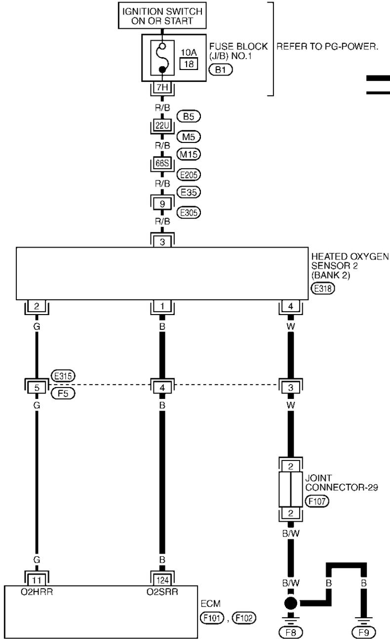
**—** : DETECTABLE LINE FOR DTC
