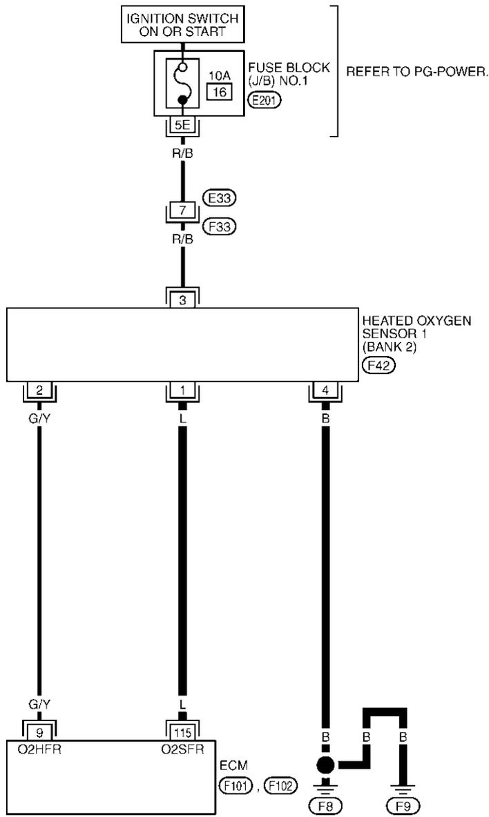
— : DETECTABLE LINE FOR DTC
