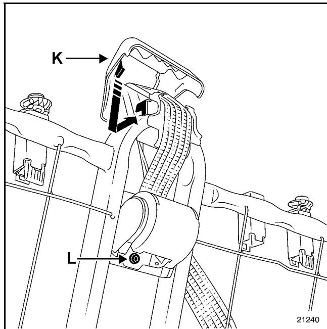
Unclip the belt guide at (K).
