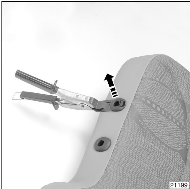
Unclip the four head restraint guide covers.
