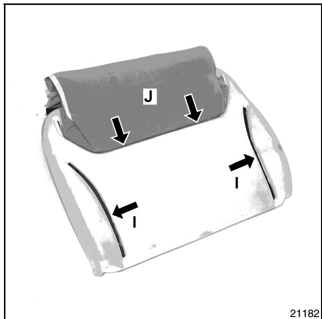
Simultaneously pull back the front and back of the seat cover upwards on the seatback.
