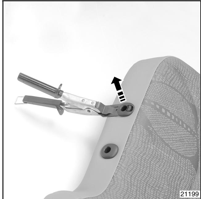
Unclip the four head restraint guide covers.
