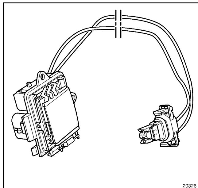
The power module controls the speed of the blower depending on the requirements determined by the automatic control.
