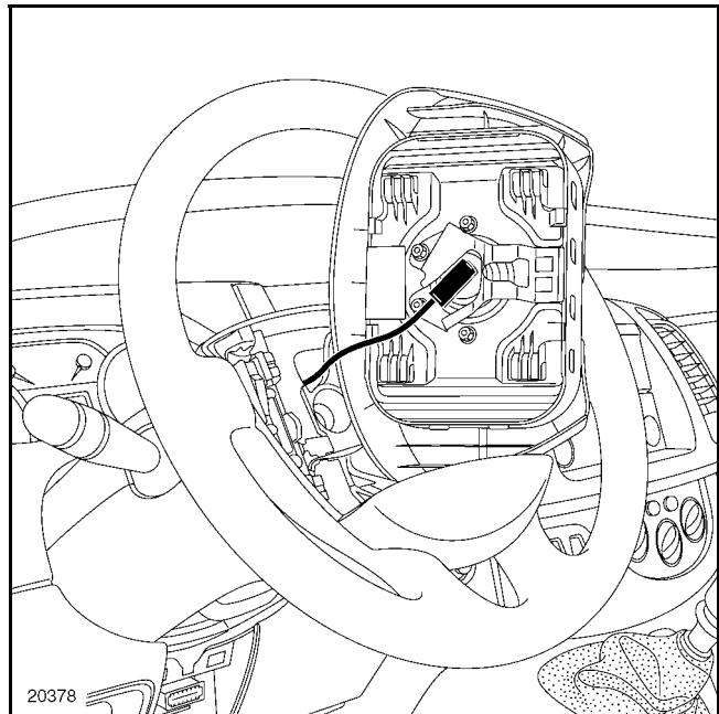
Connect the connector, the lock it.
