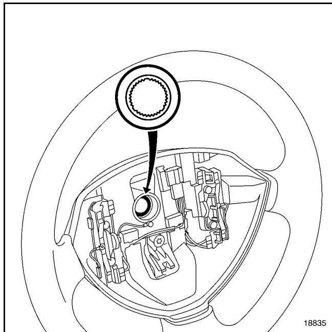
It is essential to replace the steering wheel bolt each time it is removed and to tighten it to a torque of **4.4 daNm**.
