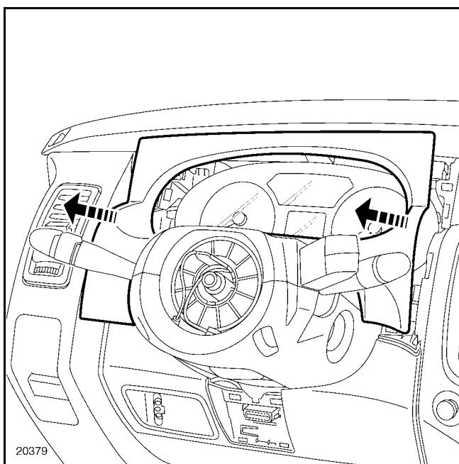
Unclip the instrument panel visor.
