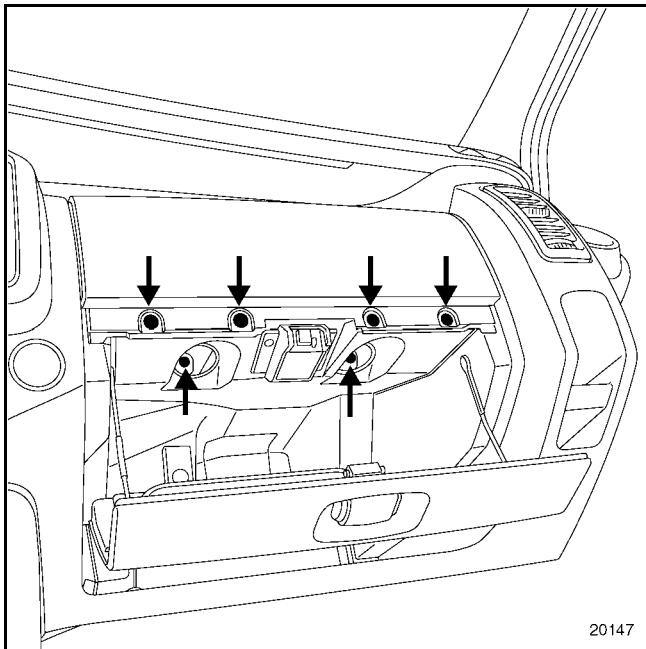
Remove the six mounting bolts from the passenger air bag.
