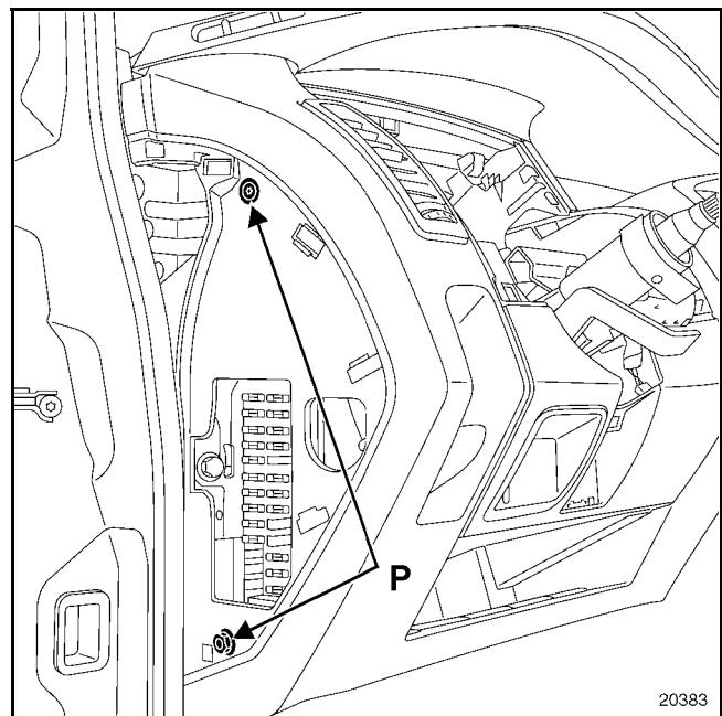
Remove the four side mounting bolts (P).
