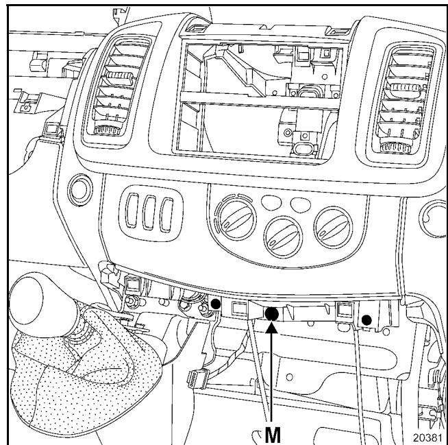
Remove the mounting bolt (M).
