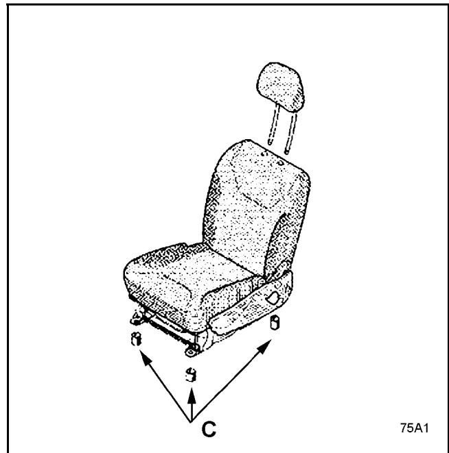
When refitting the seat and the front bench seat, ensure that seat and front bench seat height adjustment spacers (C) are replaced.
