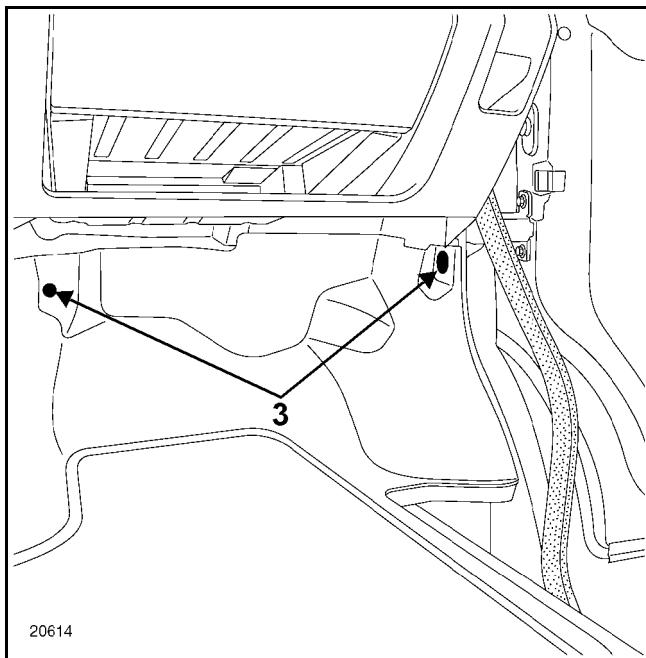
Remove the two clips (3) then partially remove the carpet and fold it back.
