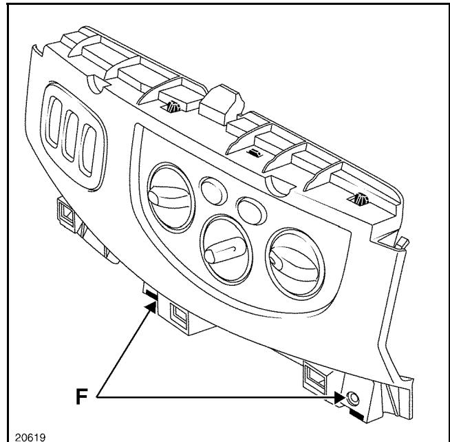
Remove lower mounting (I) and remove the control panel.
