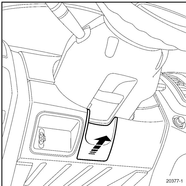
Unclip the cover under the steering wheel.
