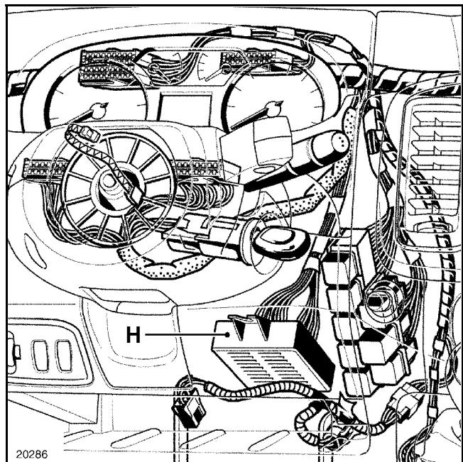
Disconnect the UCH (H) (it is located close to the steering column).
