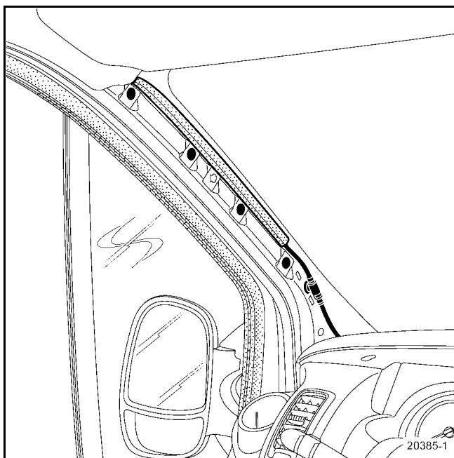
Disconnect the antenna connector.
