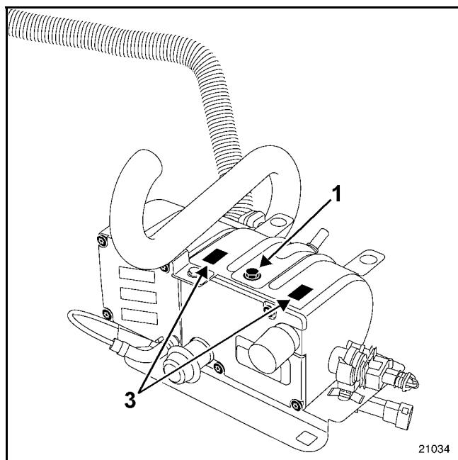
Unscrew bolt (2) and remove the heater from its mounting by releasing lugs (3).
