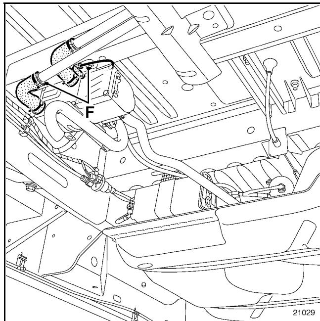
**Removal of the heater from its bracket**
