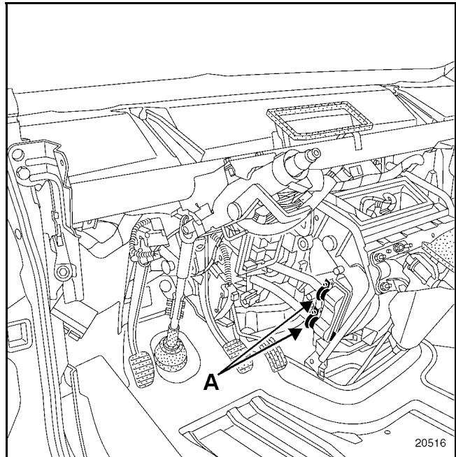
Remove the electric wiring harness and the relay plate (mountings linked to the reinforcer beam).
