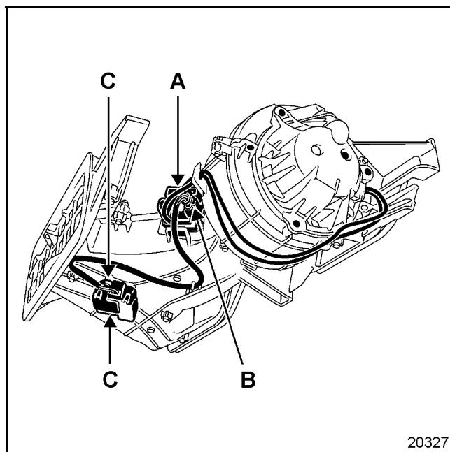
The recirculation motor positions the air inlet flap according to the requirements determined by the automatic control.
