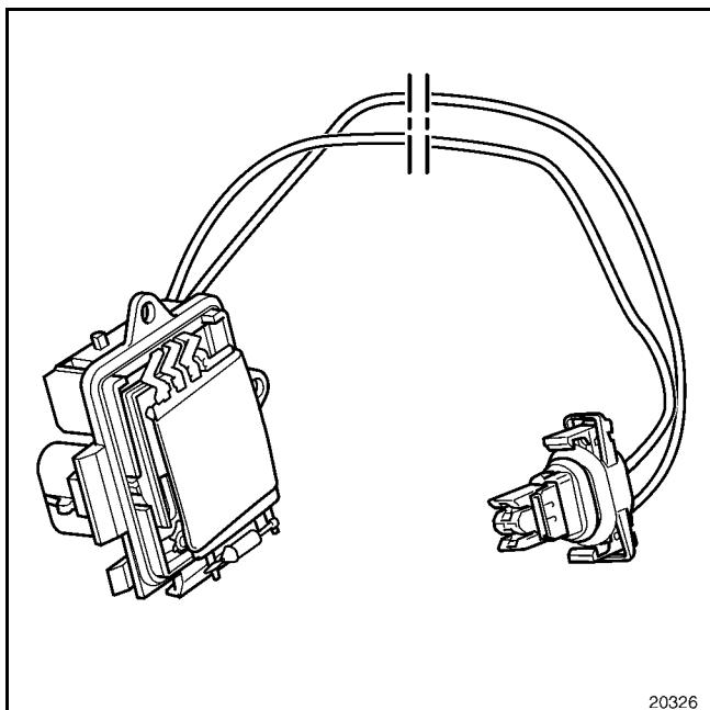
The power module controls the speed of the fan assembly depending on the requirements determined by the automatic control.
