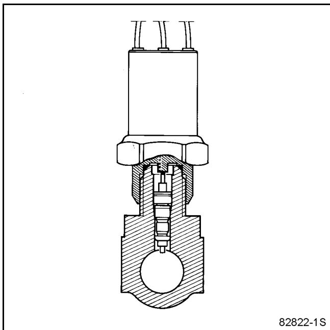
The pressure sensor fitted at the condenser inlet protects the refrigerant circuit.
