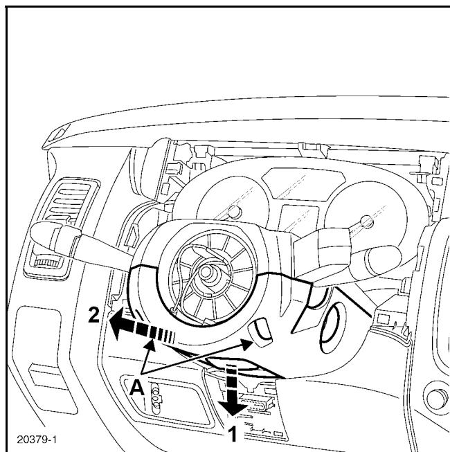
Remove the two mounting bolts (A).
