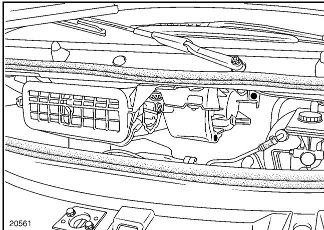
Fit a hose clamp on each refrigerant hose on the radiator in front of the heater matrix bleed screws.
