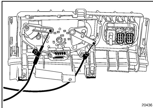
**Temperature adjustment dial control wire on the distribution unit side.**
