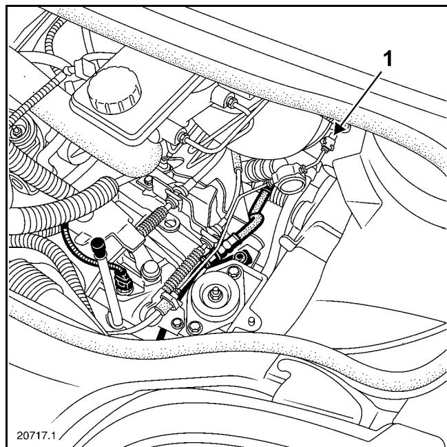
Place a cloth under the master cylinder then disconnect the master cylinder connection pipe and fit plugs to each port.
