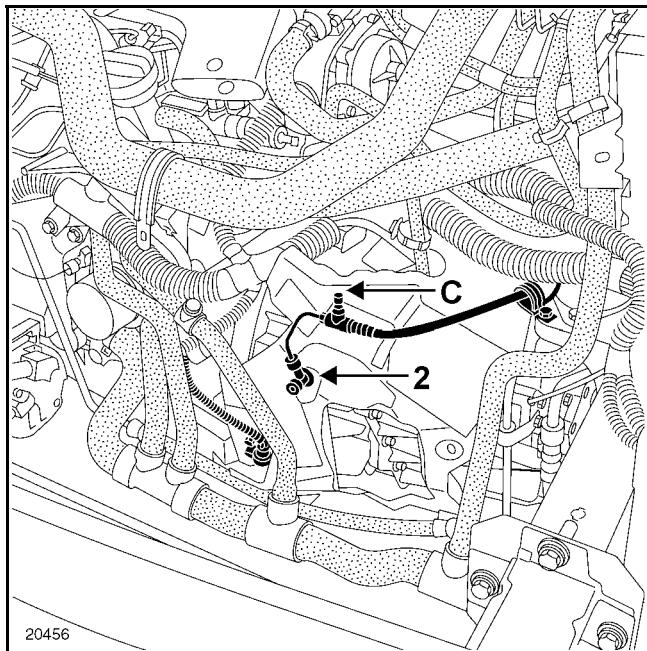
Place a cloth under the slave cylinder then disconnect the slave cylinder connection pipe (C) and fit plugs to each port.
