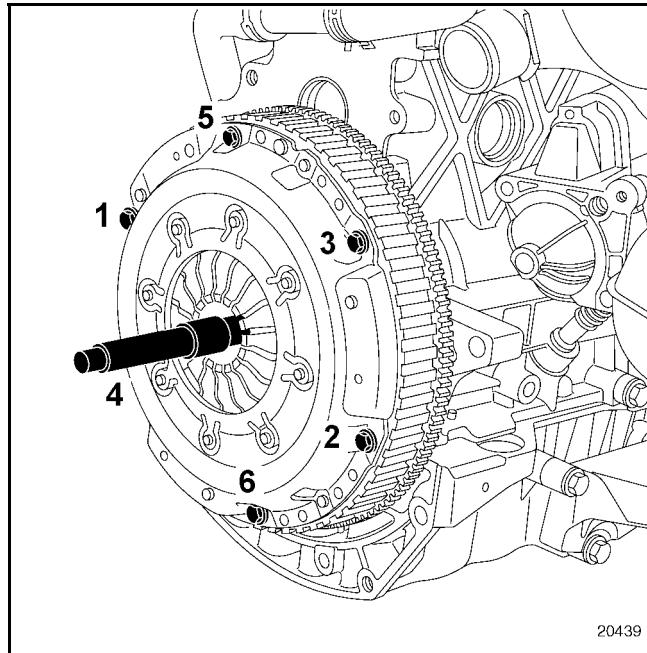
Gradually tighten the bolts in the order indicated in the diagram above, then lock the mechanism securing bolts to torque.
