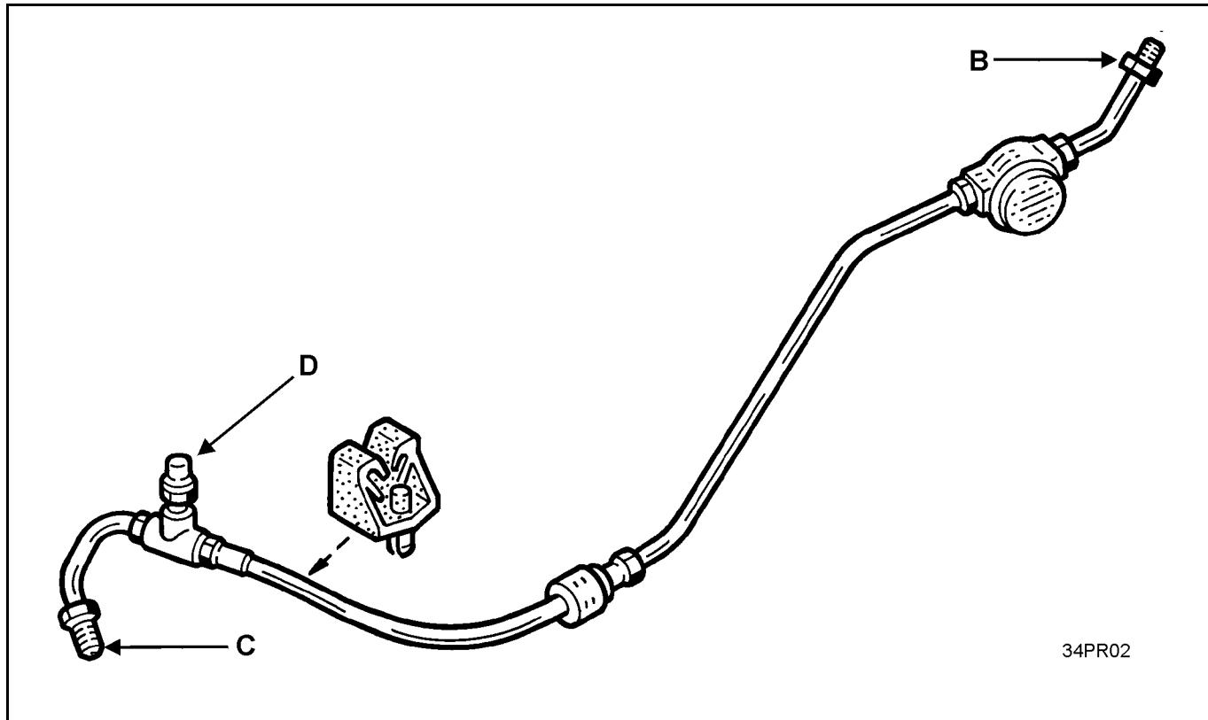
Remove the master-slave connecting pipe holding clip (2) on the slave.
