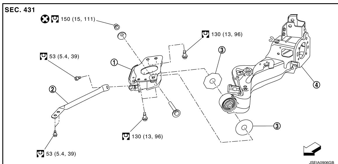
① Suspension arm bracket      ② Suspension bar      ③ Arm stopper
