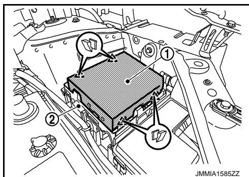
5. Disconnect the connector and remove IPDM E/R from the vehicle.
