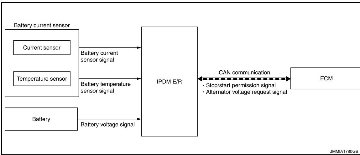
IPDM E/R has an energy management system that recognizes the battery status from the battery current signal from the battery current sensor, the battery temperature sensor signal, and the battery voltage from the battery and maintains normal battery status. Refer to the following for details.
