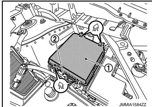
4. Pull up IPDM E/R ① with disengaging the pawls of IPDM E/R cover D ②
