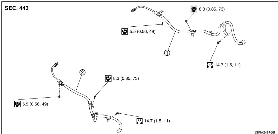
① Parking brake actuator harness RH   ② Parking brake actuator harness LH
