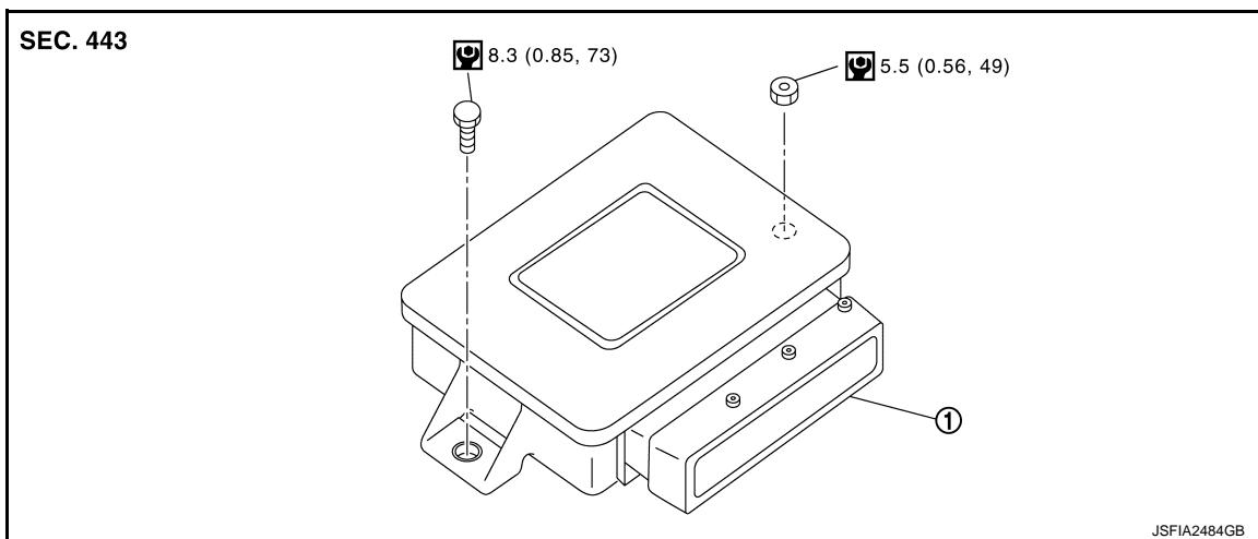
① Electric parking brake control module
