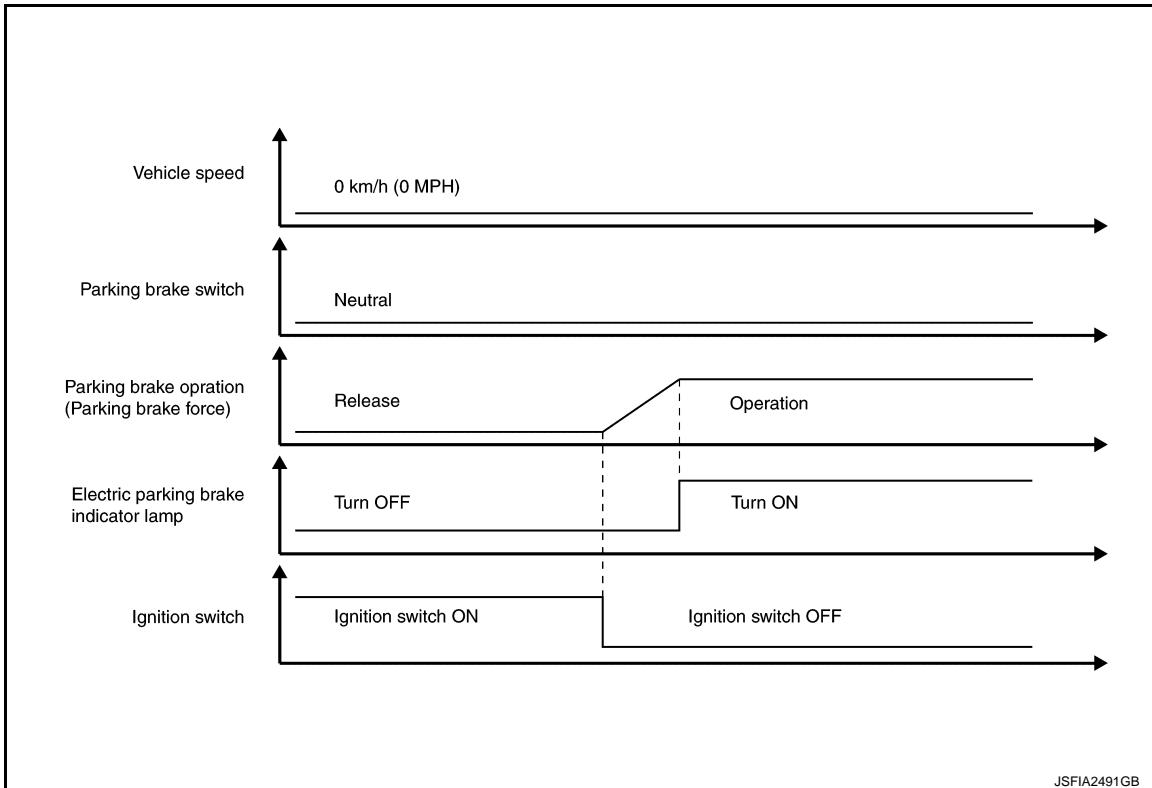
The parking brake automatically operates when vehicle is under the following conditions.
