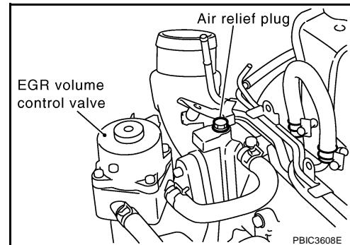
3. Fill radiator and reservoir tank to the specified level.
