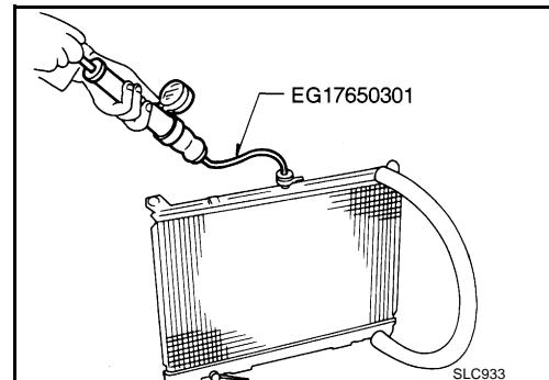
2. Check for leakage by soaking radiator in water container with the testing pressure applied.
