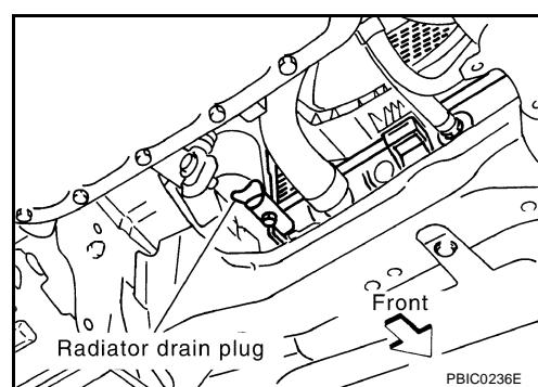
**When draining all engine coolant in the system, open water drain plug on engine cylinder block. Refer to EM-231, "DISASSEMBLY".**
