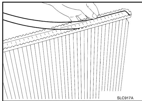
3. Caulk tank in numerical order as shown in the figure with radiator plate pliers A (special service tool).
