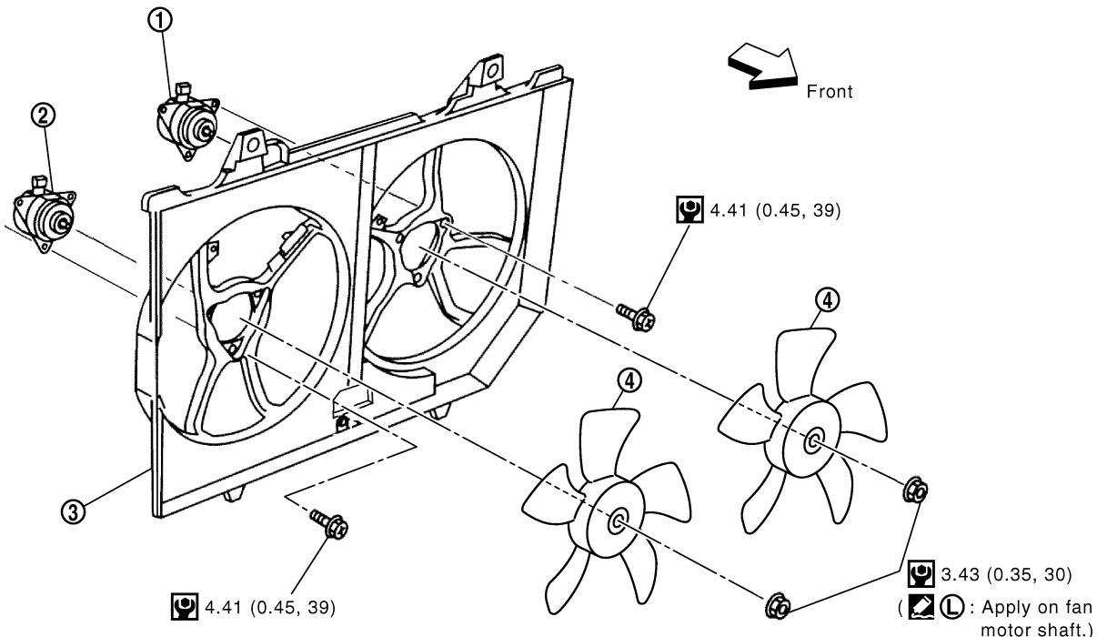
(L) : Apply thread locking sealant.
