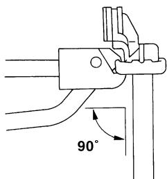
Keep Tool perpendicular to the radiator.
