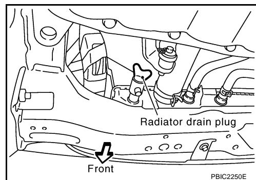
When drain all of engine coolant in the system, open water drain plug on cylinder block. Refer to [EM-94, "ASSEMBLY"](#).
