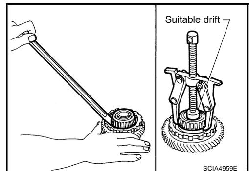
6. Remove idler gear bearing outer race from transaxle case.
