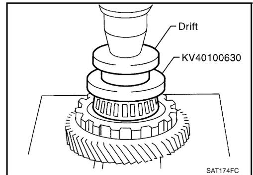
5. Install idler gear bearing outer race on transaxle case.
