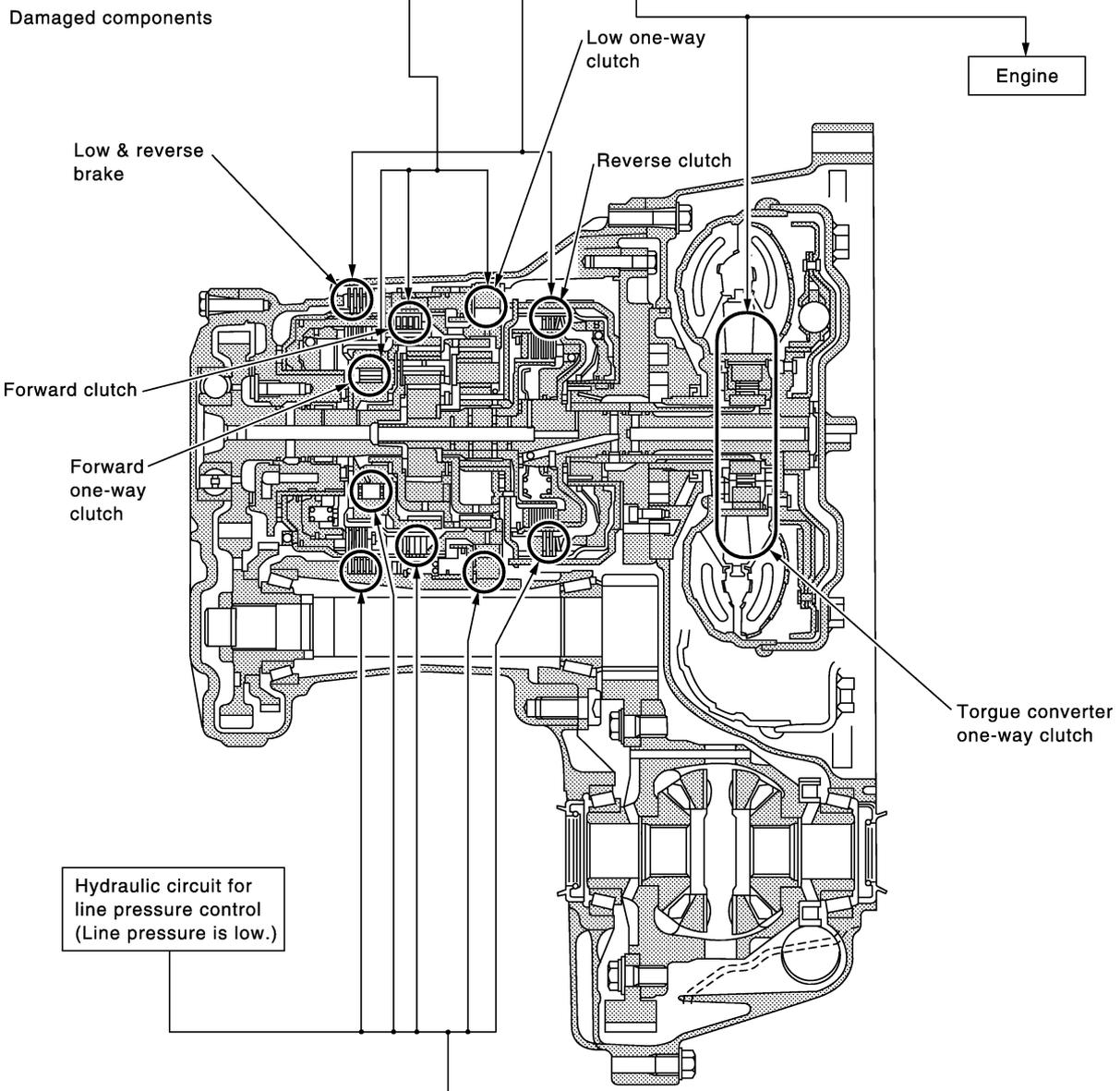
Hydraulic circuit for line pressure control
