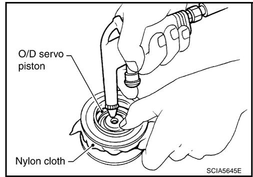
5. Remove D-ring from O/D servo piston.
