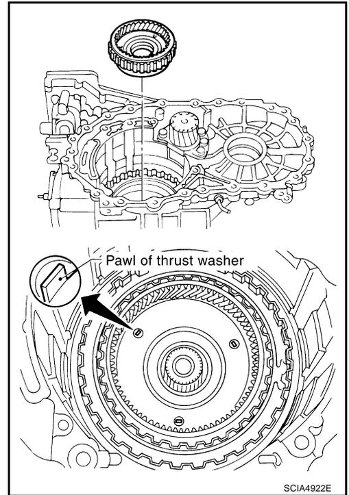
10. Install rear planetary carrier assembly and rear sun gear according to the following procedures.
