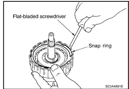
5. Set SST on spring retainer and remove snap ring from input shaft assembly (high clutch drum) while compressing return springs.
