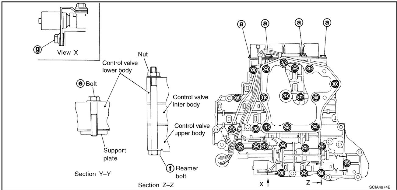
a. Install and tighten bolts **b** and nut **f** to specified torque.
