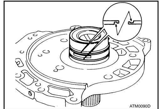
2. Loosen bolts in a crisscross pattern and remove oil pump cover.
