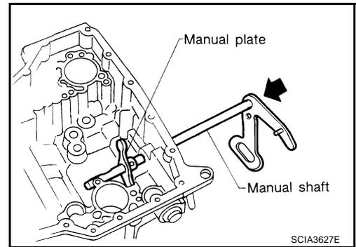
5. Align groove of manual shaft and hole of transaxle case.
