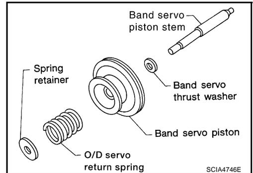
3. Place band servo piston stem end on a wooden block. While pushing spring retainer down, install E-ring.
