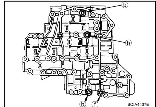
5. Remove control valve lower body from control valve inter body.
