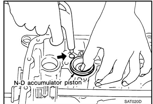
20. Check accumulator pistons and contact surface of transaxle case for damage.
