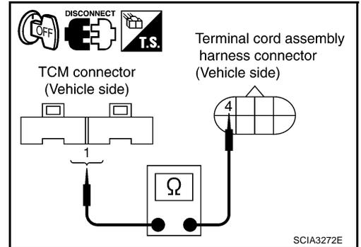
4. Check continuity between terminal cord assembly harness connector and dropping resistor harness connector.
