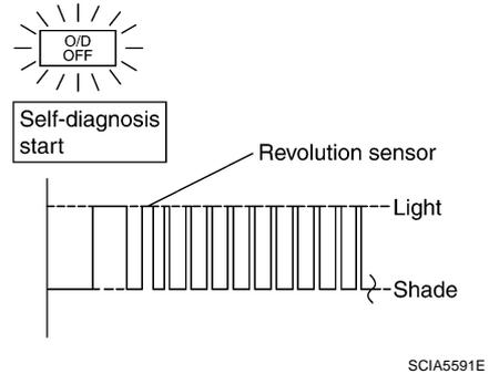
Revolution sensor circuit is short-circuited or disconnected.
