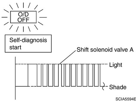
Shift solenoid valve A circuit is short-circuited or disconnected.
