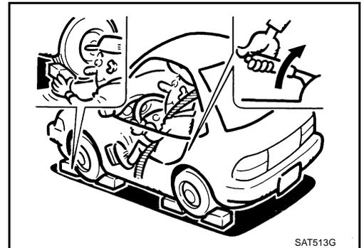
5. Start engine, apply foot brake, and place selector lever in D position.
