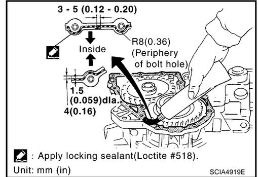
☑ : Apply locking sealant(Loctite #518).
