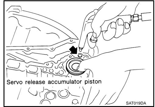
18. Remove N-D accumulator piston and return spring with compressed air.
