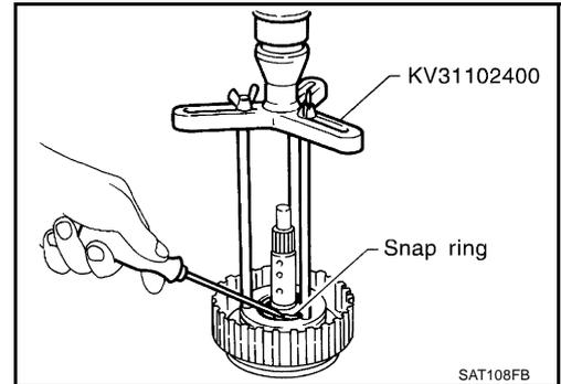
7. Remove high clutch piston from input shaft assembly (high clutch drum) by turning it.
