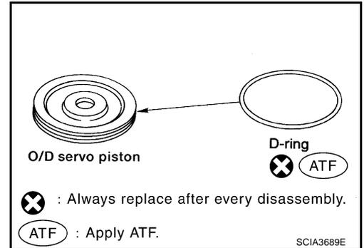
7. Install O/D servo piston to O/D servo piston retainer fitting the installation direction on it.
