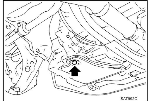
4. Disconnect terminal cord assembly harness connector.
