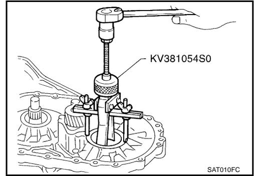
14. Insert SST and measure turning torque of final drive assembly.
