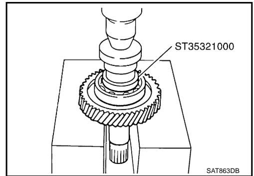
7. Press needle bearing on bearing retainer.
