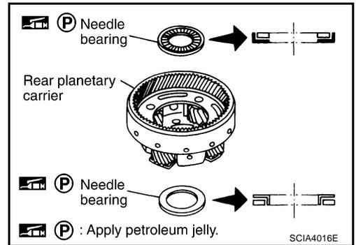
e. Check clearance between pinion washer and rear planetary carrier with feeler gauge.
