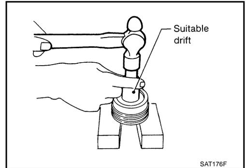
8. Install snap ring to bearing retainer.
