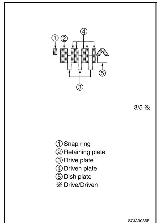
7. Install snap ring for overrun clutch.
