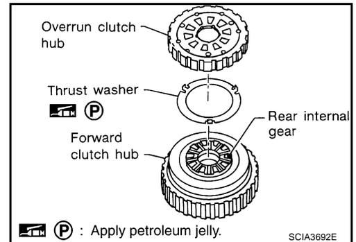
2. Remove forward clutch hub from rear internal gear.
