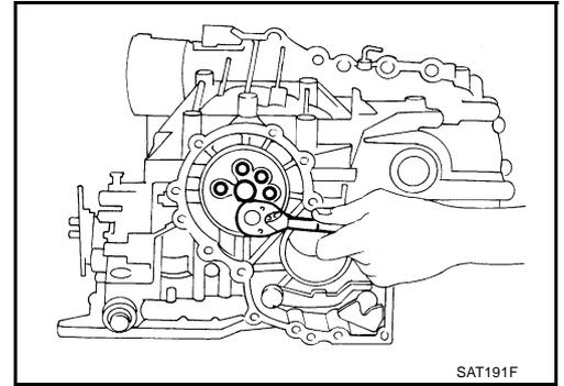
2. Install needle bearing on bearing retainer.
