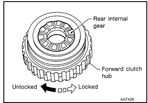
9. Install forward clutch hub and rear internal gear on transaxle case.
