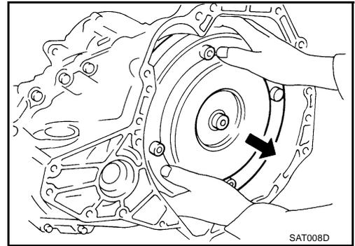
3. Check torque converter one-way clutch using check tool as shown in the right figure.
