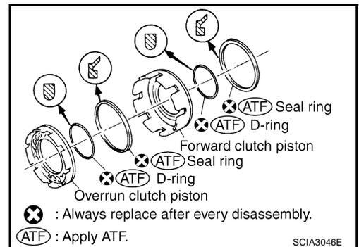
2. Install overrun clutch piston on forward clutch piston by turning it slowly.
