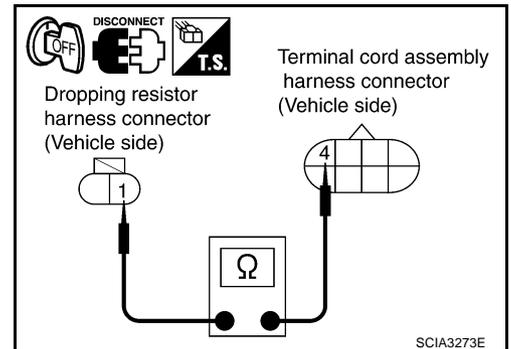
5. Check continuity between dropping resistor harness connector terminal and TCM connector terminal.
