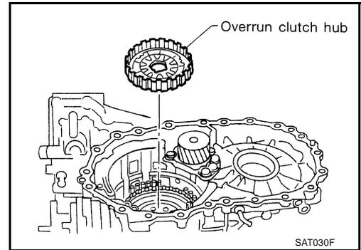
40. Remove needle bearing from overrun clutch hub and check for damage or wear.
