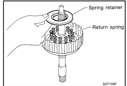
4. Set SST on spring retainer and install snap ring while slowly compressing return springs.
