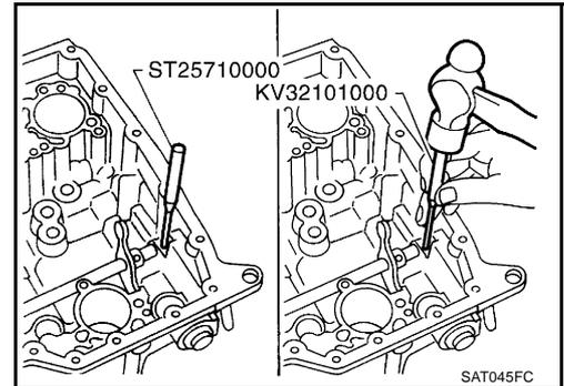
7. Set parking rod plate onto manual shaft and drive retaining pin.
