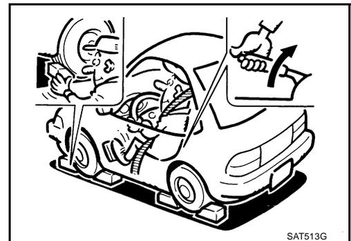
5. Start engine and measure line pressure at idle and stall speed.
