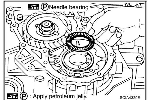
3. Install output shaft on transaxle case.
