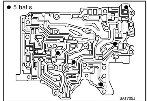
13. Check to see that steel balls are properly positioned in control valve upper body and then remove them.
