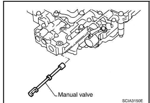
9. Disassemble and inspect control valve assembly if necessary. Refer to [AT-448, "Control Valve Assembly"](#), [AT-457, "Control Valve Upper Body"](#) and [AT-461, "Control Valve Lower Body"](#).
