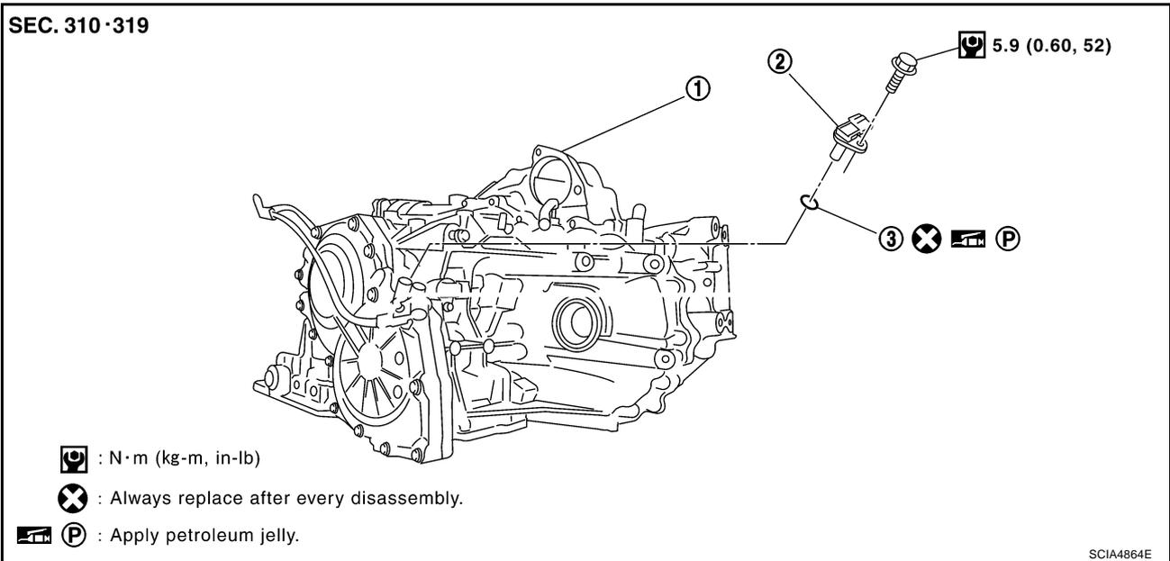
1. transaxle assembly                      2. Revolution sensor                      3. O-ring
