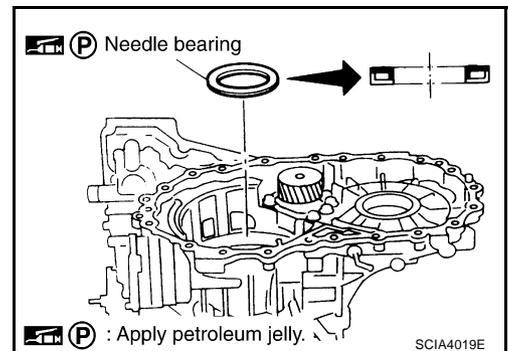
43. Remove output shaft assembly according to the following procedures.
