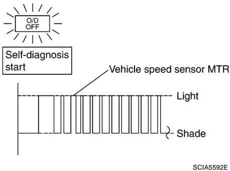
Vehicle speed sensor circuit is short-circuited or disconnected.
