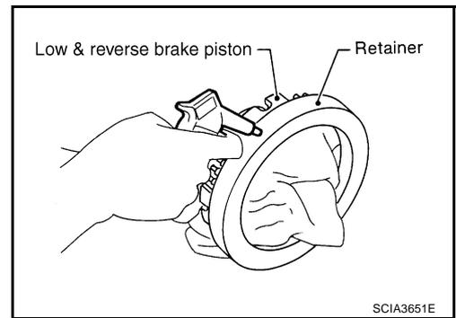
7. Remove D-rings from low & reverse brake piston.
