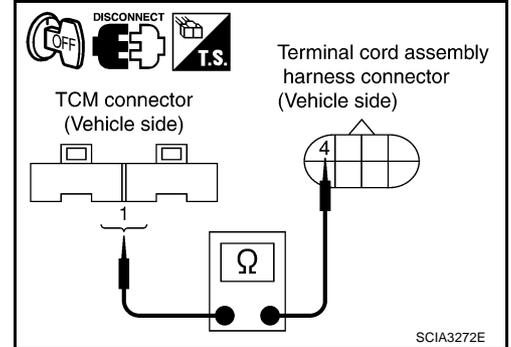
4. Check continuity between terminal cord assembly harness connector terminal and dropping resistor harness connector terminal.
