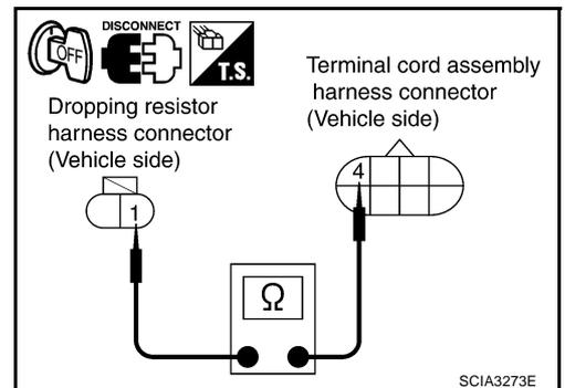
5. Check continuity between dropping resistor harness connector and TCM connector.
