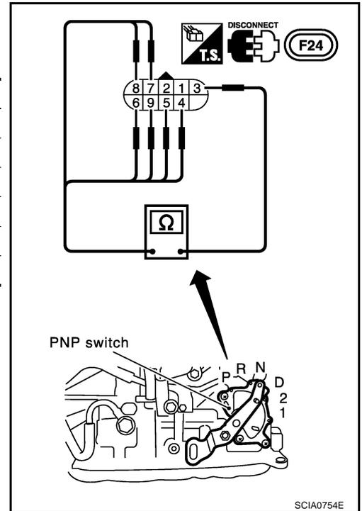
2. If NG, check again with manual control cable disconnected from manual shaft of A/T assembly. Refer to step 1.
