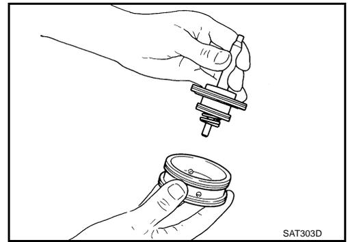
6. Install D-ring to O/D servo piston.
