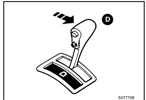
6. Accelerate to wide open throttle gradually while applying foot brake.
