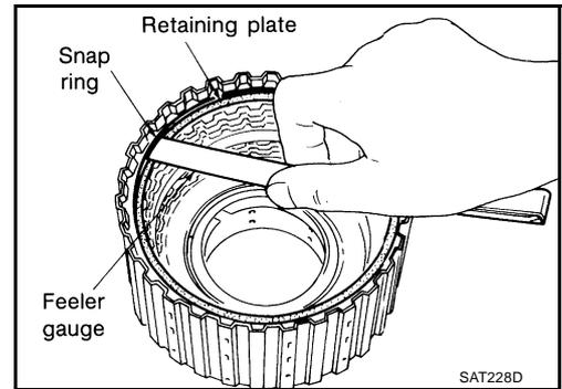
12. Check operation of forward clutch and overrun clutch. Refer to [AT-475, "DISASSEMBLY"](#).
