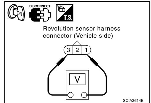
5. Check voltage between revolution sensor harness connector terminal and ground.
