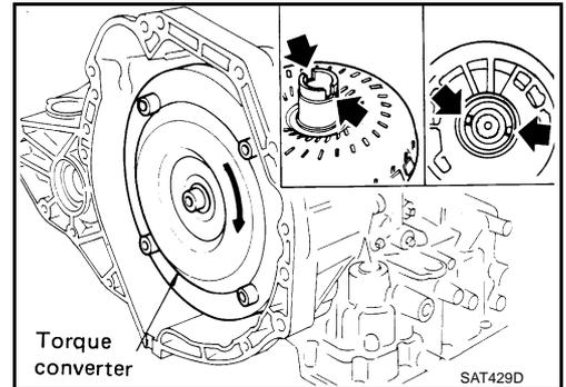
c. Measure distance "A" to Make sure that torque converter is in proper position.
