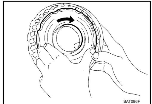
3. Install return springs and spring retainer on reverse clutch piston.
