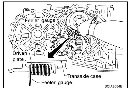
6. Install low & reverse brake piston (with retainer) and spring retainer on transaxle case.
