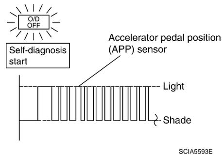
Accelerator pedal position (APP) sensor circuit is short-circuited or disconnected.
