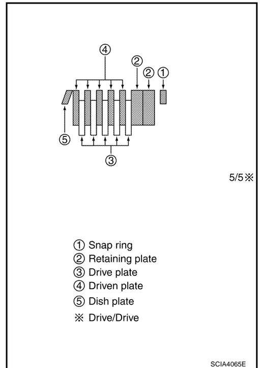
10. Install snap ring for forward clutch.
