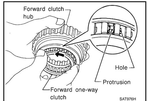
2. Install bearing on forward one-way clutch.
