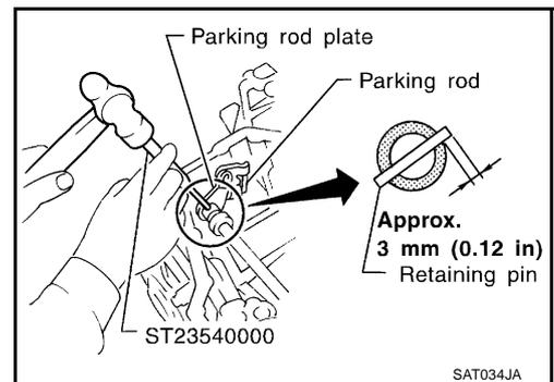
8. Install manual plate retaining pin.
