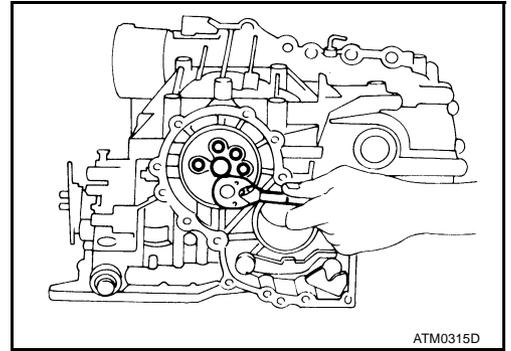
44. Disassemble reduction pinion gear according to the following procedures.
