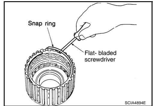
4. Remove snap ring for overrun clutch with flat-bladed screwdriver.
