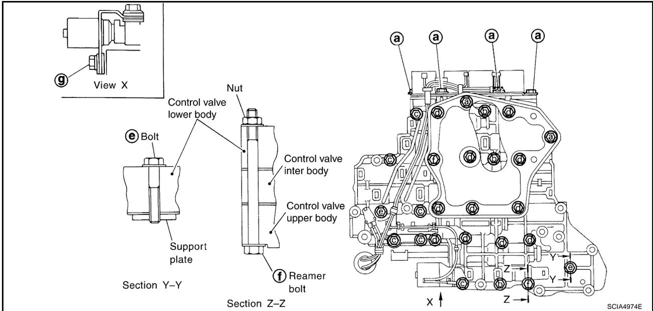
1. Remove bolts **a**, **d**, reamer bolt **f** and nut and remove oil strainer from control valve assembly.
