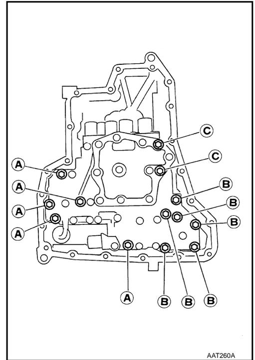
d. Remove control valve assembly from transaxle case.
