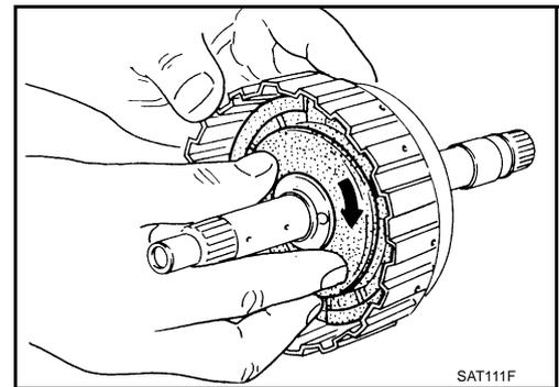
8. Remove D-rings from high clutch piston.
