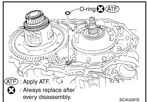
13. Install converter housing on transaxle case.
