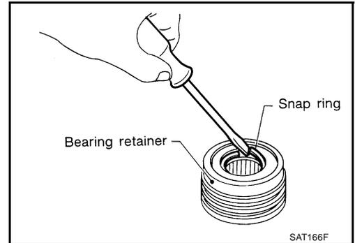
4. Remove needle bearing from bearing retainer.
