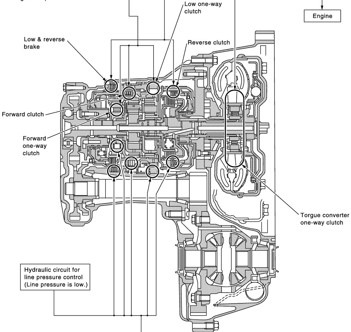
Hydraulic circuit for line pressure control
