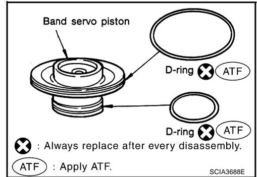
2. Install band servo piston stem, band servo thrust washer, O/D servo return spring and spring retainer to band servo piston.
