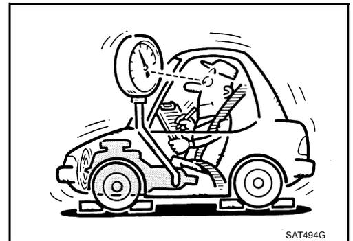
**3. CHECK STALL TEST**Check stall revolution with selector lever in D position. Refer to [AT-65, "Stall Test"](#) .**OK or NG**
