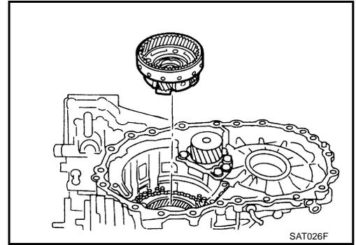
b. Remove rear sun gear from rear planetary carrier.
