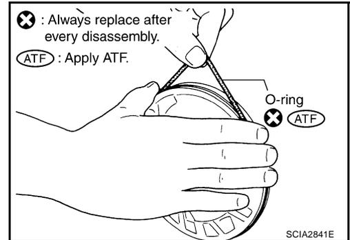
5. Remove oil pump housing oil seal.
