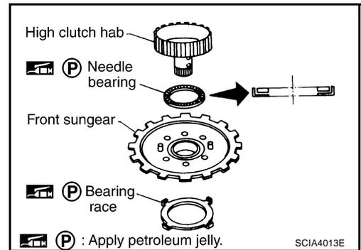
34. Remove needle bearing from transaxle case and check for damage or wear.
