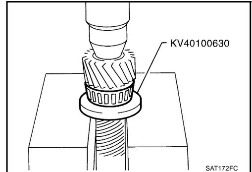
2. Install reduction pinion gear bearing outer race on transaxle case. Refer to [AT-491, "COMPONENTS"](#).
