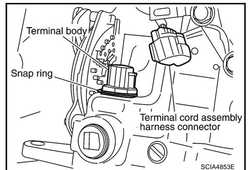
5. Remove snap ring from terminal body.
