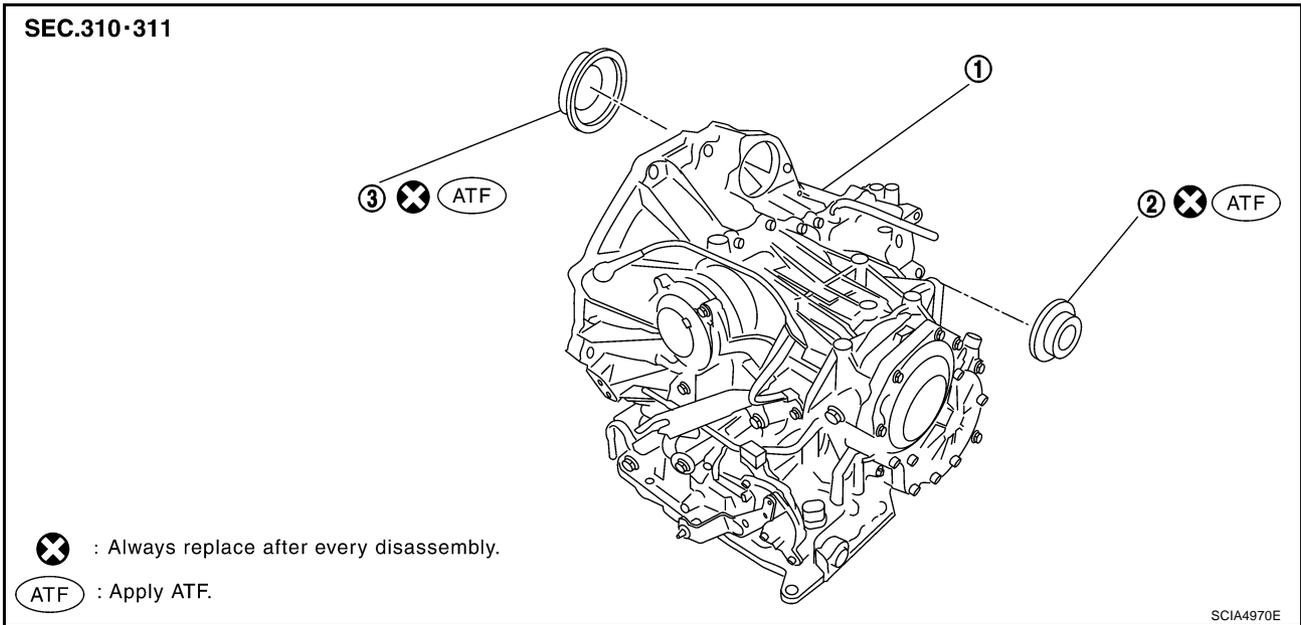
1. transaxle assembly                      2. LH differential side oil seal                      3. RH differential side oil seal
