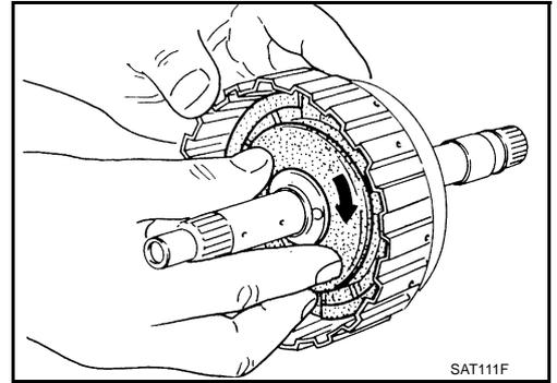
3. Install return springs and spring retainer on high clutch piston.
