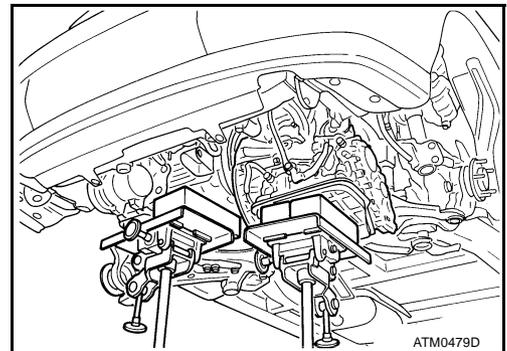
19. Disconnect harness connector and wire harness.
