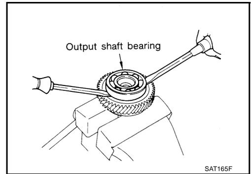
3. Remove snap ring from bearing retainer.
