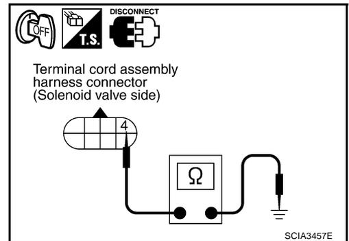
**4. CHECK HARNESS BETWEEN TCM AND TERMINAL CORD ASSEMBLY HARNESS CONNECTOR**
