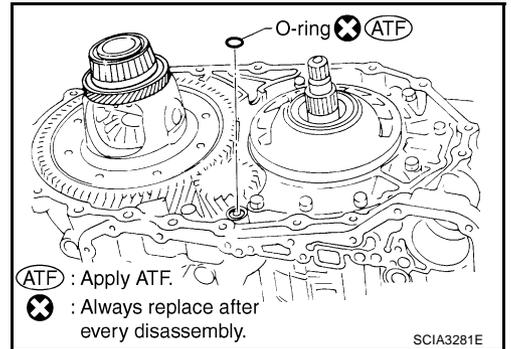
25. Remove final drive assembly from transaxle case.
