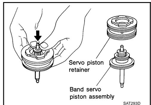
8. Place band servo piston stem end on a wooden block. While pushing spring retainer down, remove E-ring.
