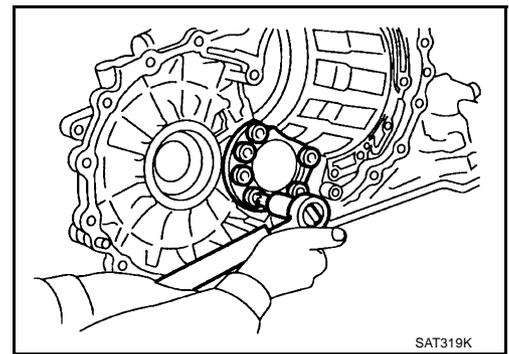
4. Press idler gear bearing inner race on idler gear.
