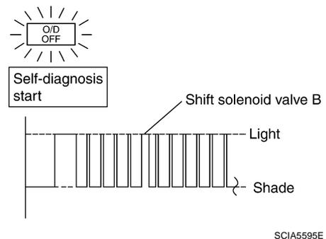
Shift solenoid valve B circuit is short-circuited or disconnected.
