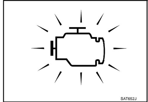
2. When the engine is started, the malfunction indicator should go off.
