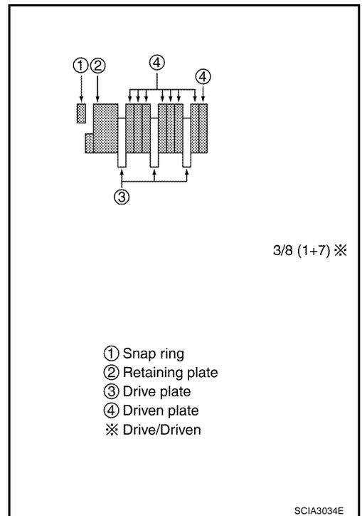
6. Install snap ring with flat-bladed screwdriver.
