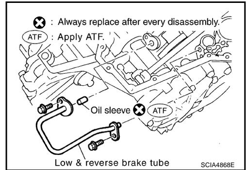
17. Install control valve assembly.
