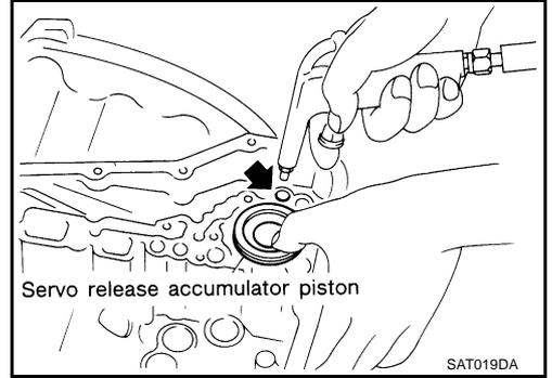
13. Blow air into the oil hole shown in the figure and remove N-D accumulator piston and return spring from transaxle case.
