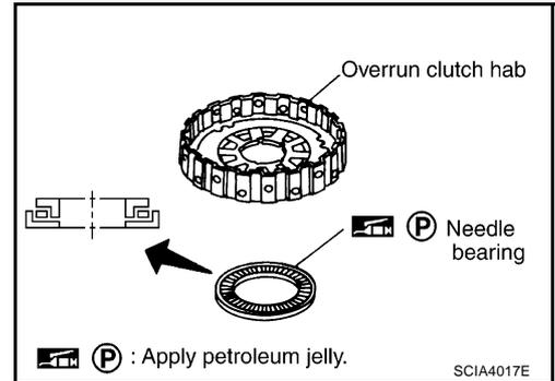
41. Remove forward clutch assembly and overrun clutch assembly from transaxle case.
