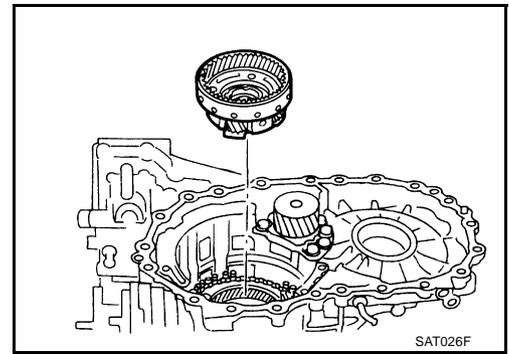
11. Install needle bearing on front planetary carrier, then install them together on transaxle case.
