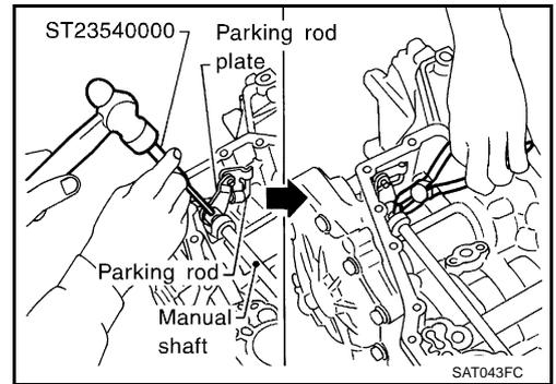
7. Pull out manual shaft retaining pin.
