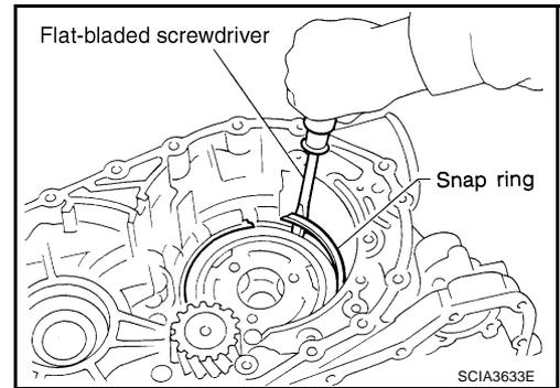
15. Install front sun gear according to the following procedures.
