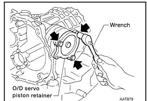
2. Apply compressed air to oil hole in transaxle case to remove O/D servo piston retainer and band servo piston assembly.
