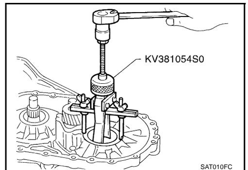
27. Remove differential side bearing adjusting shim from transaxle case.
