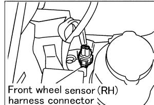
Fix the connector on the engine room (RH).
