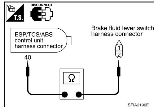
2. Check for the continuity between the brake fluid level warning switch and the ESP/TCS/ABS control unit.
