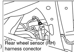
Fix the connector on the rear suspension member (RH).
