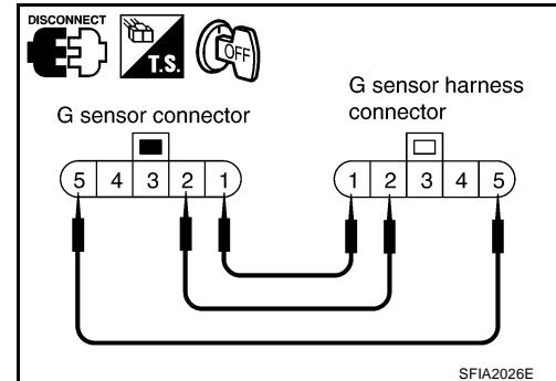
3. Check voltage between the following G sensor terminals when ignition switch turns ON and G sensor is in the following condition.
