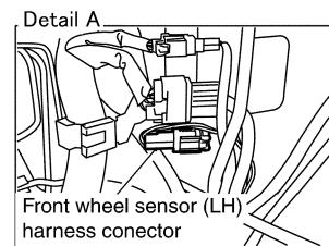
Fix the connector on the engine room (LH).
