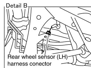
Fix the connector on the rear suspension member (LH).
