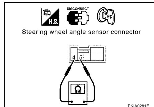
**ESP/TCS/ABS Control Unit Circuit Check**
