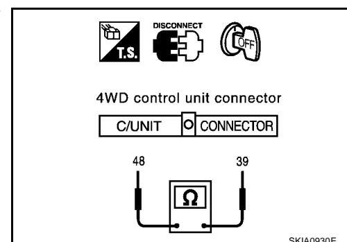
**Steering Wheel Angle Sensor Circuit Check**
