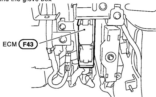
Passenger side view with dash side lower finisher removed
