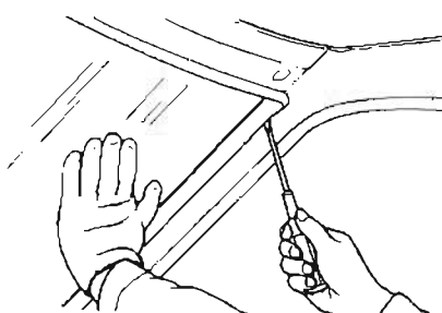
Fig. BF-51 Removing front windshield glass
