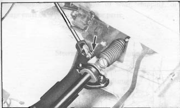
Fig. ST-13 Disconnecting lower joint from pinion
