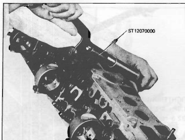
Fig. EM-69 Valve installation
