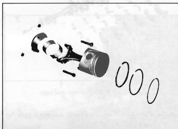
Fig. EM-72 Piston and connecting rod assembly
