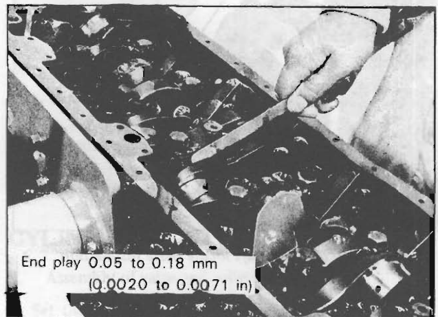
Fig. EM-75 Camshaft end play check
