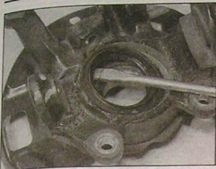
2.13 Prising the oil seal from the rear of the hub carrier
