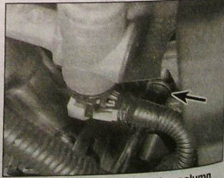
14.10 Unscrewing a steering column upper securing bolt (arrowed)
