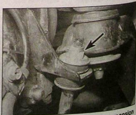
7.10 Anti-roll bar drop link-to-suspension centre link securing nut (arrowed)
