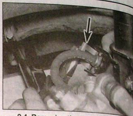
9.4 Removing the brake fluid hose securing clip (arrowed) from the rear strut
