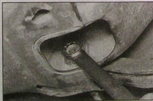
9.30a Unscrew the parallel link inboard securing nut while counterholding the bolt...
