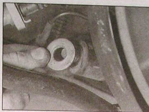
9.28b ... and recover the washer...
