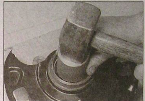
2.15 Driving the bearing from the hub carrier
