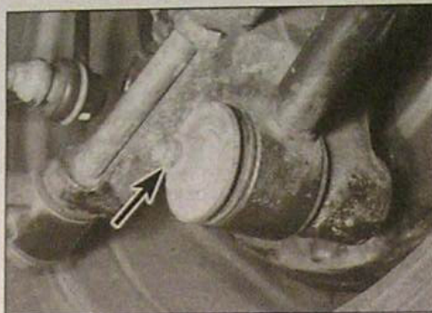
9.40 Radius rod-to-hub carrier nut (arrowed)
