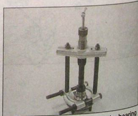
2.11 Using a puller to remove the bearing race from the hub
