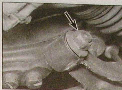
4.4 Lower arm-to-mounting pin nut (arrowed)
