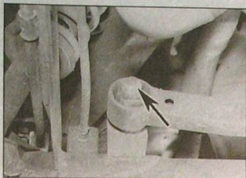
11.54a Lateral link-to-axle beam mounting nut (arrowed)
