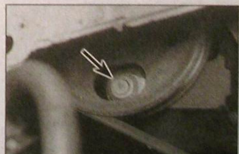
18.6 Turn the pump pulley until one of the holes lines up with the through-bolt (arrowed)
