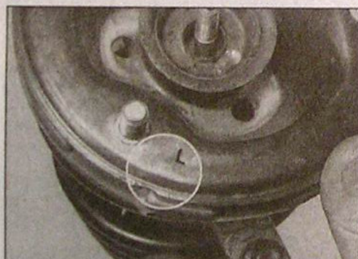
3.16j ... noting that the cut-out marked 'L' must be positioned nearest the inner edge of the suspension turret when the strut is refitted
