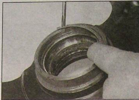
2.14a Removing the outer bearing circlip from the hub carrier
