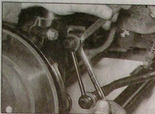
9.2 Unscrewing the anti-roll bar drop link-to-rear suspension strut nut
