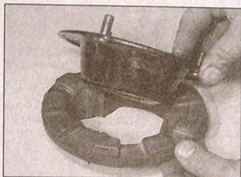
3.16h Fit the upper spring seat to the top mounting ...
