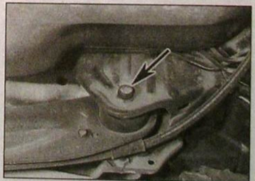
11.31 Unscrew the nuts from the trailing arm front mounting bolts (arrowed) each side
