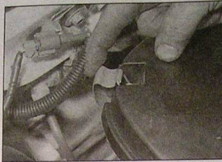
27.1b ... then release the air cleaner lid retaining clips
