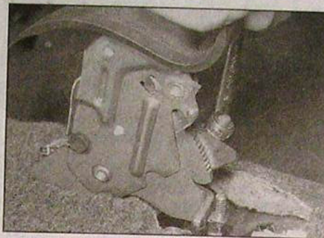
9.12 Using a spanner to turn the handbrake adjuster nut
