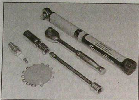
5.4 Tools required for spark plug removal, gap adjustment and refitting
