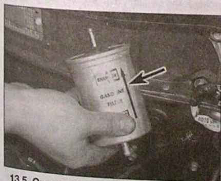
13.5 On refitting, ensure that the filter is fitted the correct way round so its arrow (arrowed) is pointing in the direction of fuel flow
