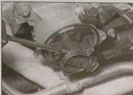
28.9b Slacken and remove the retaining screw, and pull the rotor arm off the shaft
