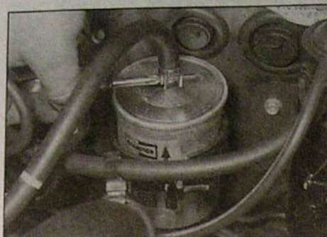
13.2 Slacken the retaining clips and disconnect the hose from the filter ...
