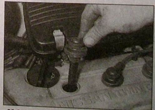
28.3 Ensure that the HT leads are clearly numbered before removing them
