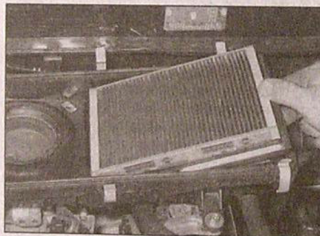
27.3b Removing the air filter element - 1.6 litre fuel injection engine
