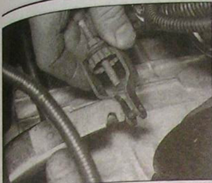
8.6 Free the clutch cable from the release lever, and position it clear of the transmission
