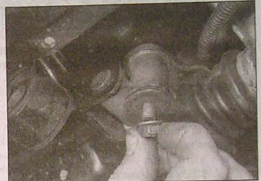
8.8b Unscrew the nut, then withdraw the pivot bolt ...
