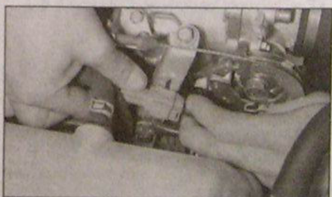
D Check all engine related wiring multi-plugs for security.
