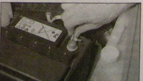
E Check the security and condition of the battery terminals.
