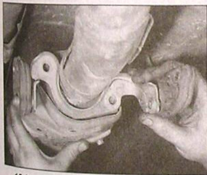
16.8b ... then remove the mounting bracket assembly and front pipe
