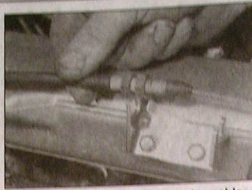
15.22b . . . and release the outer cable from its mounting bracket
