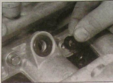
14.6b ... and recover its spacers from the manifold
