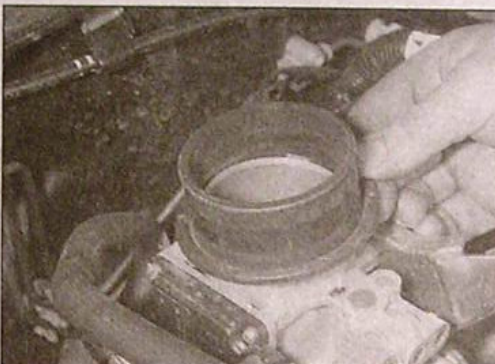
2.4d Recover the sealing ring from the throttle housing and store it with the air cleaner housing
