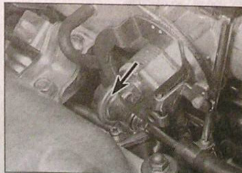
14.10 Slacken the retaining clip and disconnect the return hose from the pressure regulator (arrowed)
