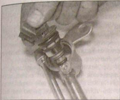
14.7b ... and withdraw the injector from the fuel rail
