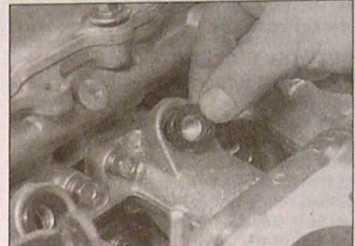
14.9b ... and fit new injector seals to the manifold
