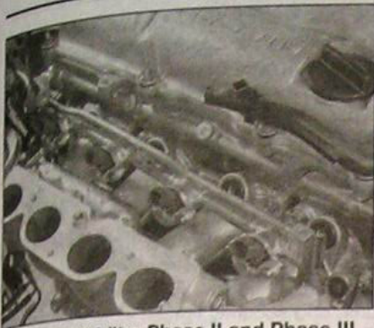
14.6a On 2.0 litre Phase II and Phase III models, remove the fuel rail ...
