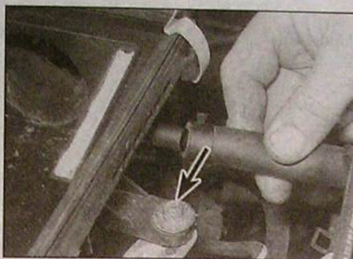
2.4b Disconnect the breather hose then undo the retaining bolt (arrowed) ...
