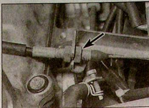
7.2 Slacken the locknut (arrowed) and free the accelerator cable from its mounting bracket
