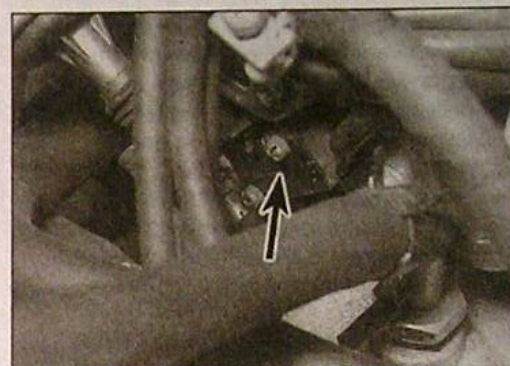
13.8 Throttle valve switch (arrowed) is mounted on the right-hand side of the carburettor
