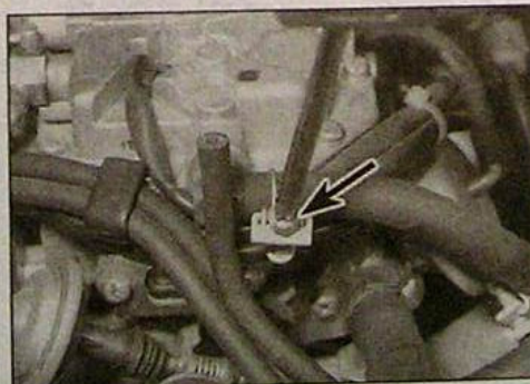
11.5 Slacken the retaining clip (arrowed) and disconnect the fuel hose from the carburettor
