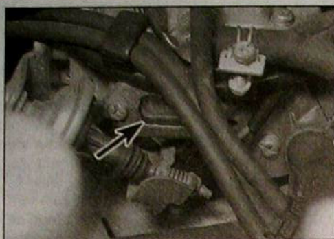
12.25 Float height setting can be checked as described in text using the inspection window (arrowed)
