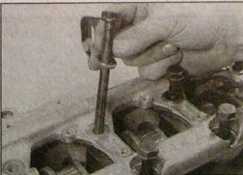
18.34b ... then (where applicable) refit the main bearing ladder, and install the retaining bolts and washers
