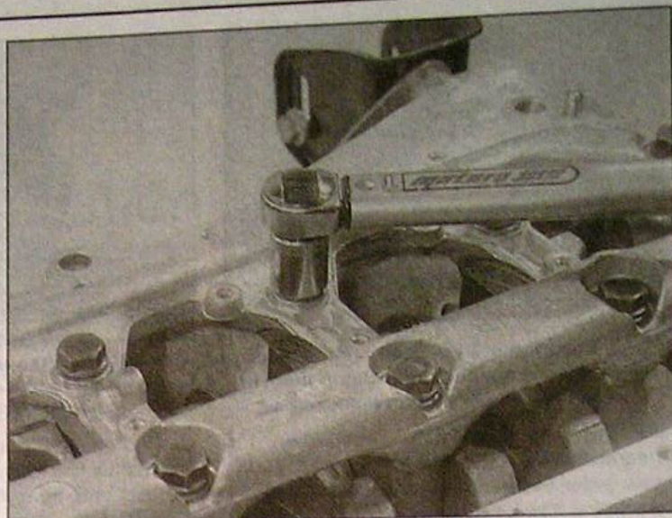
18.35b ... tighten the main bearing cap bolts to the Stage 1 torque setting ...
