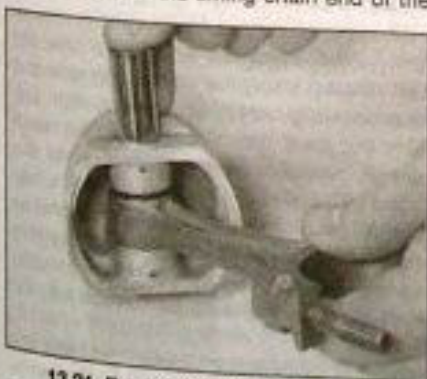
13.21 Ensure that the piston and connecting rod are correctly mated, then press the gudgeon pin into position ...
