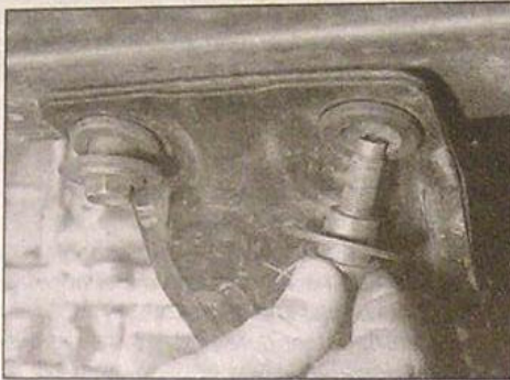
4.22a Undo the four bolts and washers . . .
