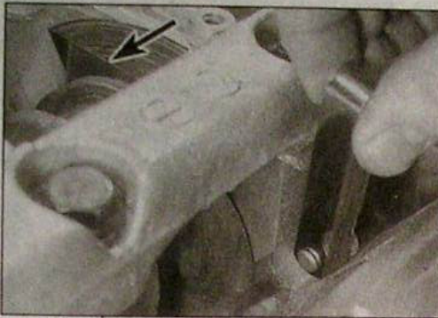
14.3 Using a feeler blade (arrowed) to measure crankshaft endfloat
