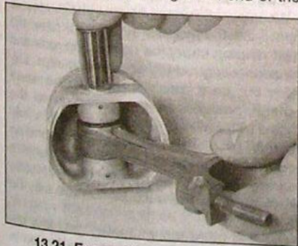
13.21 Ensure that the piston and connecting rod are correctly mated, then press the gudgeon pin into position...
