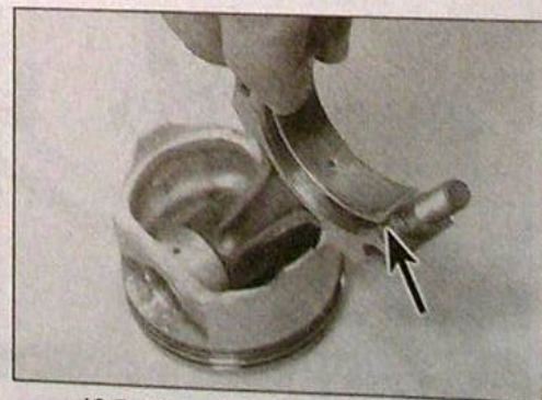
19.5 Fit each bearing shell to its connecting rod, aligning its tab with the rod cut-out (arrowed)
