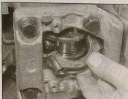
10.5 Removing a big-end cap and shell (2.0 litre engine shown)
