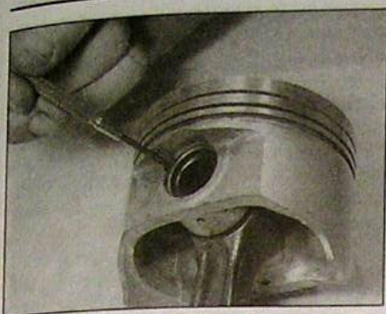
13.14 Prise out the circlips, then press the gudgeon pin out of the piston
