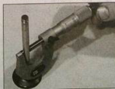
8.11 Measuring a valve stem diameter
