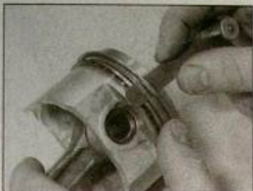
13.2 Using a feeler blade to ease piston ring removal
