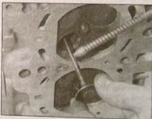
9.2 Lubricate the valve stem, and slide the valve into its respective guide
