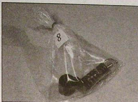
7.8 Place each valve and its associated components in a labelled polythene bag
