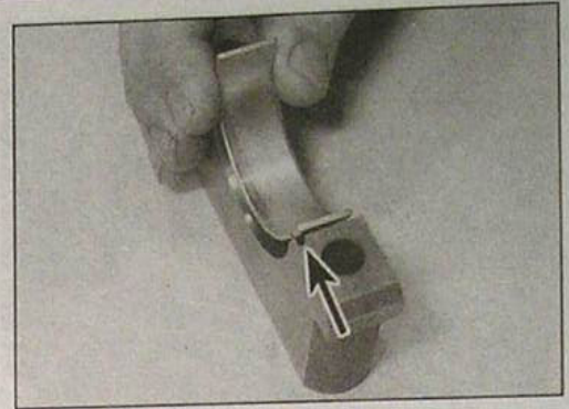
18.6b . . . and fit the lower plain shells to the caps, also aligning their tabs with the cap cut-outs (arrowed)
