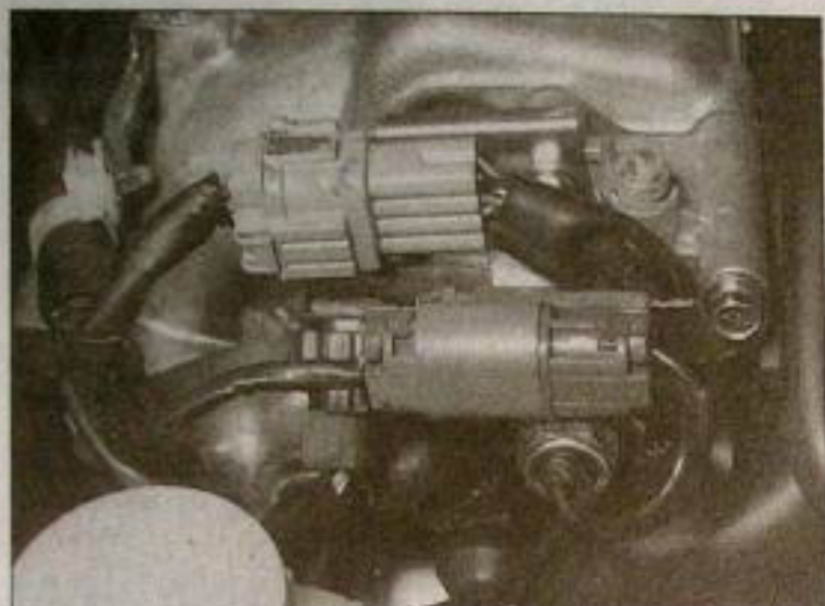
4.13a Disconnect all the relevant fuel system wiring, and free it from the inlet manifold (2.0 litre Phase II model shown)
