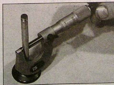
8.11 Measuring a valve stem diameter
