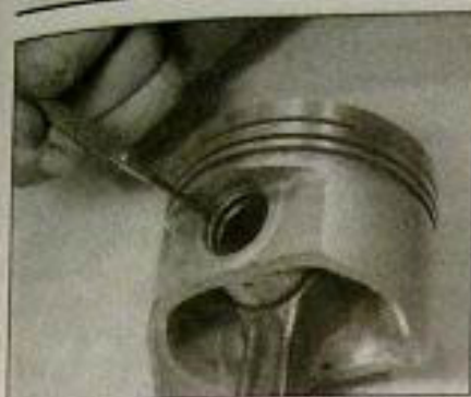
13.14 Prise out the circlips, then press the gudgeon pin out of the piston
