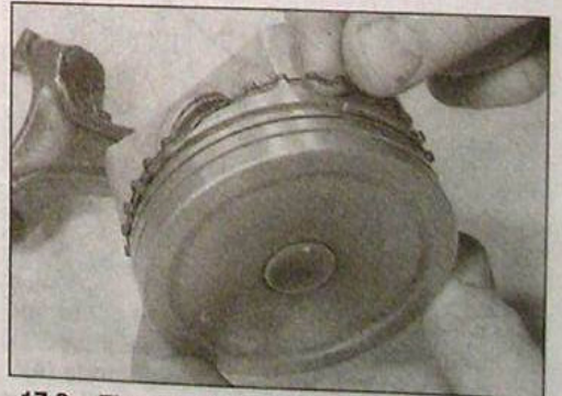
17.9a Fit the oil control ring expander...
