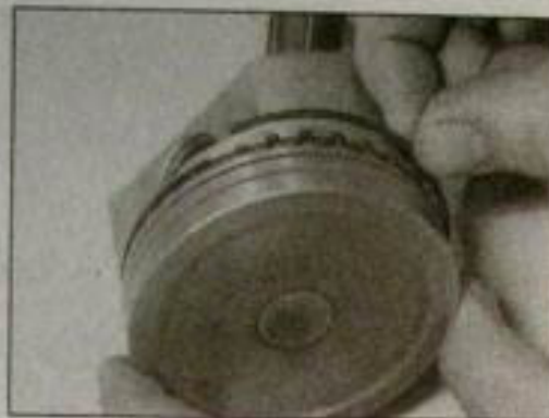
17.9b ... then install the side rails as described in text
