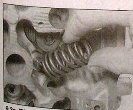
9.3a Fit the spring with its closer-pitched coils at the bottom ...
