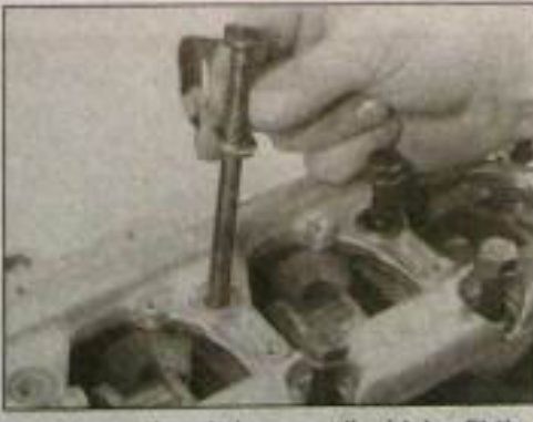
18.34b ... then (where applicable) refit the main bearing ladder, and install the retaining bolts and washers
