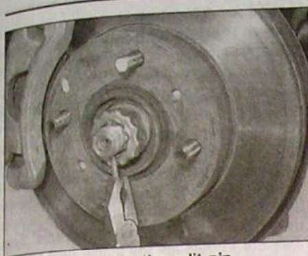
2.3a Remove the split-pin ...
