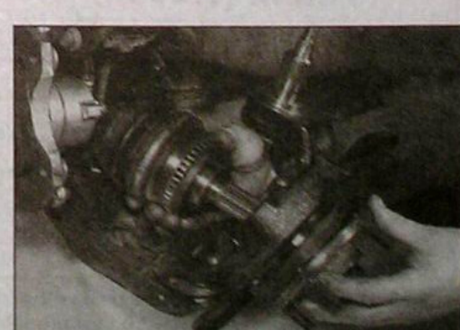
2.9 Withdraw the driveshaft from the hub carrier
