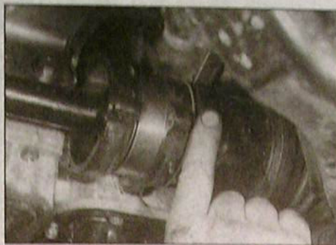
2.14 Separate the bearing housing from the bracket - 2.0 litre models
