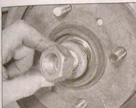
2.4 Removing the driveshaft nut
