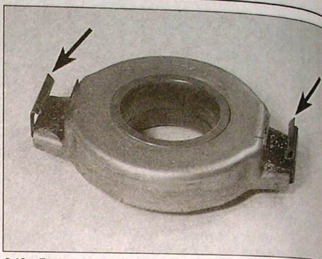
6.12a Ensure that the retaining clips (arrowed) are correctly fitted to the release bearing . . .
