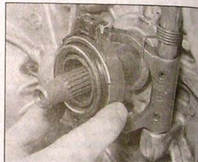
6.12b . . . then fit the bearing to the transmission, making sure the clips are correctly engaged with the release fork ends
