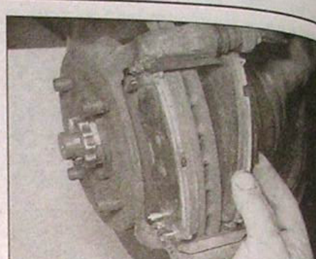
4.24c ... and inboard pads - Bendix caliper
