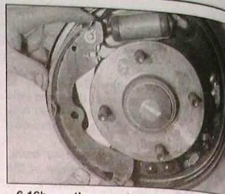
6.16b ... then manipulate the shoe into position ...
