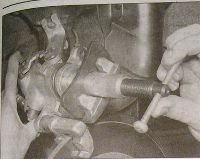
5.10a Using a retractor tool to retract a rear caliper piston
