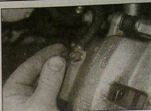
2.14b Removing the dust cap from a front caliper bleed screw
