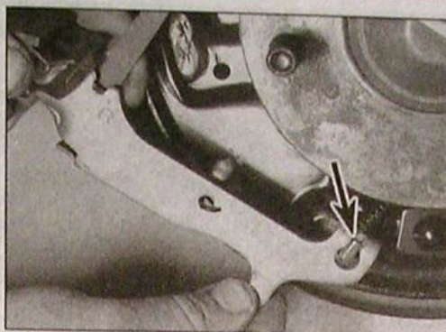
6.16a Engage the handbrake cable (arrowed) with the operating lever ...
