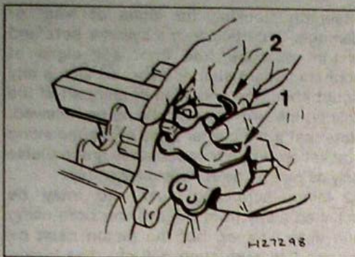
10.27 Fit the handbrake lever return spring in the order shown
