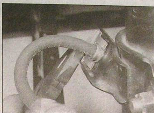
3.2b Removing a front brake hose-to-bracket securing clip
