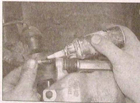
4.13b Apply locking fluid to the threads of the caliper guide pin bolts - Girling caliper
