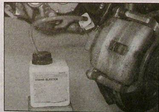
2.22 One-way valve brake bleeding kit connected to a front caliper
