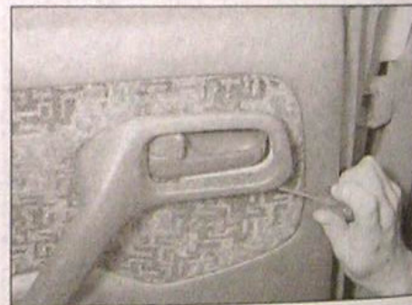
12.20a On the rear door, prise the upper part of the interior door handle surround from the door panel ...
