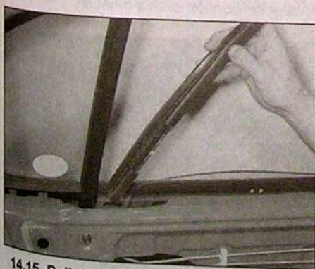
14.15 Pull the weatherstrip from the top rear corner of the window aperture and pull it up and out of the rear guide channel
