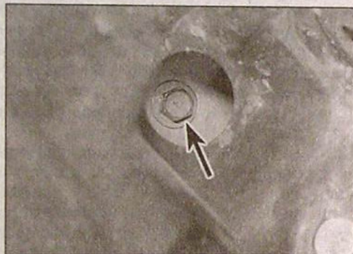
6.4b ... and rear bumper lower securing bolts (arrowed) - Hatchback model
