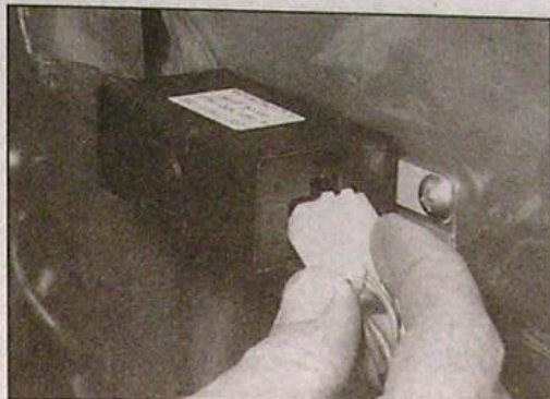
21.4 Disconnecting the wiring plug from the electric window electronic control unit
