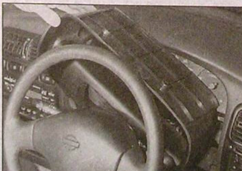
30.31 ... then withdraw the instrument panel shroud
