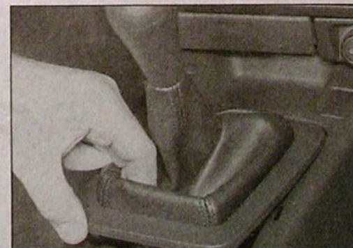
29.5 Unclip the gear lever gaiter from the centre console
