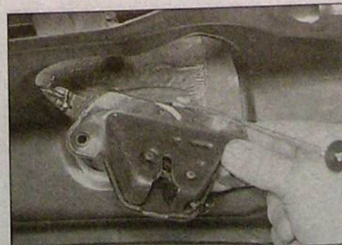
18.6 Manipulate the lock out through the tailgate aperture - Hatchback model
