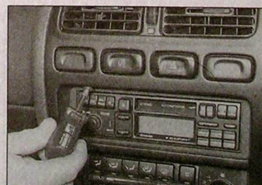
30.15a Remove the two upper ...
