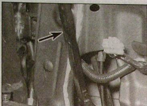
14.14b ... and withdraw the window front guide channel (arrowed) - Saloon and Hatchback models
