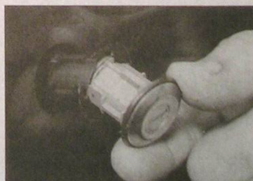
13.27b ... then withdraw the lock cylinder from outside the door
