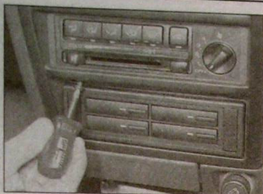
30.15b ... and the two lower securing screws ...
