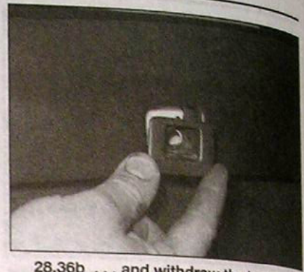
28.36b . . . and withdraw the luggage cover supports
