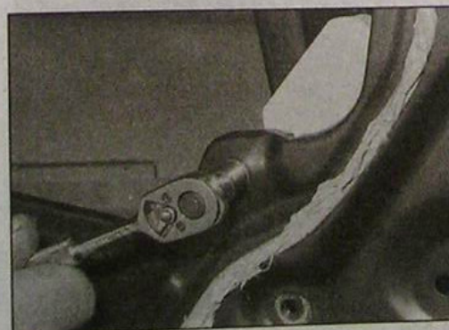
13.38 Remove the bolt securing the lock motor to the door panel
