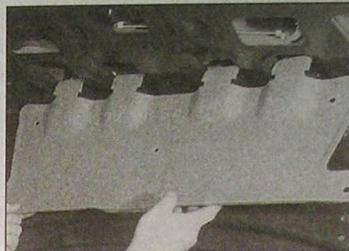
17.1b ... and withdraw the boot lid trim panel - Saloon model
