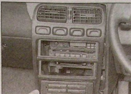
30.15c ... then pull the facia centre switch/ventilation nozzle housing from the facia
