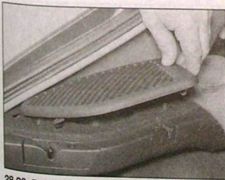
28.28 Pull out the loudspeaker cover panel - Hatchback model
