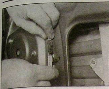
14.33 Separate the two halves of the regulator motor wiring connector - Saloon and Hatchback models
