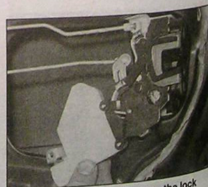
13.39b ... and withdraw the lock assembly
