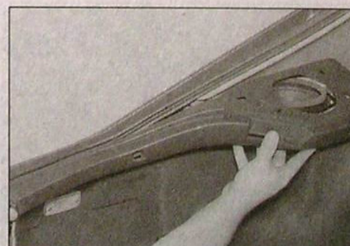
28.29b . . . then pull the panel from the body - Hatchback model
