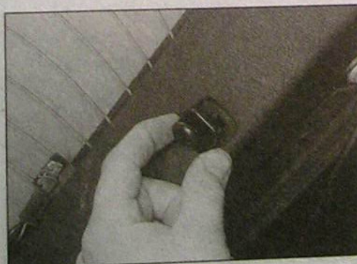
28.46b . . . then pull out the parcel shelf support cord anchors
