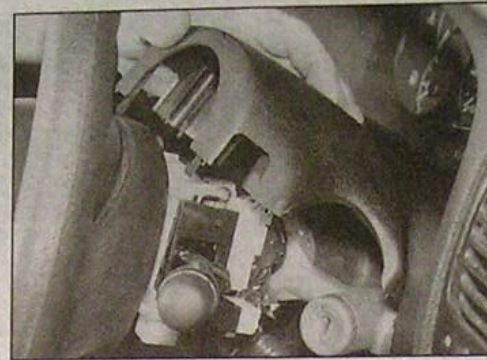
30.26 Removing the upper steering column shroud
