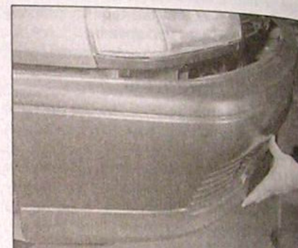
6.7 Withdrawing the front bumper from the vehicle - Hatchback model
