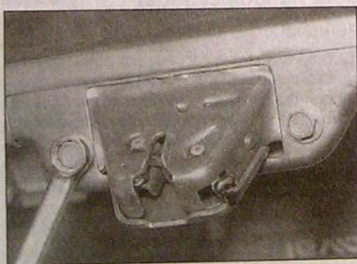
18.3 Unscrew the lock securing bolts - Hatchback model
