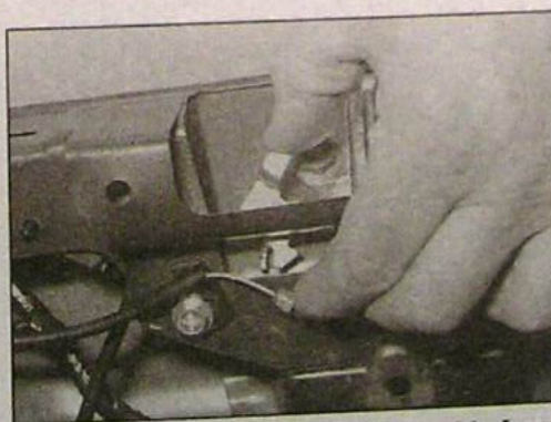
19.1 Disconnecting the release cable from the tailgate lock striker - Hatchback model
