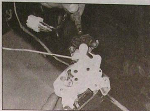
13.33b Withdraw the lock, and disconnect the central locking motor/switch wiring plug
