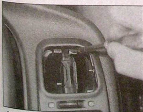
30.11a ... release the securing clips ...
