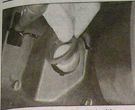
30.25b ... then unclip the ignition switch/steering column lock trim plate
