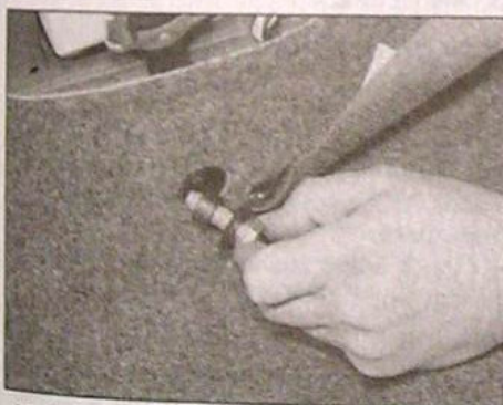
27.3 Unscrew the seat belt lower anchor bolt
