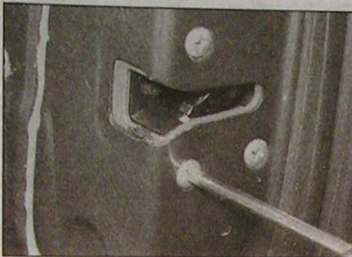
13.33a Unscrew the three lock securing bolts
