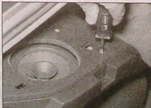
28.29a Unscrew the two side/parcel shelf trim panel securing screws . . .
