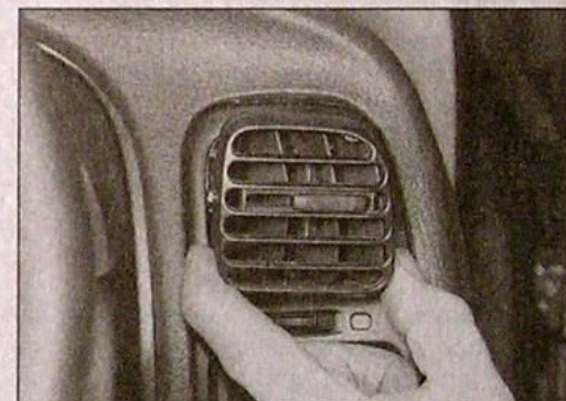
30.10 ... then prise out the ventilation nozzle ...
