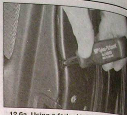
12.6a Using a forked tool to release the door trim panel securing clips
