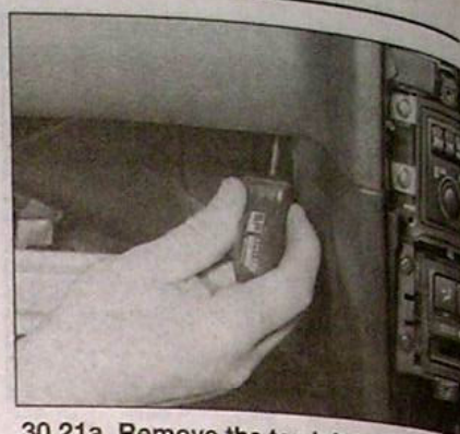
30.21a Remove the top left-hand securing screw ...
