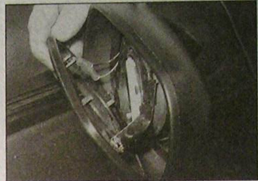
22.9b ... and lever the glass forwards to release the securing clips
