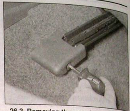
26.3 Removing the securing screw from the front seat inner rail rear trim cover
