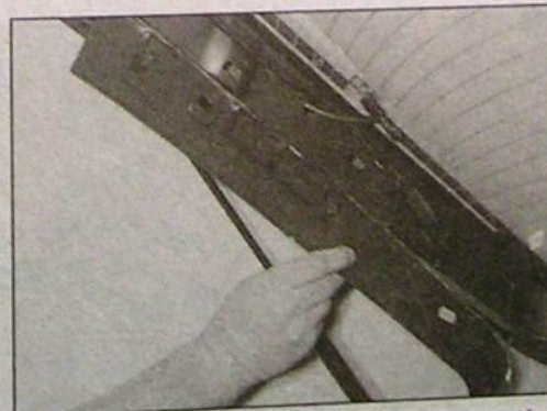
28.46c . . . and pull the trim panel from the tailgate - Hatchback model
