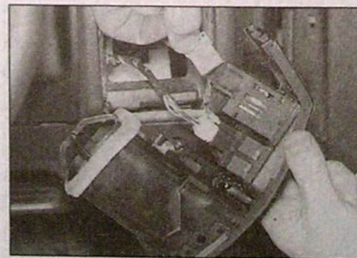
30.11b ... and pull the driver's side switch/ventilation panel from the facia
