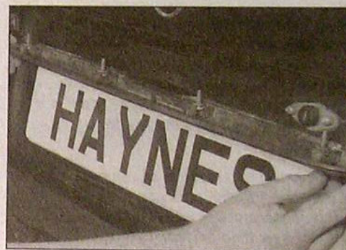
18.15b ... and withdraw the trim panel/handle - Hatchback model
