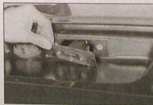
7.40 Undo the two screws and withdraw the number plate light from the tailgate - Estate models
