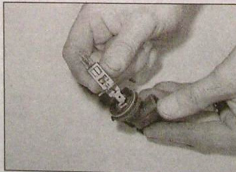
5.24 . . . and withdraw the push-fit foglight bulb
