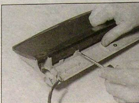
5.51b ... and lower screws to remove the LED pack from the stoplight body
