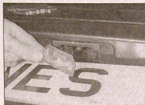
5.40b ... and lift off the number plate light lens
