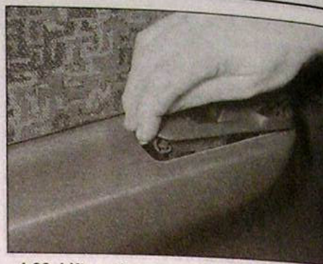
4.26 Lift up the passenger's door switch panel ...
