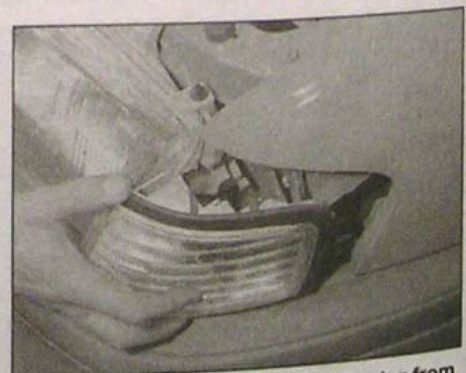
7.9 Withdraw the direction indicator from the headlight and front wing
