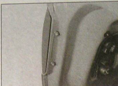
7.23 Reversing light and rear foglight outer edge retaining nuts
