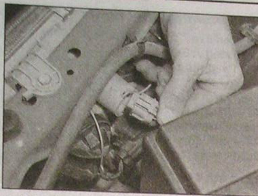
7.2a Disconnect the headlight wiring plug ...
