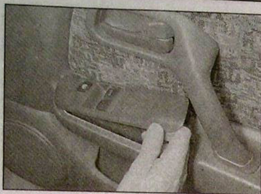
4.22a Lift up the switch panel in the driver's door ...
