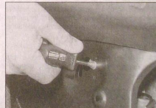
21.6 Remove the screw securing the earth lead to the body
