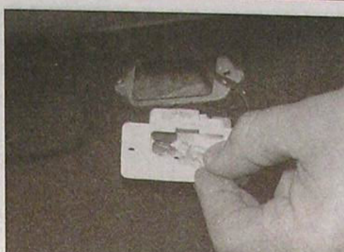
6.13 Removing the luggage compartment light bulb - Hatchback model
