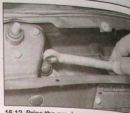
16.12 Prise the crank arm from the spindle unit
