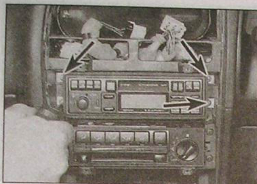
19.3 Remove the radio/cassette player securing screws (arrowed) . . .
