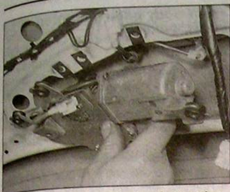
17.15 Lifting out the tailgate wiper motor - Estate model
