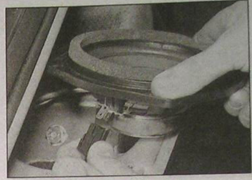
20.16b . . . then lift out the rear loudspeaker and disconnect the wiring plug - Hatchback model
