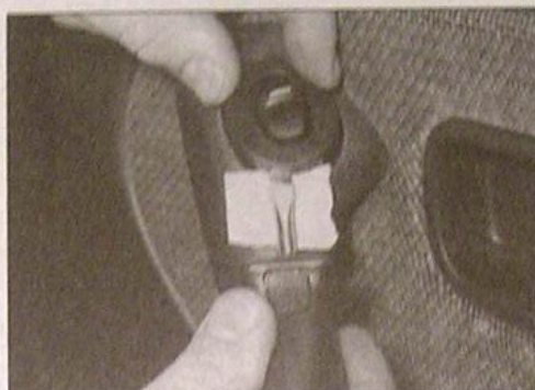
4.21 Prising an electric window switch from the front door. Note card used to protect door trim
