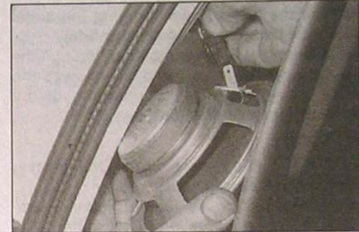
20.23b . . . then withdraw the rear loudspeaker and disconnect the wiring plug - Estate model
