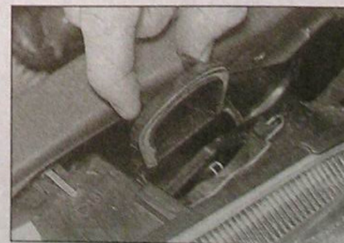
5.40 Remove the plastic cover from the light unit . . .
