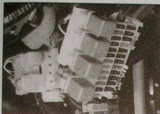
3.13e Driver's side lower facia panel removed to expose relays next to fusebox
