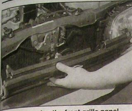
7.2 Removing the front grille panel
