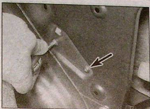
21.9 Unscrew the two screws securing the aerial to the body
