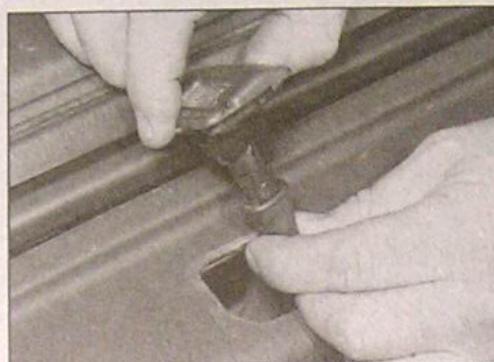
5.74 Pulling the rubber cover from the rear number plate light - Hatchback model
