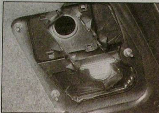
7.20 Rear stop/tail/direction indicator light unit securing nuts - Saloon model
