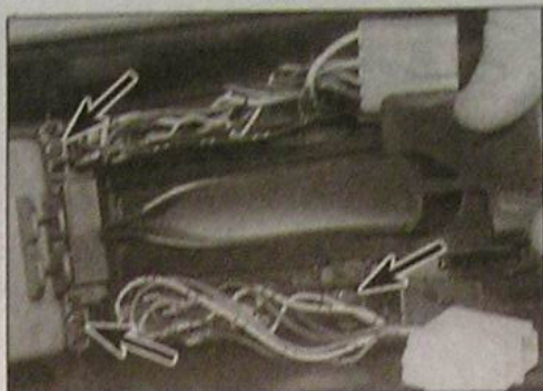
4.18a Remove the securing screws (two for each switch - arrowed) . . .
