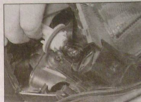
5.27 Withdrawing the bulbholder from the direction indicator light unit - Saloon and Hatchback models
