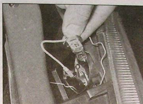
5.41b ... and remove the bulb from the driving light - Saloon and Hatchback models
