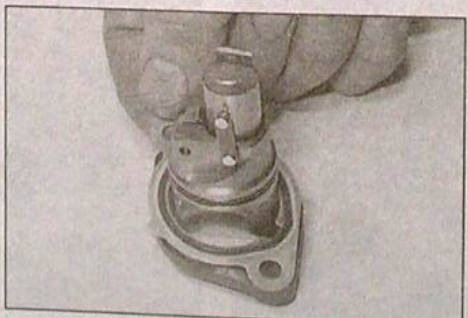
7.26b Fit a new O-ring and gasket to the tensioner, making sure that the gasket is fitted the correct way round
