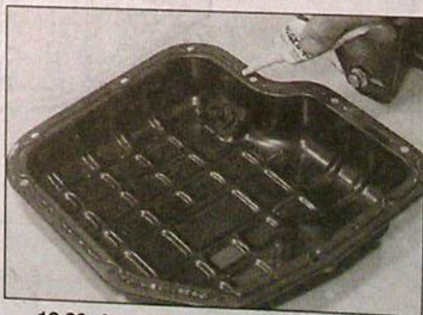
12.30 Apply a bead of sealant to the pressed-steel sump flange ...
