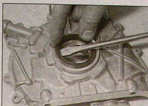
6.14a Lever out the crankshaft oil seal with a large flat-bladed screwdriver ...
