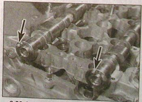
9.20 Lay the camshafts in the cylinder head, positioning the locating pins (arrowed) as shown
