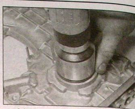
6.14b ... and tap the new one into position using a suitable socket
