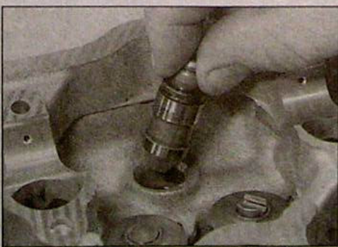
10.3b ... and remove the hydraulic adjuster from the cylinder head
