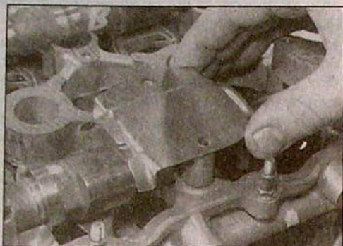
9.23a Fit the baffle plate to No 2 exhaust camshaft bearing cap ...
