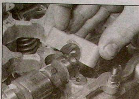
9.22 Fit the bearing caps, using the marks made prior to removal to ensure that each is correctly positioned
