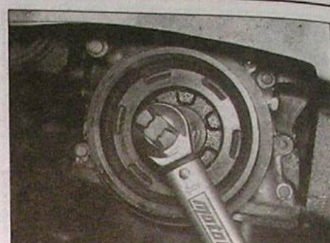
5.7 Refit the retaining bolt (and washer) and tighten to the specified torque
