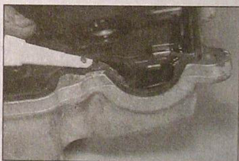
4.9 Apply a bead of sealant to the seal on 1 cm either side of the exhaust camshaft bearing cap cut-out
