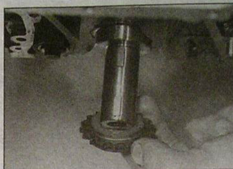
7.19 . . . and slide on the crankshaft sprocket
