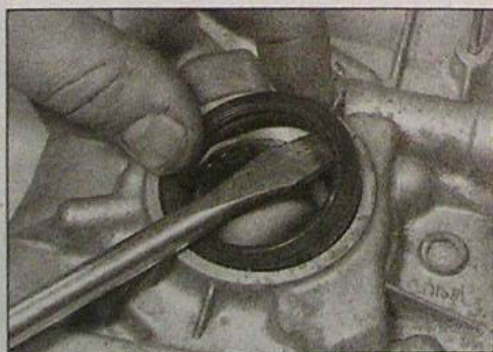
6.14a Lever out the crankshaft oil seal with a large screwdriver ...
