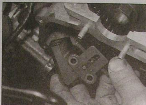
7.4b ... then retract the tensioner as described in the text and remove it from the head
