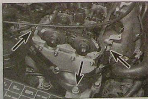
6.5a Undo the three retaining bolts (arrowed) and remove the bracket from the engine mounting
