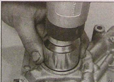
6.14b ... and tap the new seal into position with a suitable socket
