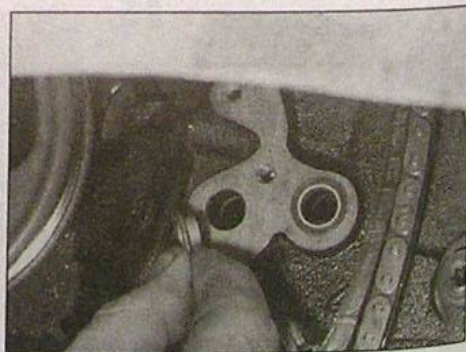
6.16 Fit the new special sealing collars to the cylinder block oil galleries
