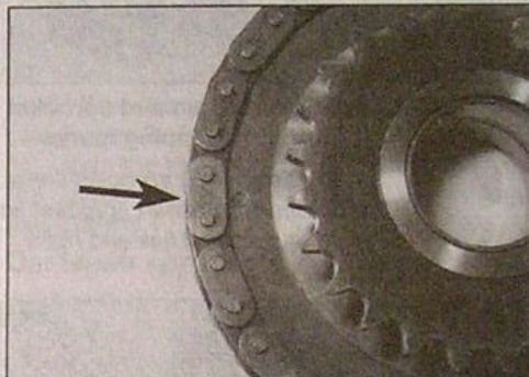
7.20b . . . then engage the sprocket with the timing chain, aligning its timing mark with one of the chain's coloured links (arrowed)
