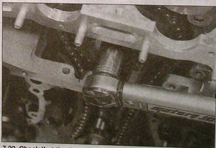
7.22 Check that the timing marks are correctly positioned then fit the idler sprocket bolt and washer, and tighten it to the specified torque
