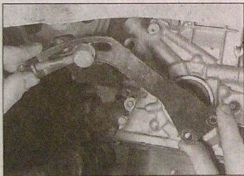
6.4 Removing the power steering pump mounting bracket
