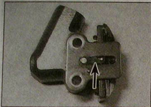
8.25 On early models, prior to refitting retract the plunger and secure it in position with the hook (arrowed)
