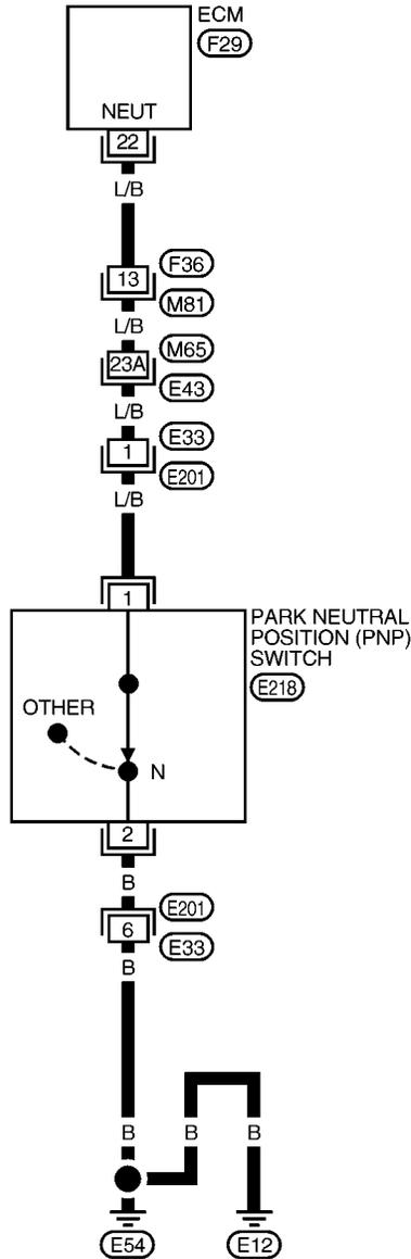
: Detectable line for DTC
