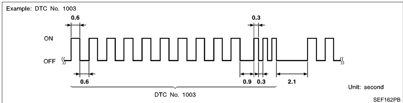
Long (0.6 second) blinking indicates the two LH digits of number and short (0.3 second) blinking indicates the two RH digits of number. For example, the MIL blinks 10 times for 6 seconds (0.6 sec x 10 times) and then it blinks three times for about 1 second (0.3 sec x 3 times). This indicates the DTC "1003" and refers to the malfunction of the park/neutral position (PNP) switch.
