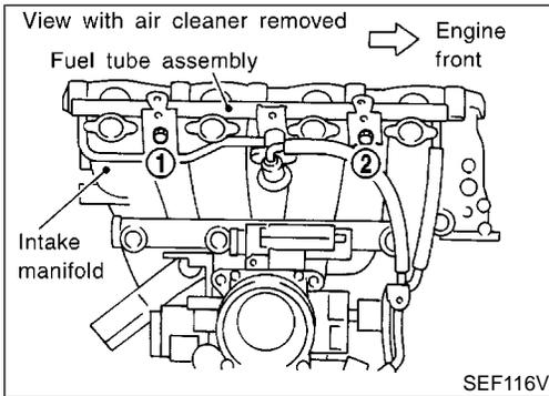
5. Install injectors with fuel tube assembly to intake manifold. **Tighten in numerical order shown in the figure.**
