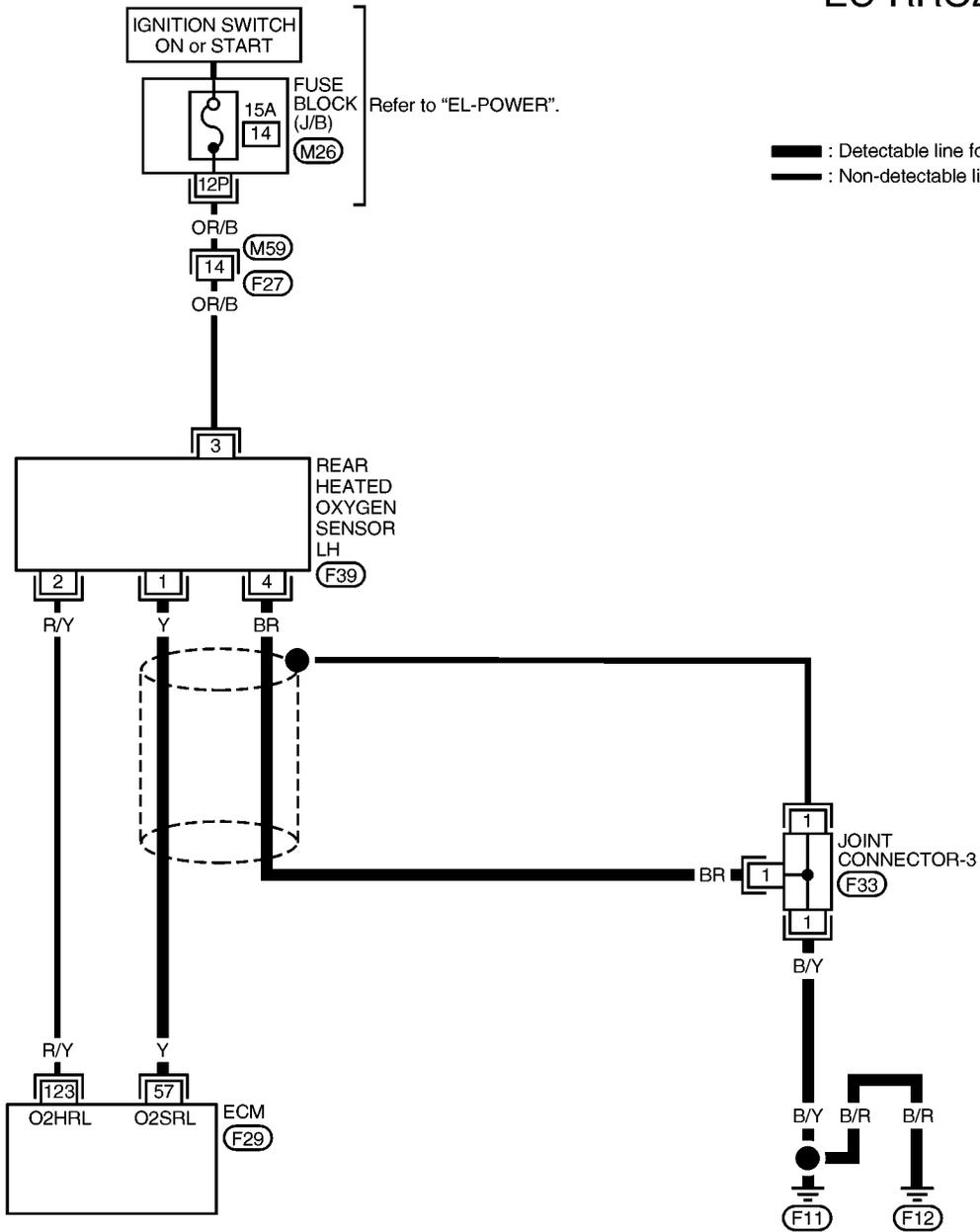
— : Detectable line for DTC
