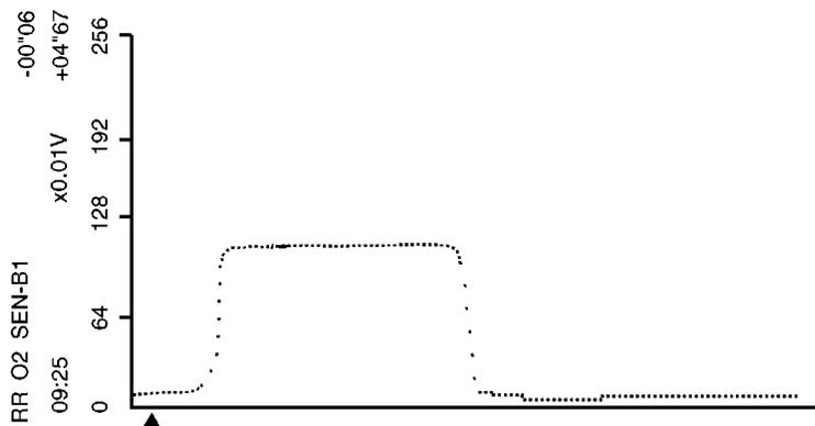
•“RR O2 SEN-B1” may increase immediately after depressing the accelerator pedel and may decrease after releasing the pedal.
