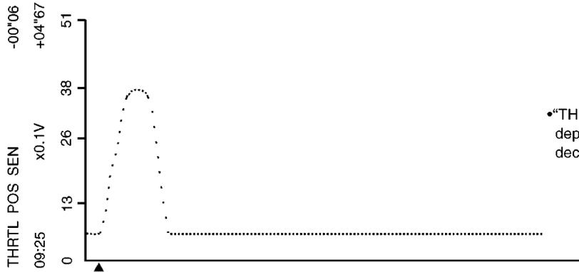
•“THRTL POS SEN” should increase while depressing the accelerator pedel and should decrease while releasing it.
