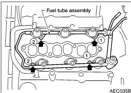
9. Install injectors with fuel tube assembly to intake manifold.
