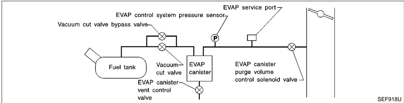
In this evaporative emission (EVAP) control system, purge flow occurs during non-closed throttle conditions. Purge volume is related to air intake volume. Under normal purge conditions (non-closed throttle), the EVAP canister purge volume control solenoid valve is open. Purge flow exposes the EVAP control system pressure sensor to intake manifold vacuum.
