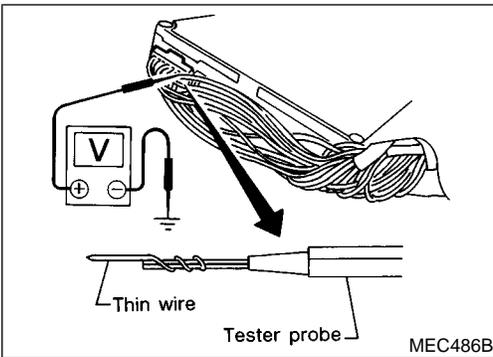
3. Perform all voltage measurements with the connector connected. Extend tester probe as shown to perform tests easily.
