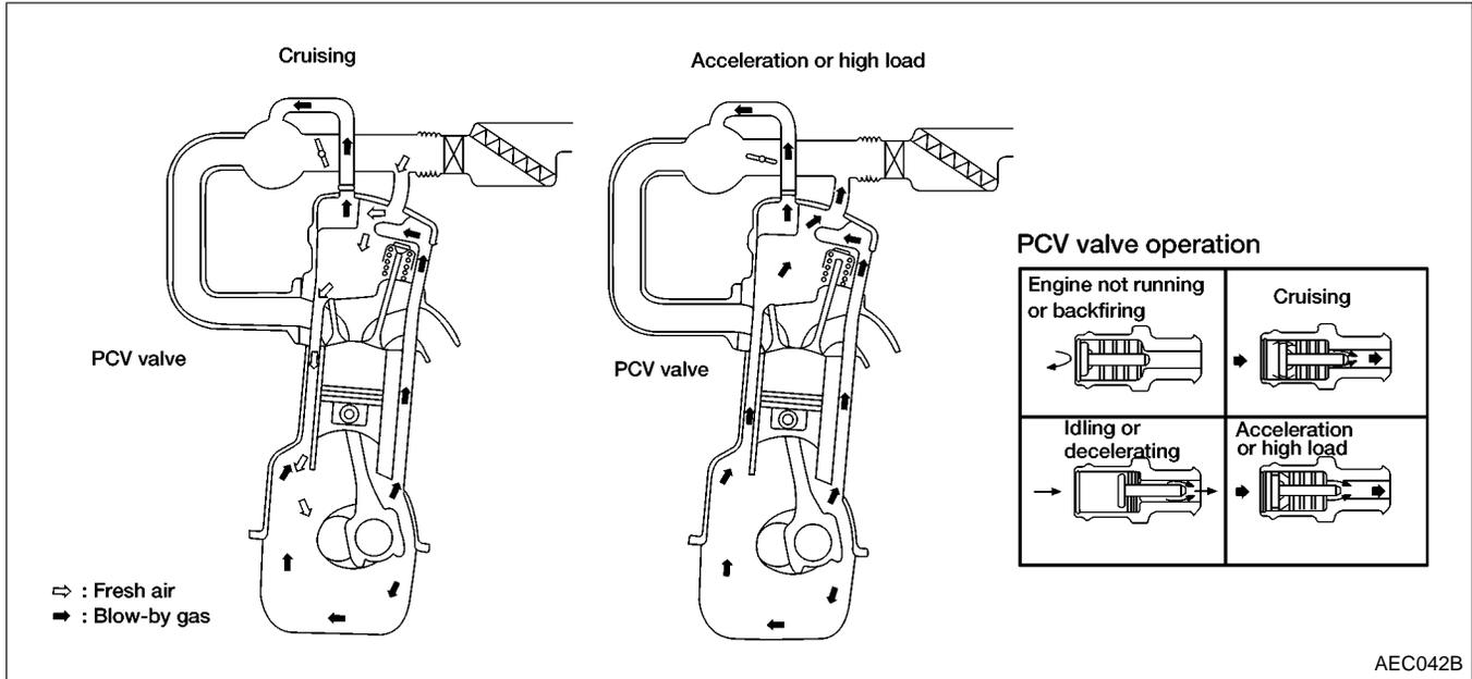
This system returns blow-by gas to the intake collector.
