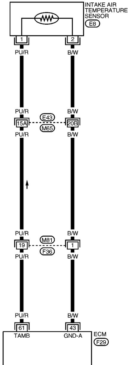
— : Detectable line for DTC
