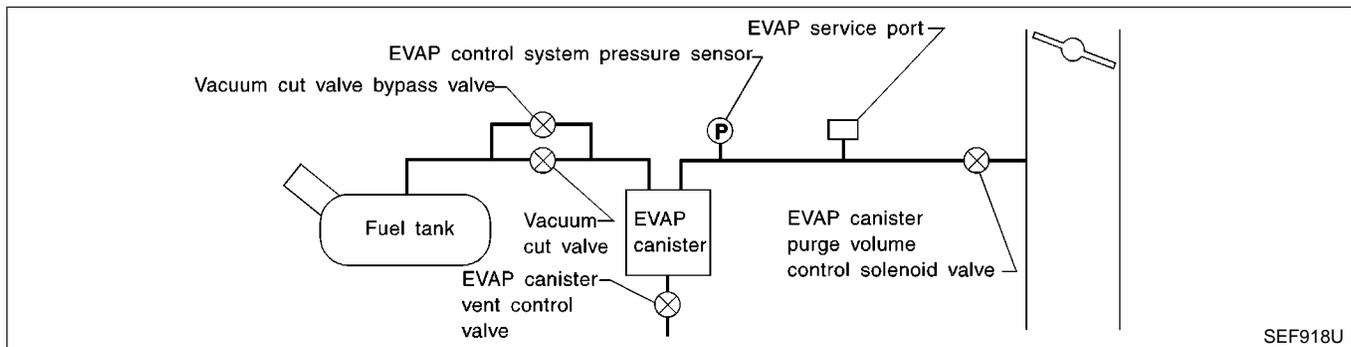
Malfunction is detected when EVAP control system has a very large leak, such as fuel filler cap fell off, EVAP control system does not operate properly.
