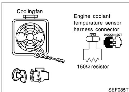
5. Connect 150Ω resistor to engine coolant temperature sensor harness connector.
