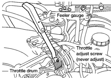
“Continuity should exist” while inserting 0.3 mm (0.012 in) feeler gauge.
