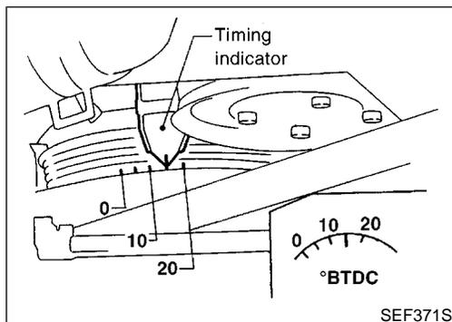
8. Check ignition timing. Refer to "Basic Inspection", EC-669. Make sure that ignition timing is  $15^\circ \pm 2^\circ$  at  $700 \pm 50$  rpm. If NG, adjust ignition timing and then recheck.
