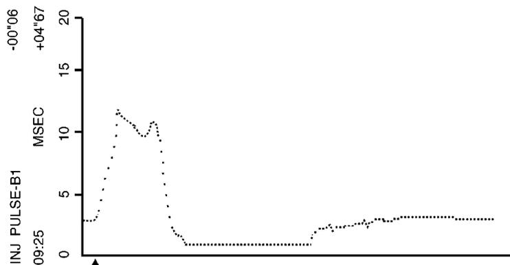
•“INJ PULSE-B1” should increase when depressing the accelerator pedal and should decrease when the pedal is released.
