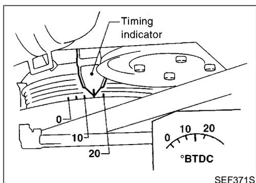
10. Check ignition timing. Refer to "Basic Inspection", EC-669. Make sure that ignition timing is  $15^\circ \pm 2^\circ$  at  $700 \pm 50$  rpm. If NG, adjust ignition timing and then recheck.
