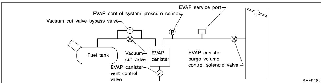
Malfunction is detected when EVAP control system has a leak, EVAP control system does not operate properly.
