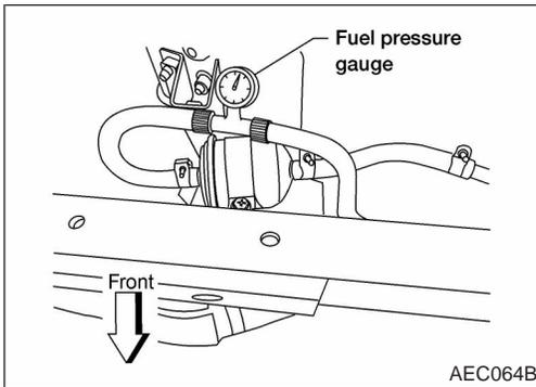
3. Install pressure gauge between fuel filter and fuel tube.
