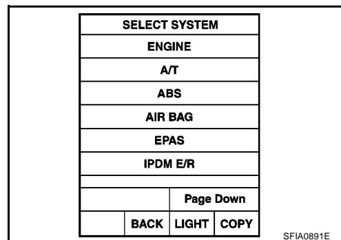
5. Select desired part to be diagnosed on "SELECT DIAG MODE" screen.
