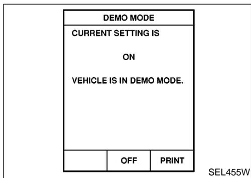
3. Touch “ON”. Now, the system is in demonstration mode. (To return to normal mode, touch “OFF”.)
