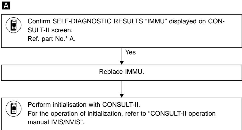
\* Ref. part No.: reference part No. of Diagnostic System Diagram on EL-449.
