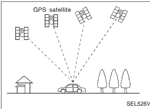
GPS is the global positioning system developed and operated by the US Department of Defense. GPS satellites (NAVSTAR) transmit radio waves and orbit around the earth at an altitude of approximately 21,000 km (13,000 miles).
