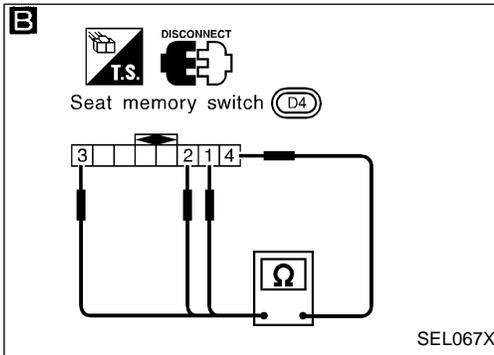
**CHECK SEAT MEMORY SWITCH INPUT SIGNAL.**
