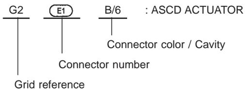
The following Harness Layouts use a map style grid to help locate connectors on the drawings:
