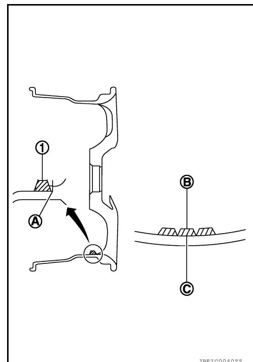
4. If calculated balance weight value exceeds 50 g (1.76 oz), install two balance weight sheets in line with each other as shown.
