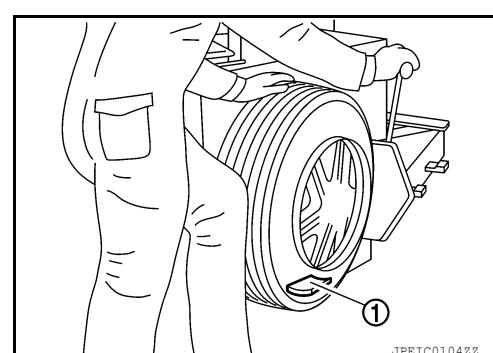
5. Lubricate the tire inside bead well with a suitable non-silicone lubricant, and remove inside of tire from the wheel.
