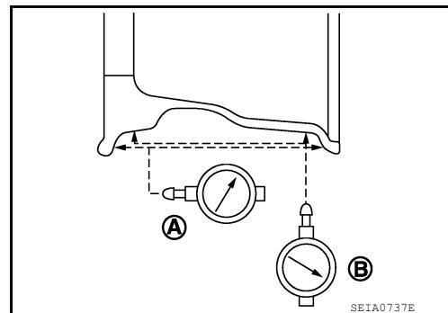
**Axial Runout (A)** : Refer to [WT-76, "Wheel"](#).
