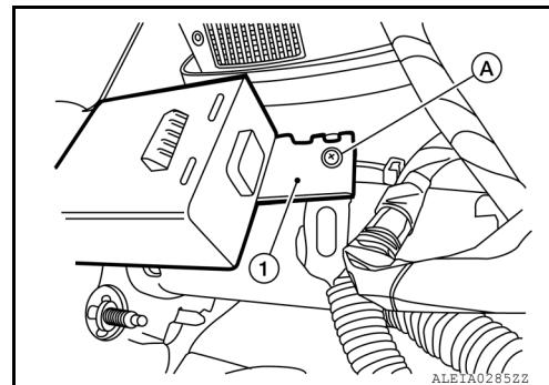
5. Remove low tire pressure warning control unit.
