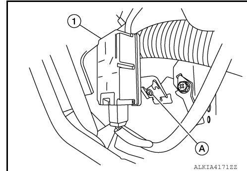
4. Remove remote keyless entry receiver from bracket.
