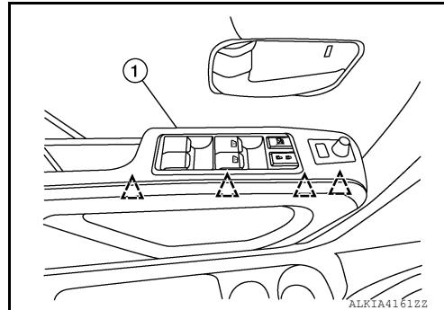
2. Disconnect the harness connector (1) from the main power window and door lock/unlock switch.
