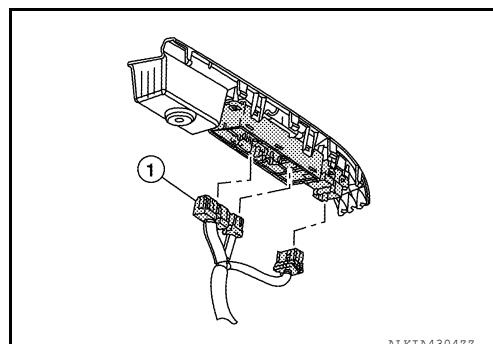
3. Release the main power window and door lock/unlock switch finisher pawls from the main power window and door lock/unlock switch (1) using suitable tool.
