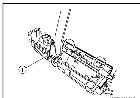
4. Remove the main power window and door lock/unlock switch (1).
