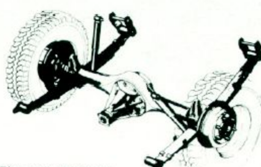
Bias-mounted rear shock absorbers reduce axle wind-up; leaf springs give stability.
