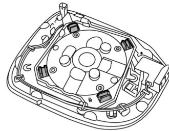
**caution** Remove the fixing pawls slowly so they are not damaged.
