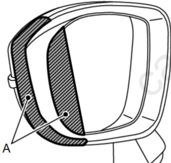
3. Insert remover tool (A) into the recess at outside between glass mirror and door mirror actuator, and then disengage glass mirror fixing pawls.
