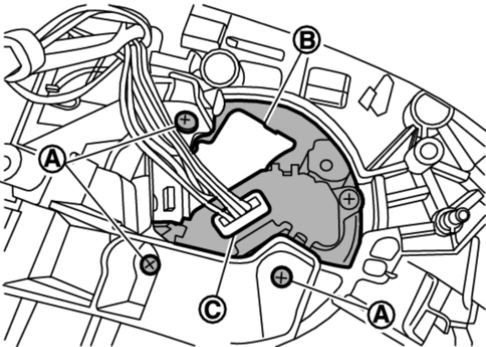
10. Disconnect harness connectors **B** and **C**, and then remove door mirror actuator.
