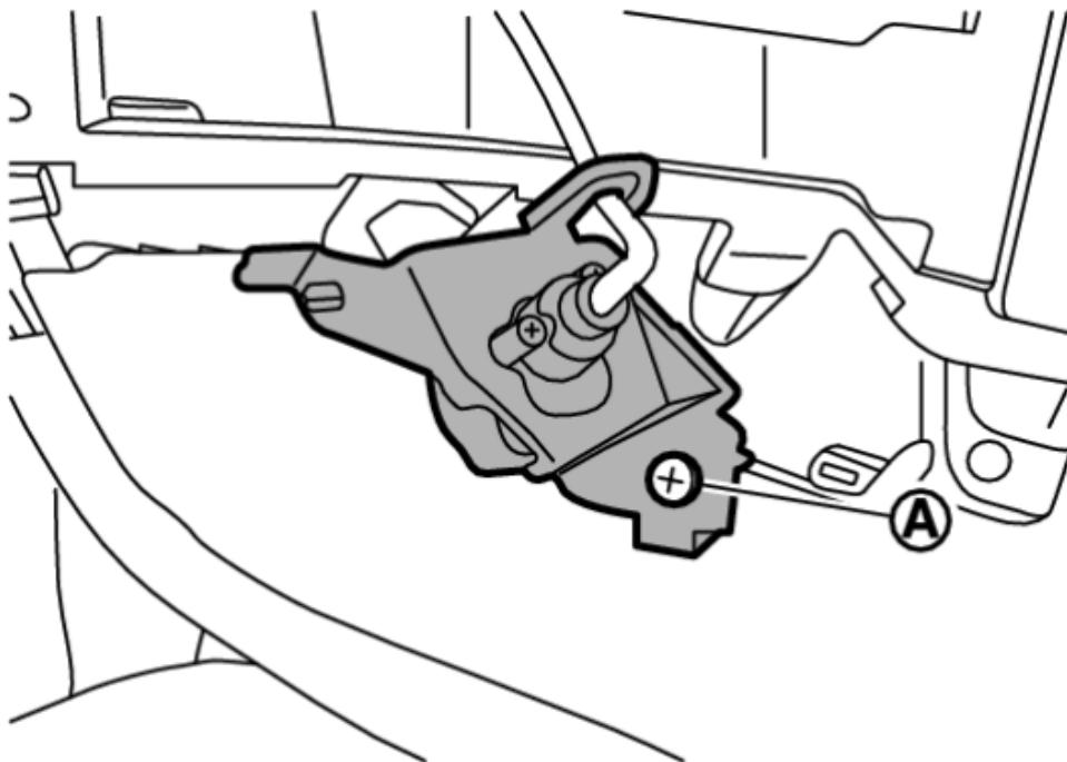
8. Remove side turn signal light (with side turn signal light). Refer to [Removal and Installation](#)
