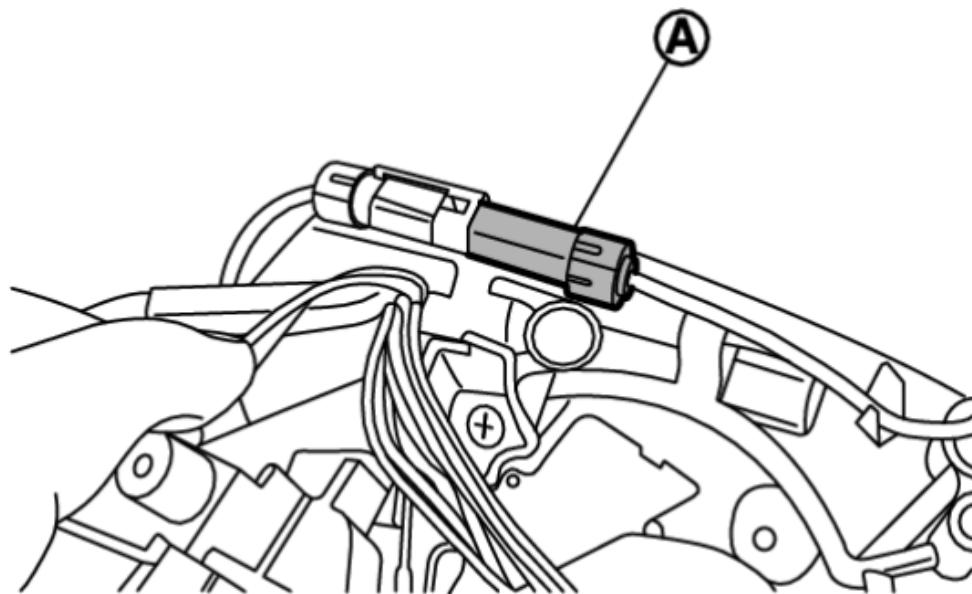
7. Remove side camera fixing screw Ⓐ, and then remove side camera (with side camera).
