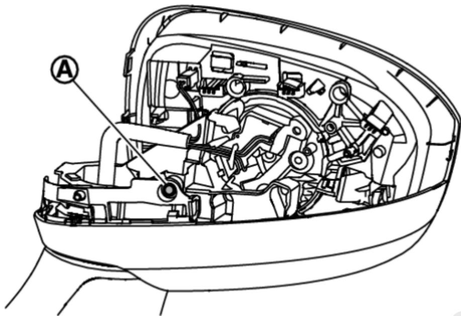
5. Disengage door mirror finisher fixing pawls, and then remove door mirror finisher.
