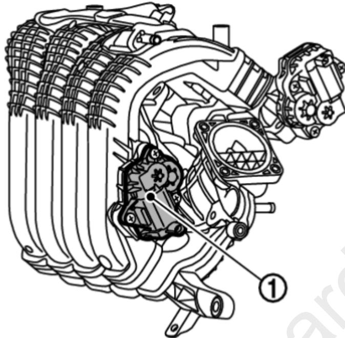
Intake manifold tuning valve consists of valve and motor.
