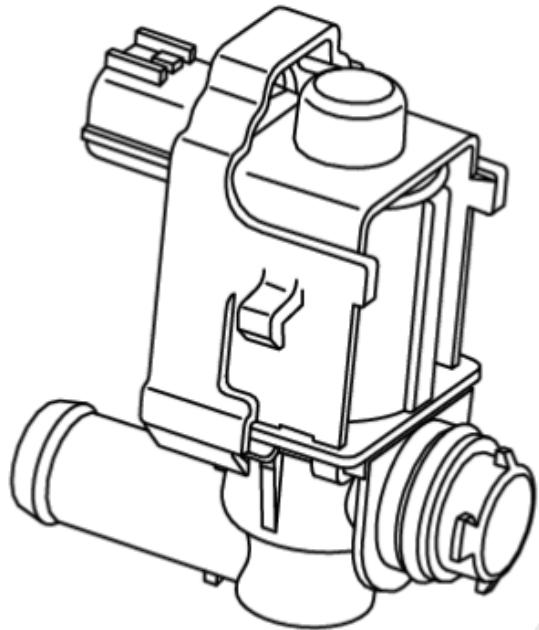
This solenoid valve responds to signals from the ECM. When the ECM sends an ON signal, the coil in the solenoid valve is energized. A plunger will then move to seal the canister vent. The ability to seal the vent is necessary for the on board diagnosis of other evaporative emission control system components.
