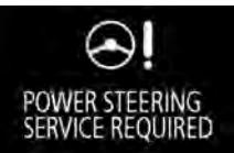
POWER STEERING<br>SERVICE REQUIRED              | ● There is a fault in the EPS.                                                                                                                                                                  | ● Have the vehicle inspected by a MITSUBISHI MOTORS Authorised Service Point as soon as possible.<br>Refer to "Electric power steering system (EPS)" on page 7-32.             |
