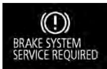
When the operation mode of the power switch is put in ON, if the brake fluid is low, this warning is displayed.
