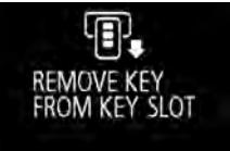
REMOVE KEY<br>FROM KEY SLOT                     | ● You have forgotten to remove the keyless operation key from the key slot.                                                                                                                     | ● Remove the keyless operation key from the key slot.<br>Refer to "Keyless operation key reminder" on page 7-13.                                                               |
