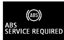
If there is a malfunction in the system, the ABS warning lamp will come on and the warning display will appear on the information screen in the multi information display. Under normal conditions, the ABS warning lamp only comes on when the operation mode is put in ON and goes off a few seconds later.
