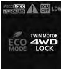
If the ECO mode switch is switched OFF, the drive mode will be returned to "4WD LOCK" mode.
