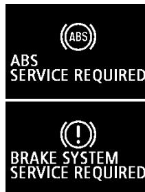
The ABS and brake force distribution function may not work, so hard braking could make the vehicle unstable.
