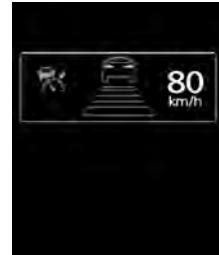
The ACC control is automatically cancelled and the ACC is placed in the ‘standby’ state in any of the situations listed below; you are alerted to this condition by the sound of a buzzer and a message on the display. You can make the system restart the control by using the “SET -” or “RES +” switch if the conditions for resuming the control are reestablished.
