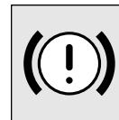
This lamp illuminates when the operation mode of the power switch is put in ON, and goes off after a few seconds.
