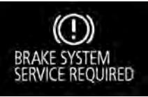
BRAKE SYSTEM<br>SERVICE REQUIRED                | ● The brake fluid level in the reservoir has fallen to a low level.<br>● There is a fault in the brake system.                                                                                  | ● Immediately stop the vehicle in a safe place.<br>We recommend you to consult a MITSUBISHI MOTORS Authorised Service Point.<br>Refer to "Brake warning display" on page 6-39. |
