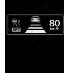
If the vehicle in front stops, the ACC reacts to it by stopping your vehicle.
