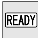
The ready indicator keeps flashing until Plug-in Hybrid EV System is activated. When the Plug-in Hybrid EV System has activated normally and the vehicle becomes ready to run, the lamp stops flashing and stays lit. Refer to "Starting the Plug-in Hybrid EV System" on page 7-12. If the indicator keeps flashing, the vehicle can not drive.
