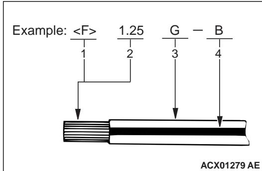
If a cable has two colours, the first of the two colour code characters indicates the basic colour (colour of the cable coating) and the second indicates the marking colour.
