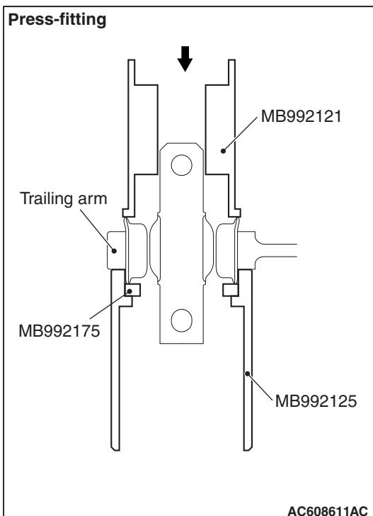
3. Use the special tools MB992121, MB992125 and MB992175 to press-fit the trailing arm bushing up to the position shown in the figure.
