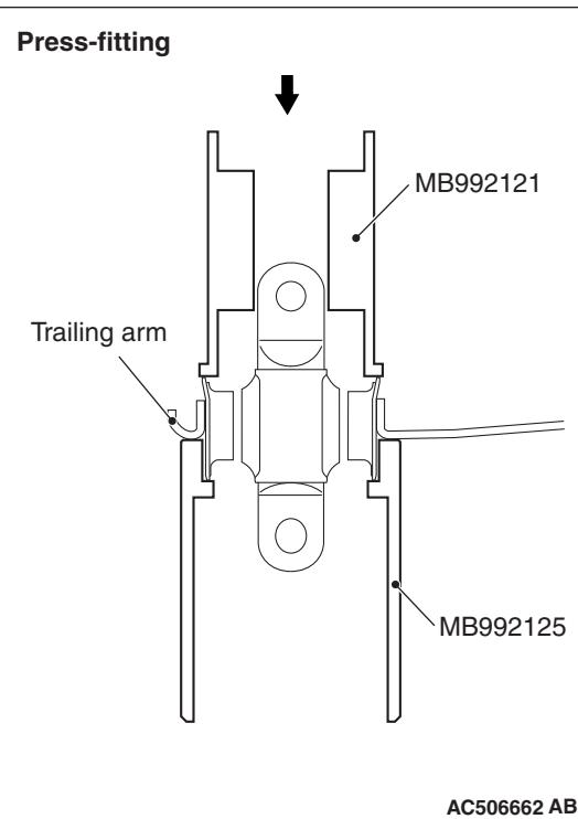
3. Use the special tools MB992121 and MB992125 to press-fit the trailing arm bushing up to the position shown in the figure:
