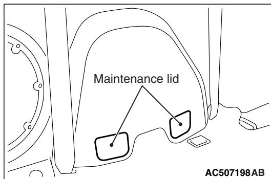
Remove the maintenance lid as shown in the figure, and then remove the shock absorber mounting nut.
