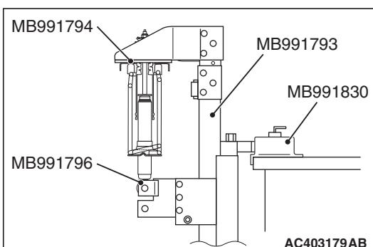
1. Install the coil spring end as shown in the figure, so that it should face the vehicle rearward.
