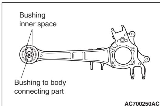
2. Determine the installation direction and the installation position of the trailing arm bushing.
