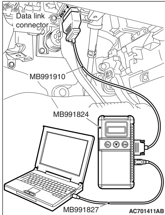
**STEP 2. Using scan tool MB991958, read the ETACS-ECU diagnostic trouble code**
