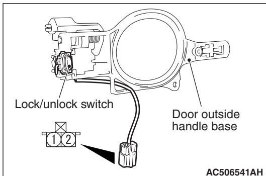
**STEP 3. lock/unlock switch (front door: LH) check.**
