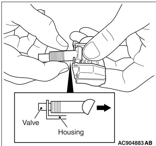
2. Clean the TPMS transmitter and the valve stem. <In case of not removing the valve>
