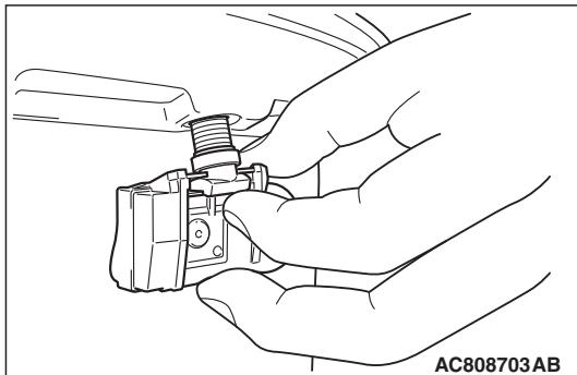
2. Insert the seal washer up to the base of the TPMS transmitter, making sure to secure the valve base with a thumb as shown.
