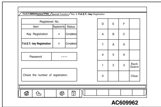
5. Check the number of the registered keys and keyless operation keys.
