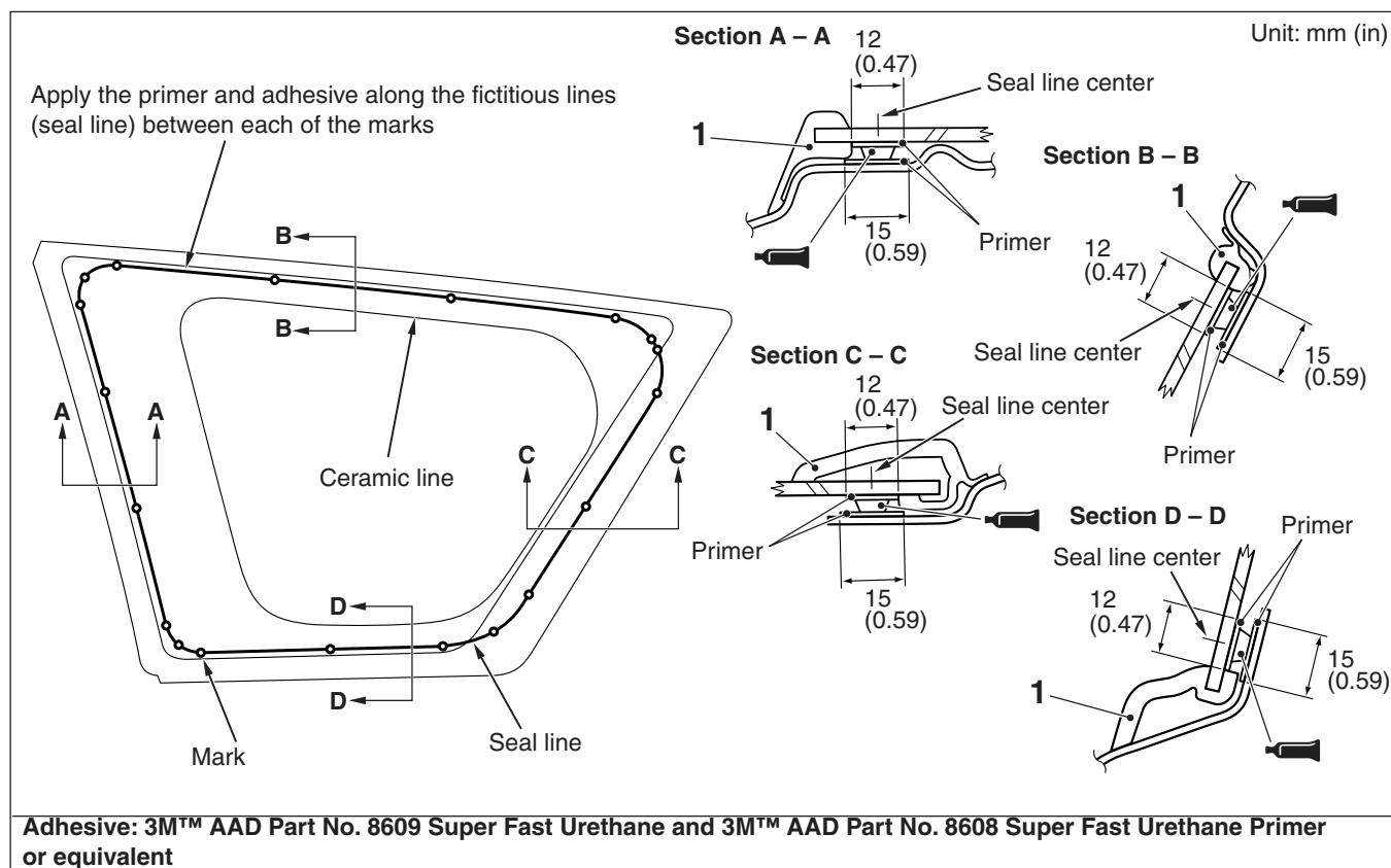
Adhesive: 3M™ AAD Part No. 8609 Super Fast Urethane and 3M™ AAD Part No. 8608 Super Fast Urethane Primer or equivalent
