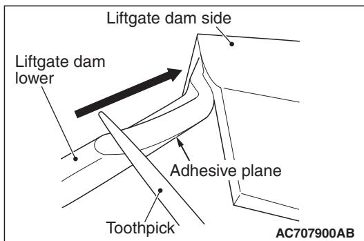
(3) After adhering the lip of the liftgate dam lower 30°-end with the lip of the liftgate dam side 62°-end, apply the adhesive to the remaining area.
