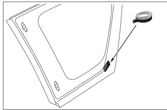
Adhesive tape: Double-sided tape [8 mm (0.31 in) width, 25 mm (0.98 in) length and 1.2 mm (0.047 in) thickness.]
