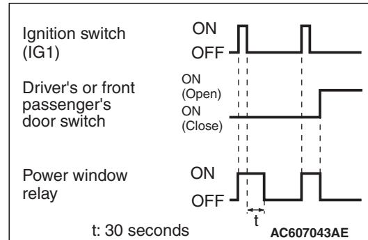
Even after the ignition is switched off, the ETACS-ECU keeps the power window relay activated for approximately 30 seconds, enabling raising or lowering of the power windows by using the power window switches (timer function). After approximately 30 seconds, the power window relay is deactivated.
