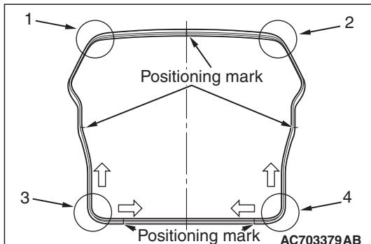
1. The marking on the upper center of the liftgate opening weatherstrip should be positioned at the center of the vehicle body.
