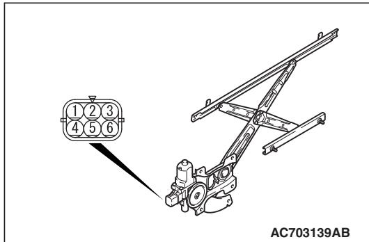
**STEP 6. Check the front power window motor (RH).**
