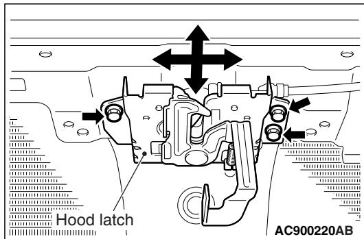
4. Loosen the hood latch mounting bolts but do not remove them. Move the hood latch up/down and left/right to align the hood level and adjust the hood striker engagement.
