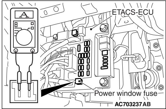
1. Remove the power window fuse to check that it is normal, and connect a multimeter as shown in the illustration.
