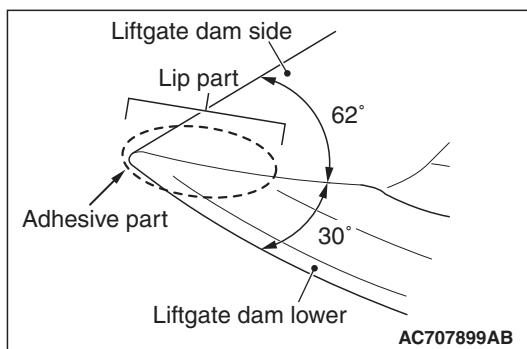
**NOTE:** When applying the adhesive to the adhesion surfaces of the liftgate dam lower center and the liftgate dam lower side (LH, RH), the task becomes easier if a tooth pick is used.
