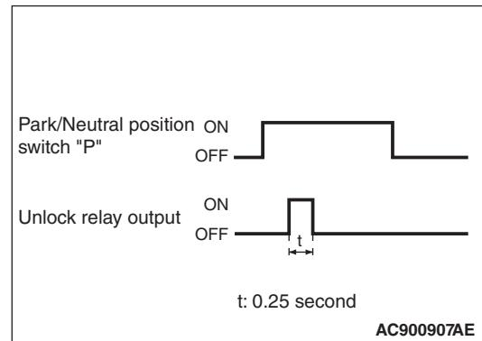
When the selector lever is shifted to the P position with the ignition switch turned ON, the transaxle range switch "P" turns ON, ETACS-ECU turns the unlock relay output ON for 0.25 seconds to unlock all the doors (including the liftgate).
