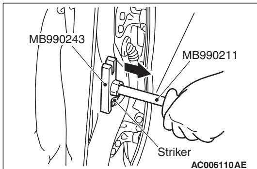
(2) Adjustment by using the striker (toward the outside of the vehicle)
