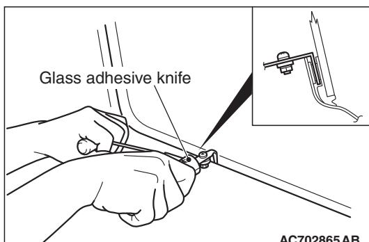
4. Working inside the vehicle, insert the tip of a windshield knife into the sealed part of the quarter window glass assembly.
