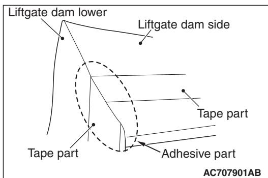
(4) Adhere the remaining area (ensure that there is no level difference at the tape part).
