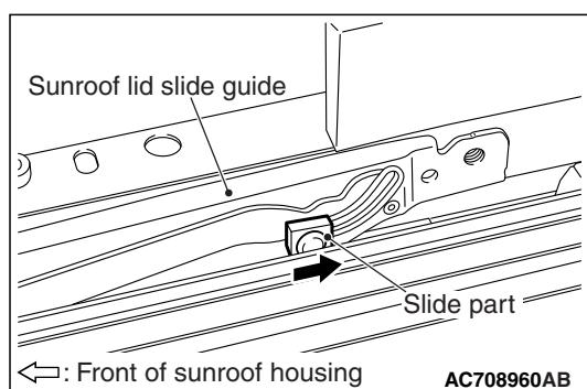
Slide the slide part of the sunroof lid slide guide to the rear of the sunroof housing, and then pull out the sunroof drip plate and sunroof lid slide guide.
