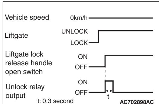
When the liftgate lock release handle is operated to open the liftgate (the liftgate lock release handle open switch turns ON) while the vehicle is parked, ETACS-ECU turns the unlock relay output ON for 0.3 second, thus the liftgate can be opened by the liftgate lock release handle.
