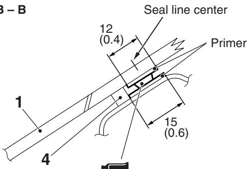
Adhesive: 3M™ AAD Part No. 8609 Super Fast Urethane and 3M™ AAD Part No. 8608 Super Fast Urethane Primer or equivalent
