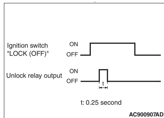
When the ignition switch is turned to the "LOCK (OFF)" position, ETACS-ECU turns the unlock relay output ON for 0.25 second to unlock all the doors.
