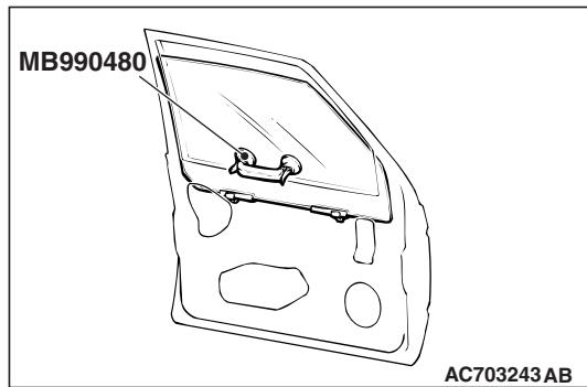
2. Lift the door window glass, and attach special tool MB990480 to the glass as shown to prevent the glass from falling.
