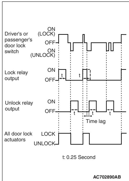
When the door is locked by the driver's or passenger's door lock switch, the ETACS-ECU operates its door lock relay and passes a current through the door lock actuators of all the doors (including the liftgate) for 0.25 second to lock all the doors (including the liftgate).
