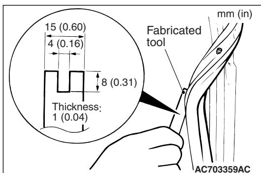
**INSTALLATION SERVICE POINTS****>>A<< DOOR TAPE INSTALLATION**
