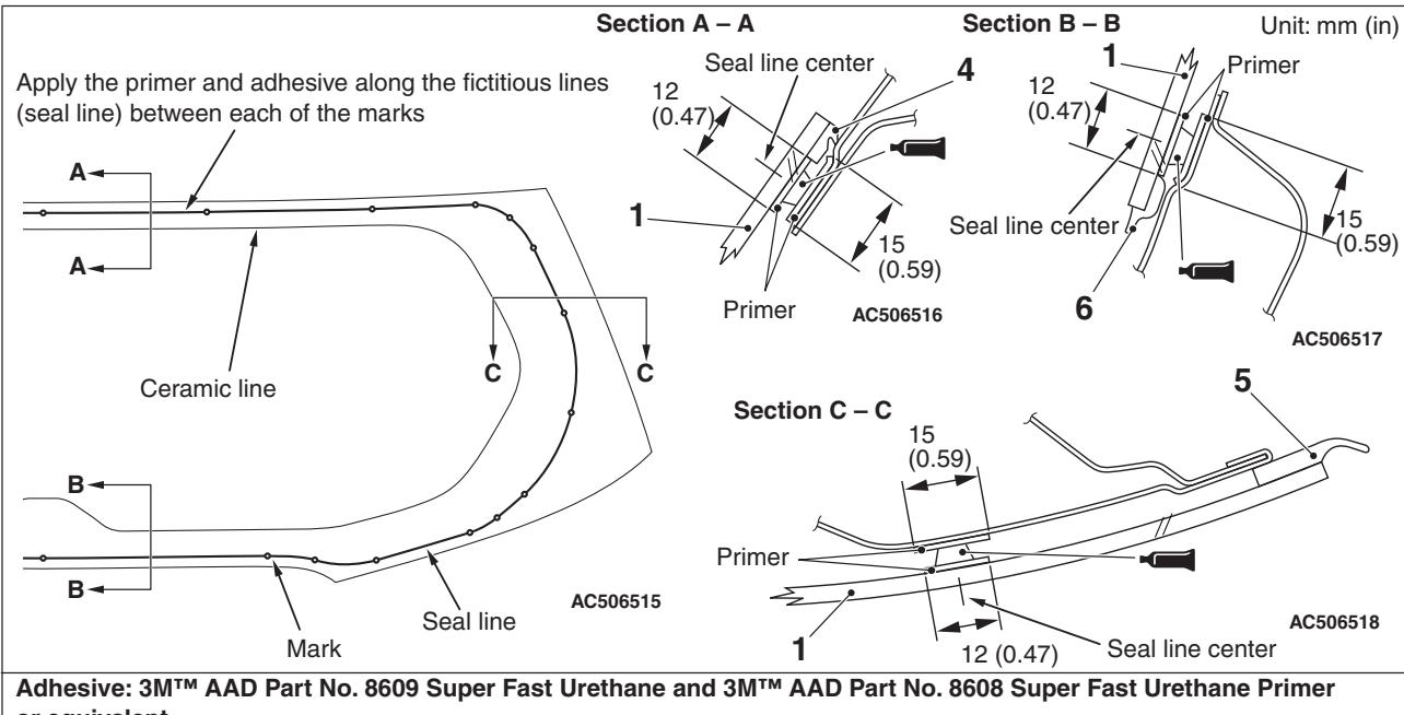
Adhesive: 3M™ AAD Part No. 8609 Super Fast Urethane and 3M™ AAD Part No. 8608 Super Fast Urethane Primer or equivalent
