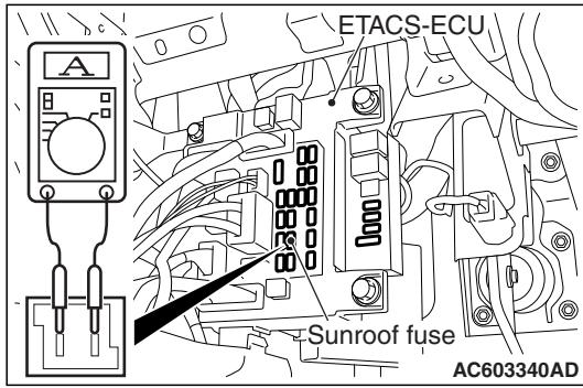
1. Remove the fuse of the sunroof to check that it is normal, then connect the circuit tester as shown in the Figure.
