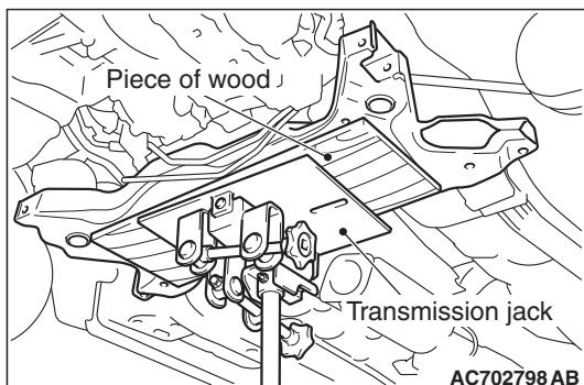
1. Jack up and support the front axle crossmember assembly, and remove it.
