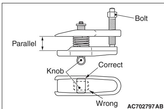
2. Turn the bolt and knob to make the special tool jaws parallel, then hand-tighten the bolt. After tightening, check that the jaws are still parallel.
