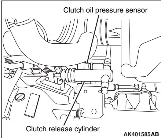
The clutch oil pressure sensor is a sensor detecting the variation of the hydraulic pressure in the clutch release cylinder according to the clutch pedal depressed.
