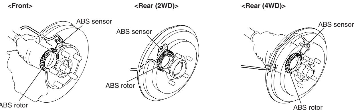
The ABS sensors consist of fixed ABS sensors and the ABS rotors that rotate at the same speed as the wheels, and output alternating current signals at frequencies which are proportional to the wheel speed.
