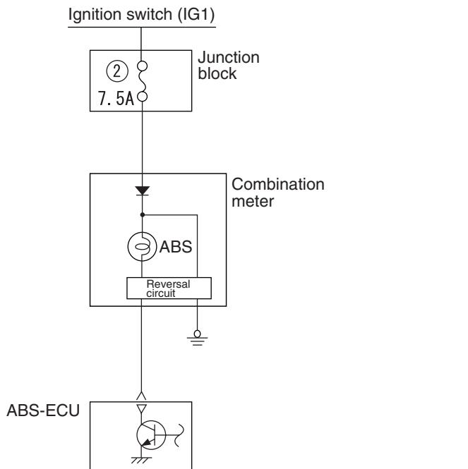
The ABS warning lamp is controlled by the ABS-ECU. The warning lamp drive circuit in the combination meter contains an reversal circuit, which turns the ABS warning lamp off when the transistor in the ABS-ECU is ON and turns the lamp on when the transistor is OFF. The ABS warning lamp illuminates in the following cases:
